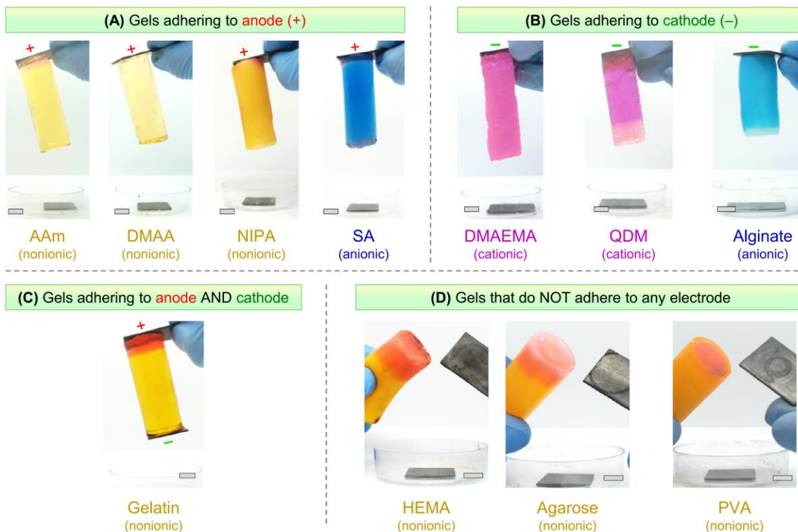
Figure 3.4. Adhesion results for graphite to various gels by EA [HS] . The results are shown through photos. Gels are imbued with dyes and are thus color-coded as follows: non-ionic gels in yellow, anionic gels in blue and cationic gels in pink. Strips of graphite are placed on either end of a cylindrical gel and 5-10 V DC is applied for 15 min. (A) Gels that adhere only to the anode (+); (B) Gels that adhere only to the cathode (-); (C) Gelatin is the only gel that adheres to both electrodes; (D) Gels that do not adhere to either electrode. Scale bars are 1 cm.
