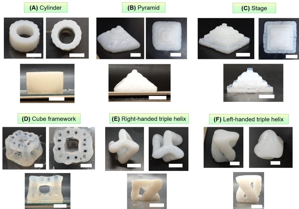
Figure 4.5. Various 3D Structures Printed by Electro-Gelation. (A) Cylinder. (B) Pyramid. (C) Stages. (D) Cube framework. (E) Right-handed triple helix with three-armed-star top & bottom. (F) Left-handed triple helix with triangular top & bottom. Scale bars are 1 cm.
