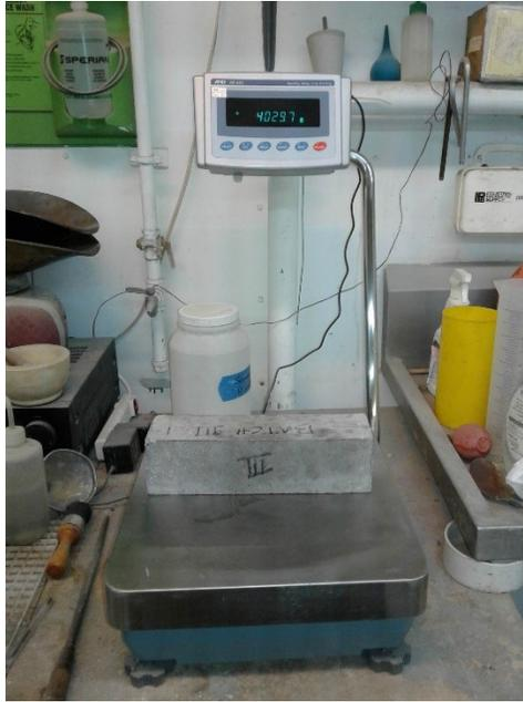
Figure 6-2: Concrete Specimen Positioned for Weight Measurement on a Digital Scale
