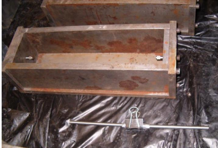
Figure 5-12: Steel Gage Studs in Steel Prism Mold and 10in. Rod Spacer
