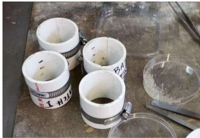
Figure 5-10: Overview of 2in. x 2in. Cylinder Molds
