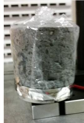
Figure 5-14: 2in. x 2in. Concrete Cylinder Wrapped in Teflon Film Ready for Scanning
