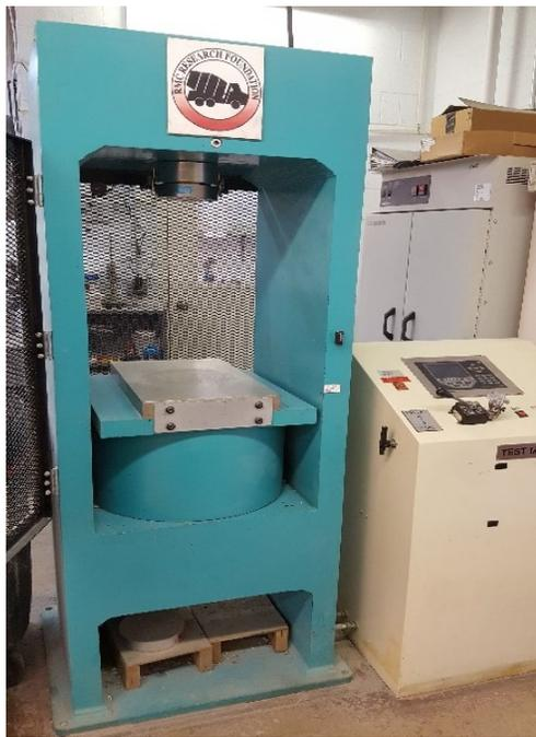
Figure 6-4: Compression Testing of a Concrete Cylinder
