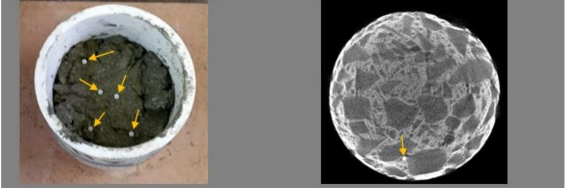
Figure 5-8: Placement of Polystyrene Microsphere (yellow arrows) During Casting
