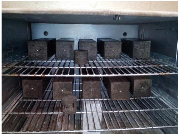
Figure 5-5: Specimens in Oven During Duggan Heat Treatment
