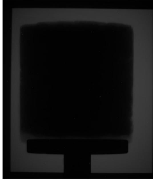
Figure 8-2: Neutron Radiograph of a Concrete Specimen
