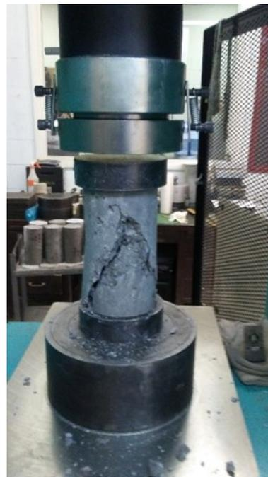
Figure 6-3: Compressive Test Machine Used
