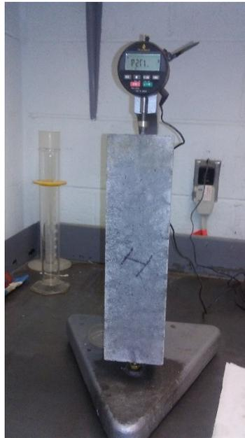
Figure 6-1: Comparator Set Up for Expansion Measurement
