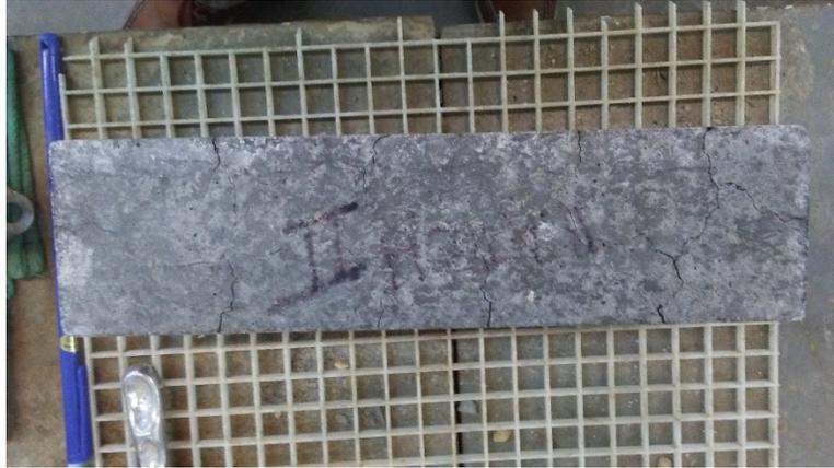
Figure 9-5: Appearance of Hairline Crack at the Surface of Heat-Treated Concrete Specimen with High Potassium at Age 357 days
