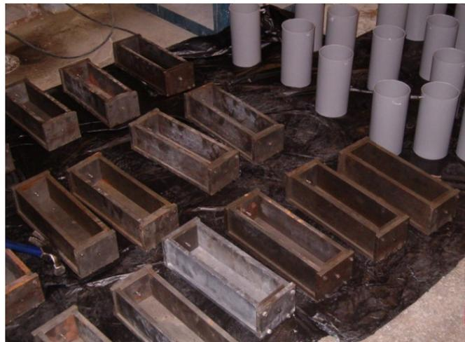
Figure 5-11: Steel Prism Molds and 4in. x 8in. PVC Cylinder Molds
