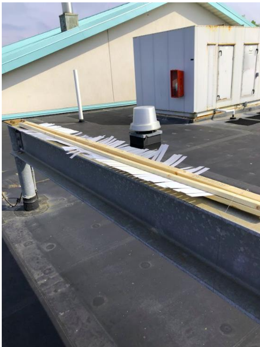
Figure A1. Control board deployed on top of building with six types of plastic: PP, PVC, LDPE, HDPE, PS, and PET.
