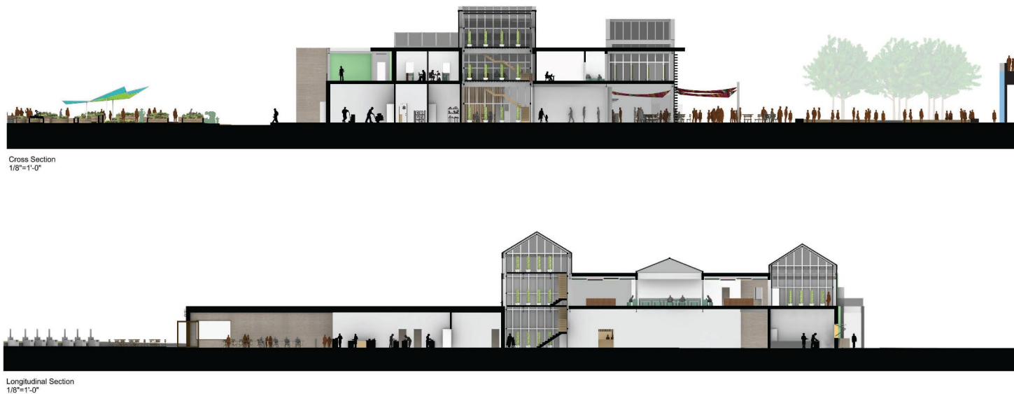
Figure 52 New Building Sections (developed by author)
