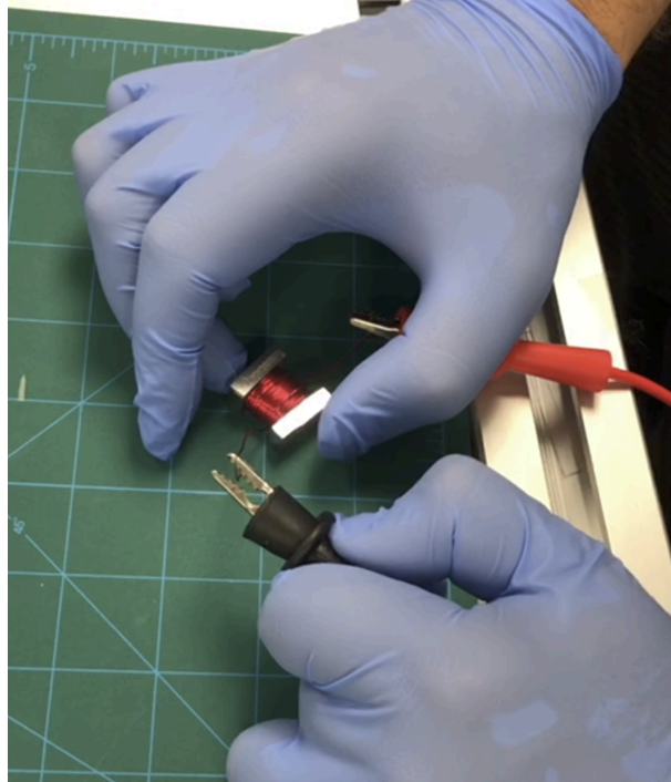
Figure 23. Testing of EPM magnetic field output at different currents and pulse lengths.
