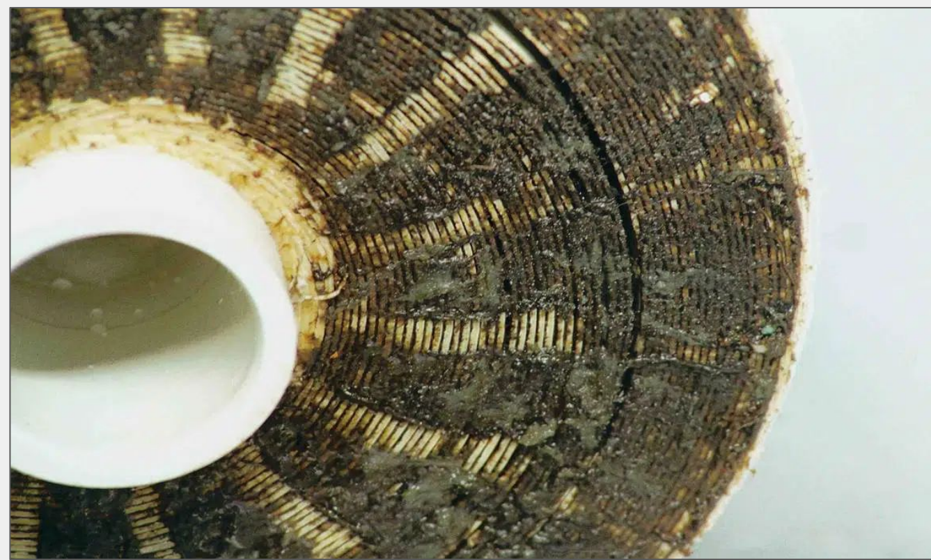
Figure 1: Fouled R.O. Membrane
