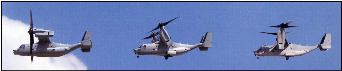
Figure 1.1. V-22 Osprey in airplane, conversion and helicopter modes (from Ref. 1).
