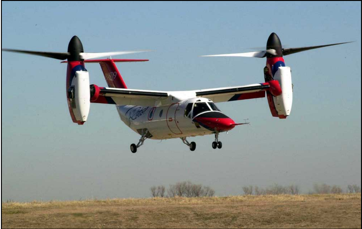
Figure 1.5. First flight of the BA-609 commercial tiltrotor (from Ref. 11).
