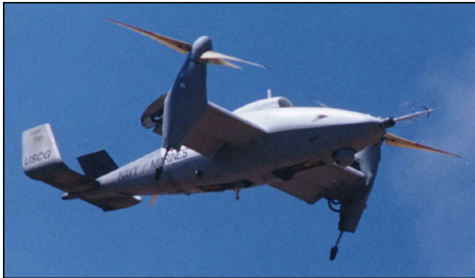
Figure 1.4. Bell Helicopter's 7/8-scale Eagle Eye UAV (from Ref. 10).
