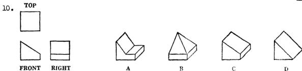
In question No. 10, object C looks like the view marked "TOP" when looked at from directly above, and like the views marked "FRONT" and "RIGHT" when looked at from the front and right side respectively. Therefore, the space under C has been blackened for question No. 10 on the Sample Answer Sheet.
