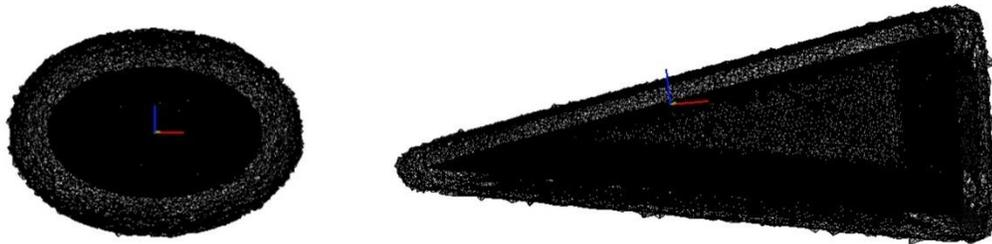
**Figure 3.2:** Trimmed no slip boundary condition of the ellipsoid (left) and ramp (right) with a trim distance of .0015 m and .005 m, respectively.
