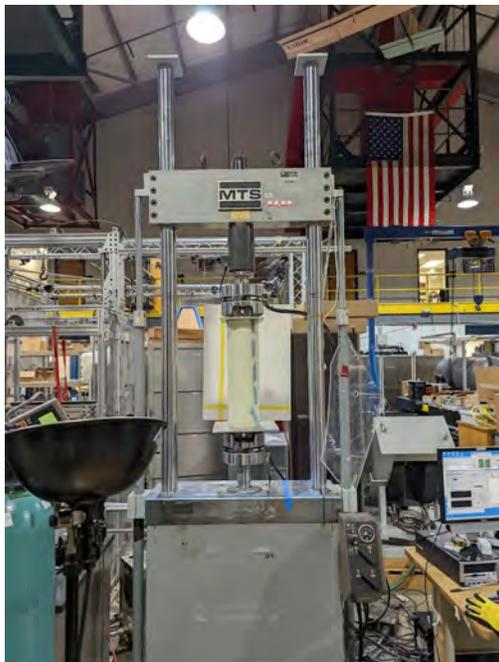
**Fig. 13 Fiberglass tube in testing jig**
