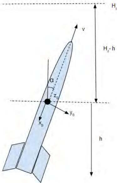
Fig. 58 The relevant states ( $h$ ,  $v$  and tilt off the vertical-axis  $\alpha$ ) of the closed-loop altitude control system and body axis
