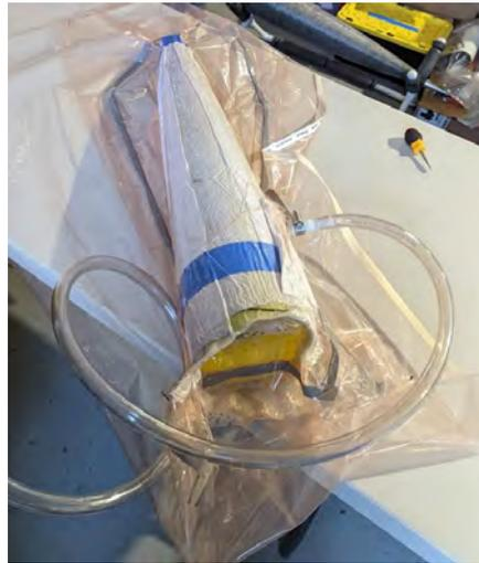
**Fig. 21** Fiberglass layup using a PLA mold and vacuum bagging
