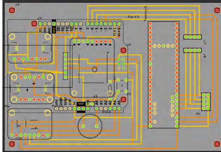
Fig. 57 *Terpulence II* air brake PCB diagram
