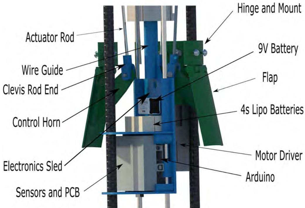
**Fig. 52 Middle section of the air brake**
