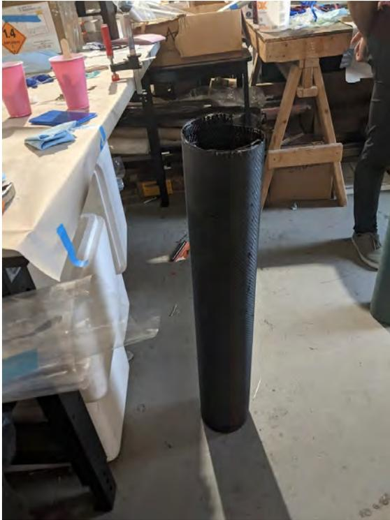
**Fig. 8 Airframe after removal from the mandrel**
