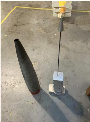
**Fig. 72 Mounting system. Left: Nose cone shell. Right: Payload frame and bulkhead on support blocks**
