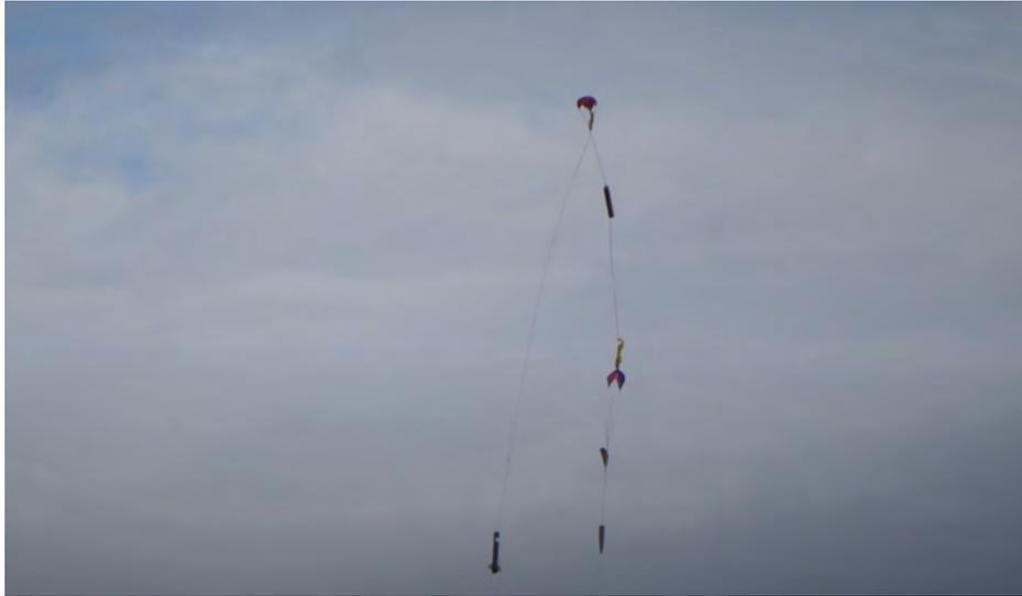
**Terpulence II's main parachute wrapped around the kevlar harness**
