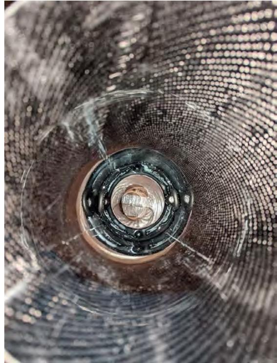
**Fig. 34** The motor mount after being epoxied into the airframe.
