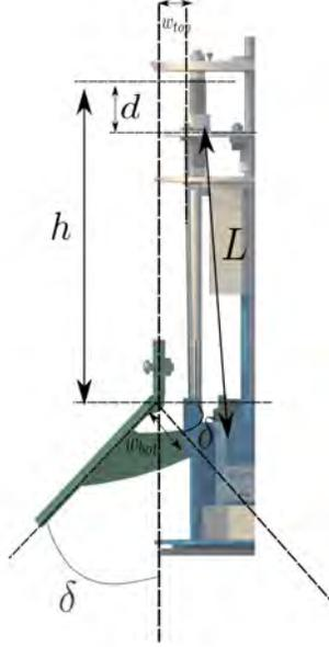
**Fig. 47 Geometry Of deployment mechanism**
