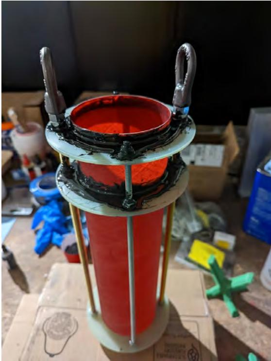
**Fig. 33** A view of the motor mount before installation into the airframe
