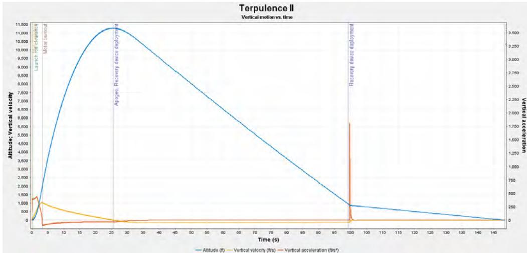
**Fig. 4 OpenRocket simulation for Spaceport America conditions**
