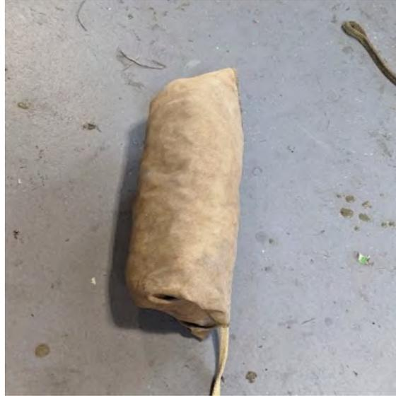
**Fig. 30** The main parachute tightly wrapped in the nomex blanket and ready for launch
