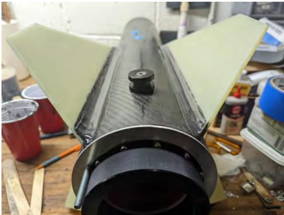
**Fig. 19** A set of external fillets curing
