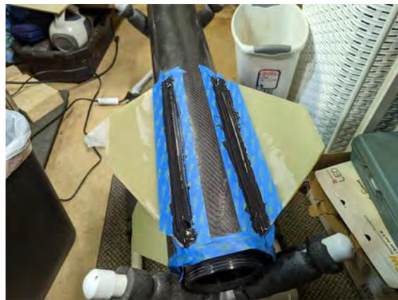
**Fig. 79** Reapplied external fillets curing
