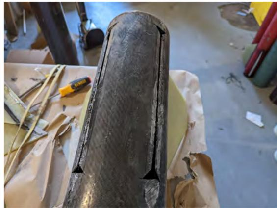
**Fig. 77** Airframe with expanded fin slots cut out
