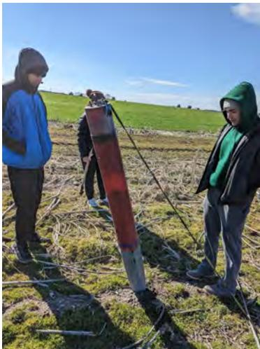
**Fig. 74 Top half of our rocket after the main parachute failed to deploy**
