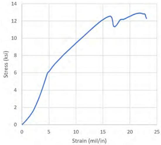
**Fig. 12 Stress - Strain for fiberglass tube**
