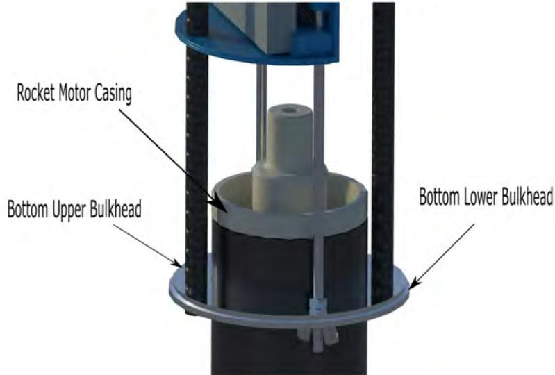
**Fig. 54 Lower section of the air brake**
