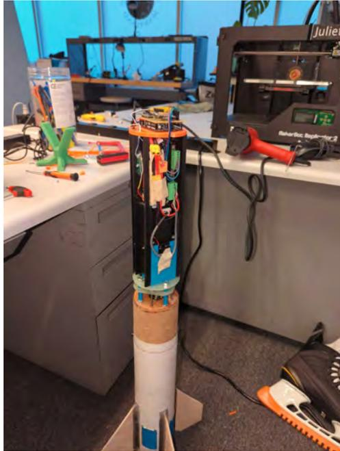
**4in air brake test rocket assembly**
