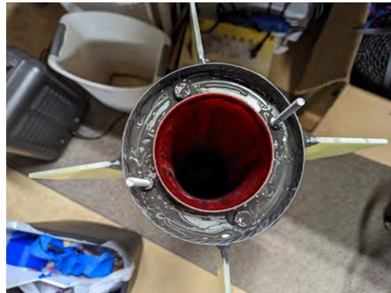
**Fig. 20** The aft centering ring epoxied into the airframe
