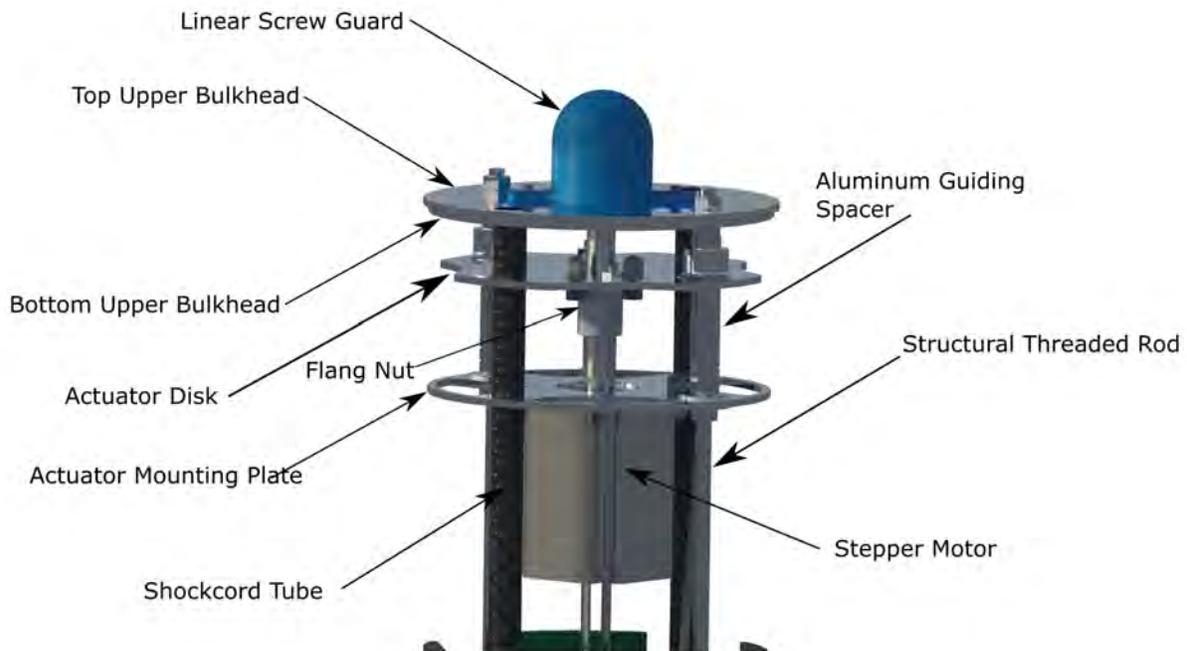
**Fig. 49 Upper section of the air brake**
