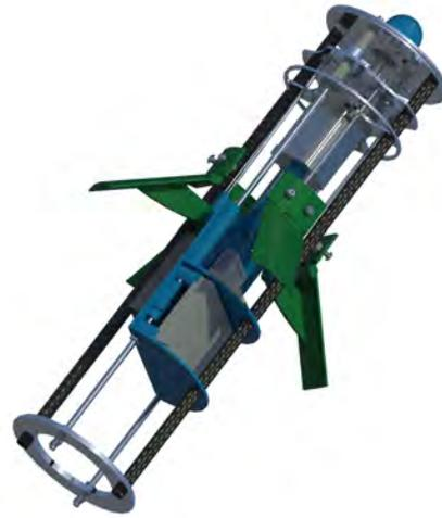
**Fig. 42 Internal CAD of the air brake module.**
