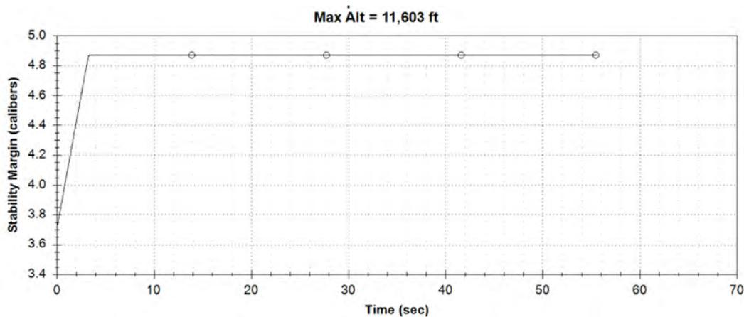
**Fig. 6 Stability margin simulation from RasAero II**
