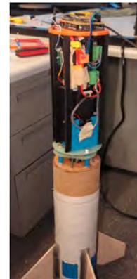
**Fig. 62 4in air brake test rocket**
