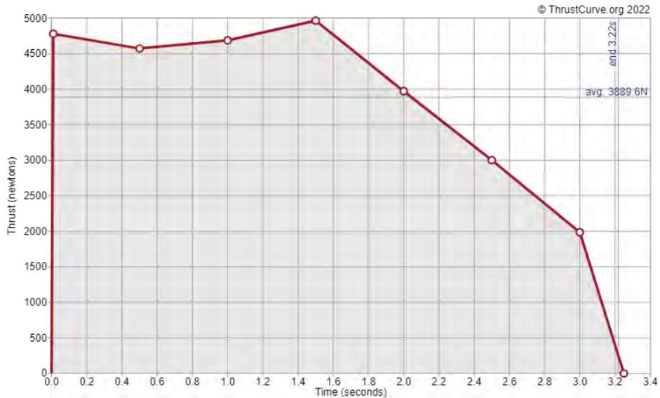
**Fig. 3 Loki N3800 motor characteristics [7]**
