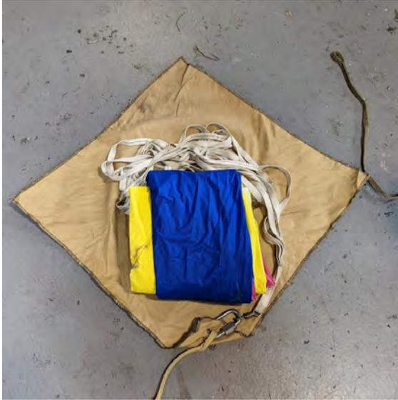
**Fig. 29** The main parachute folded and shroud lines loosely folded over the nomex blanket.
