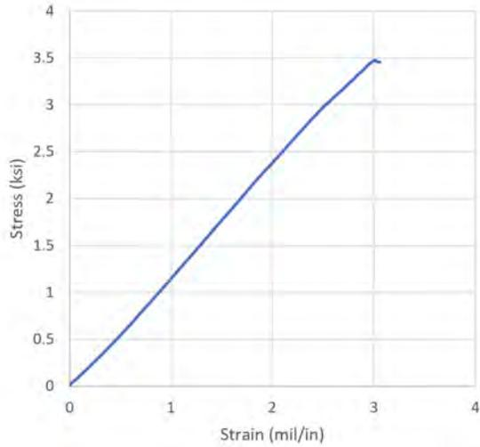
**Fig. 11 Stress - Strain for carbon fiber tube**
