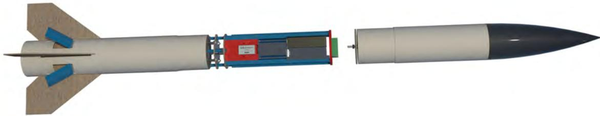
**Fig. 61 CAD of 4in air brake test rocket**
