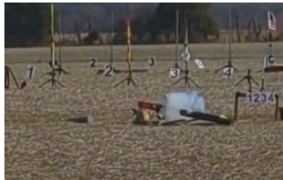
**Fig. 37** Drogue deployment test
