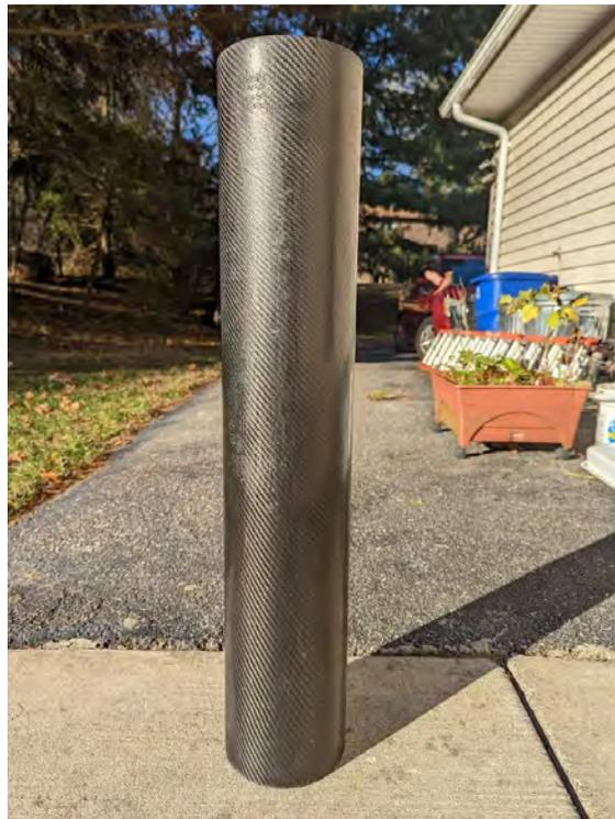
**Fig. 9 Airframe with light coats of epoxy**
