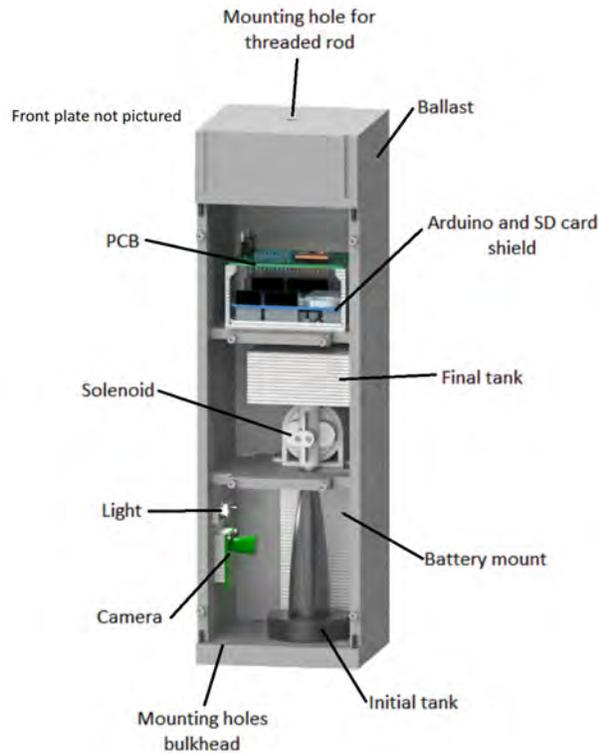
**Fig. 70 Payload CAD**
