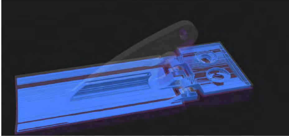
**Fig. 53 Carbon fiber placement on the flap**
