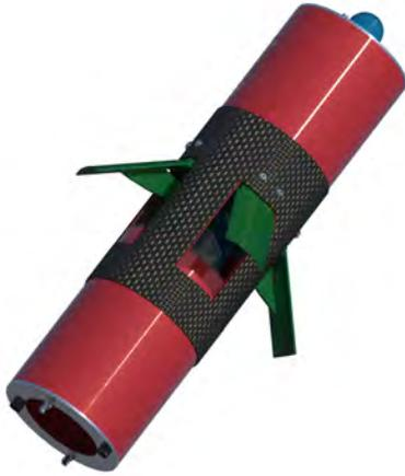
**Fig. 41 External CAD of the air brake module.**
