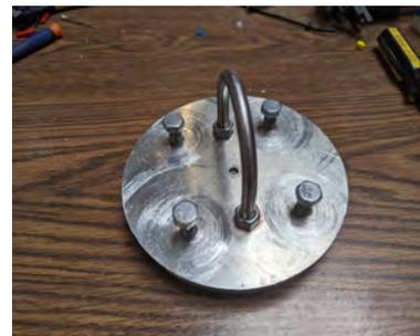
**Fig. 32** Nose cone bulkhead
