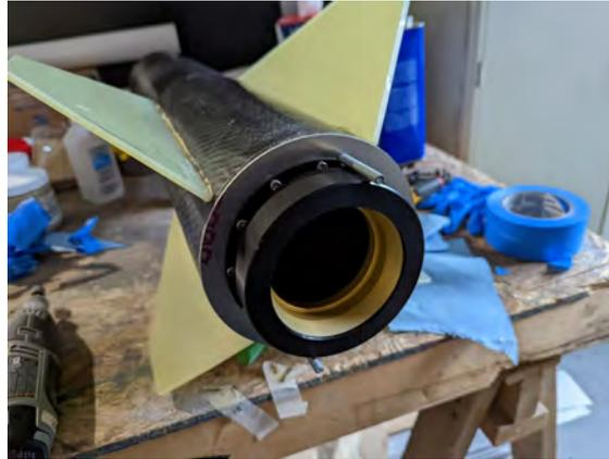
**Fig. 28 Thrust plate integrated with rocket**
