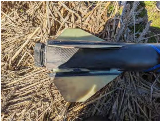
**Fig. 76** Damage to two of the fins after Impact
