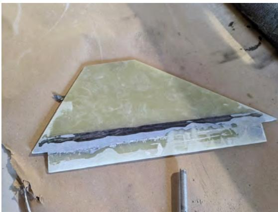
**Fig. 78** Fins after sanding down remaining epoxy
