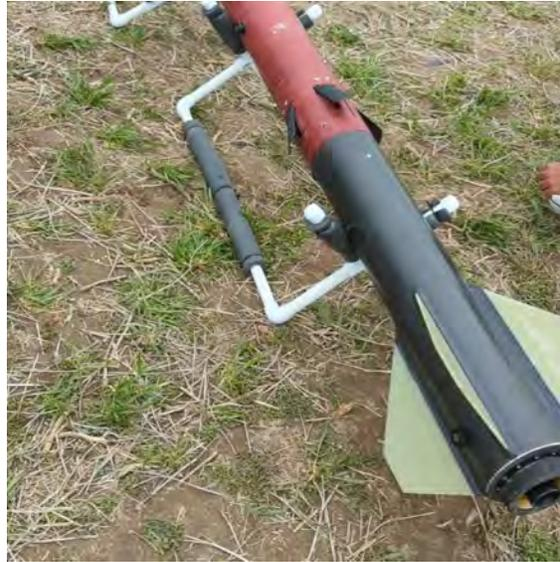
**Fig. 40 Air brake module installed in Terpulence II**
