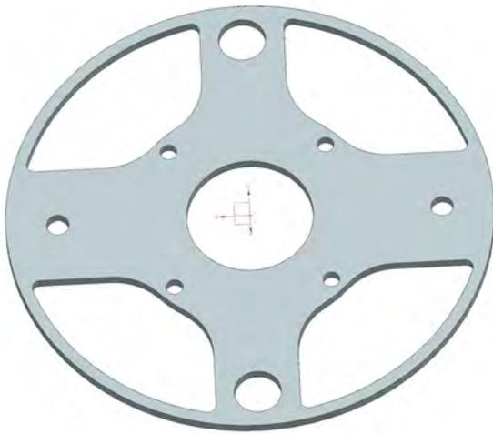
**Fig. 50 Actuator mounting plate CAD**
