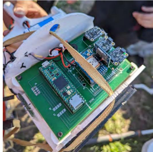
**Fig. 56 Air brake sled and electronics**
