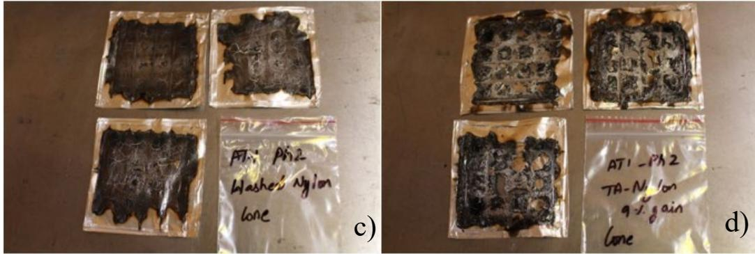
Figure 4.1: Cone Calorimeter Charred Remains for Control Cotton (a), PA Cotton (b), Control Nylon (c), and TA Nylon (d) samples [48]
