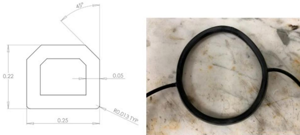
Figure 2.4: Schematic Cross Section of the Seal (Left), Top-Down View of the Seal (Right)
