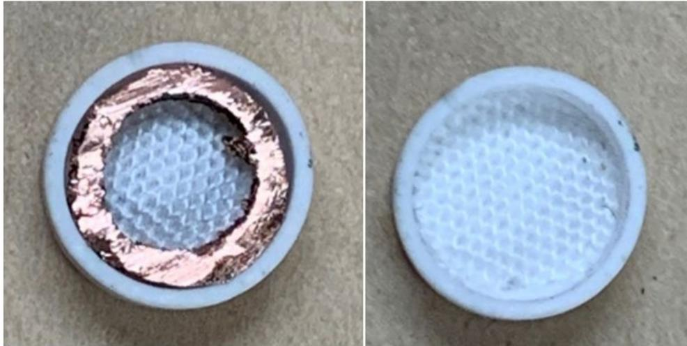
Figure 3.4: 4 Layers of Cotton packed into the crucible with the Ring Method (Left) and the Tamper Method (Right)
