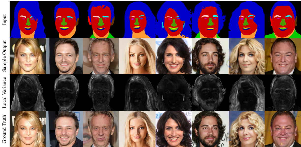
Figure 5.11: Examples of local stochastic variations. Top to bottom rows represent the input image, one sample output, the standard deviation of each pixel over 20 different outputs of the same input, and the ground truth image respectively.
