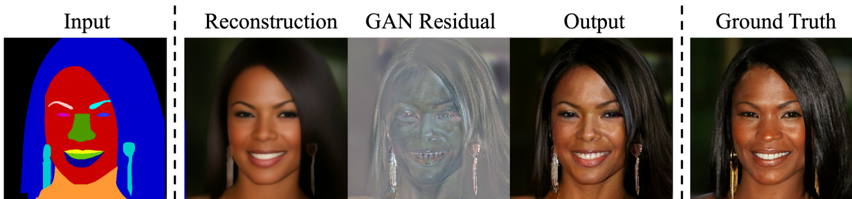
Figure 5.1: We decouple the optimization of reconstruction and adversarial losses by synthesizing an image as a combination of its reconstruction (low-frequency) and GAN residual (high-frequency) components. The GAN residual adds realistic fine details while avoiding the pixel-wise penalty imposed by reconstruction losses.
