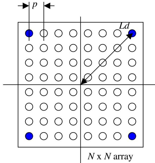
**Figure 37: A schematic top view of a  $N \times N$  array interconnect**
