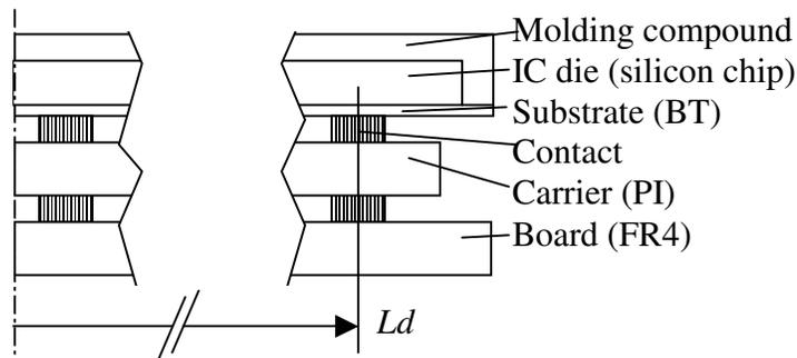
**Figure 38: A schematic cross-section view along the center and one corner contact**
