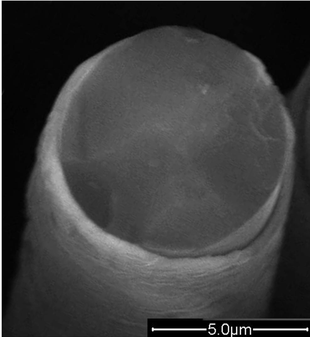
**Figure 6: Cross section of nickel-coated carbon fibers**
