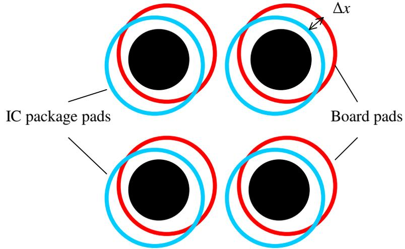
**Figure 39: Pads offset due to CTE mismatch does not affect the contact integrity in this case**
