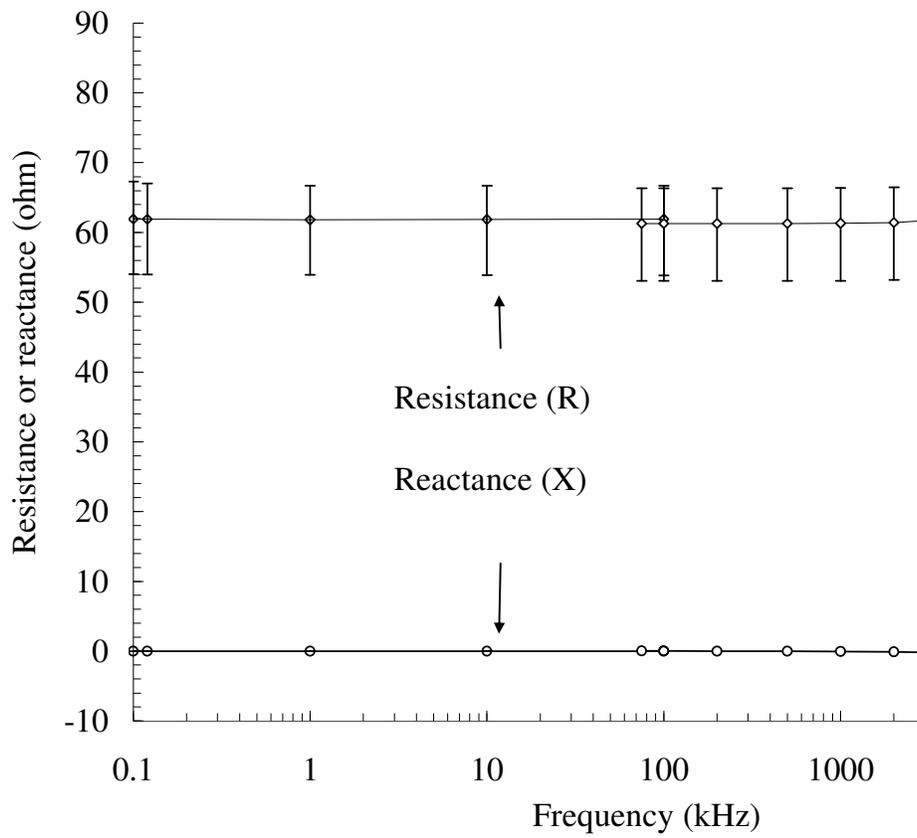
**Figure 11: Resistance and reactance of individual nickel-coated carbon fiber**
