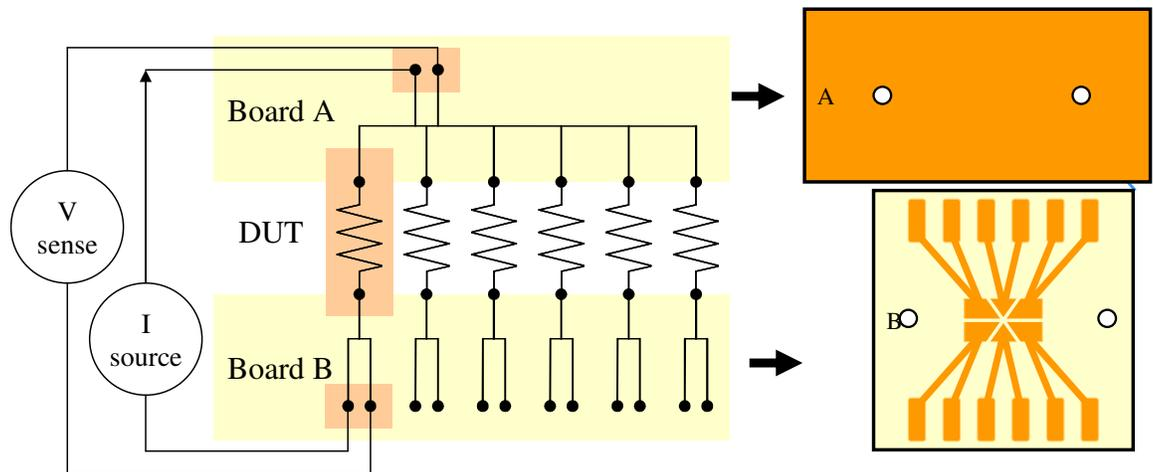
**Figure 41: Diagram of the test circuit**
