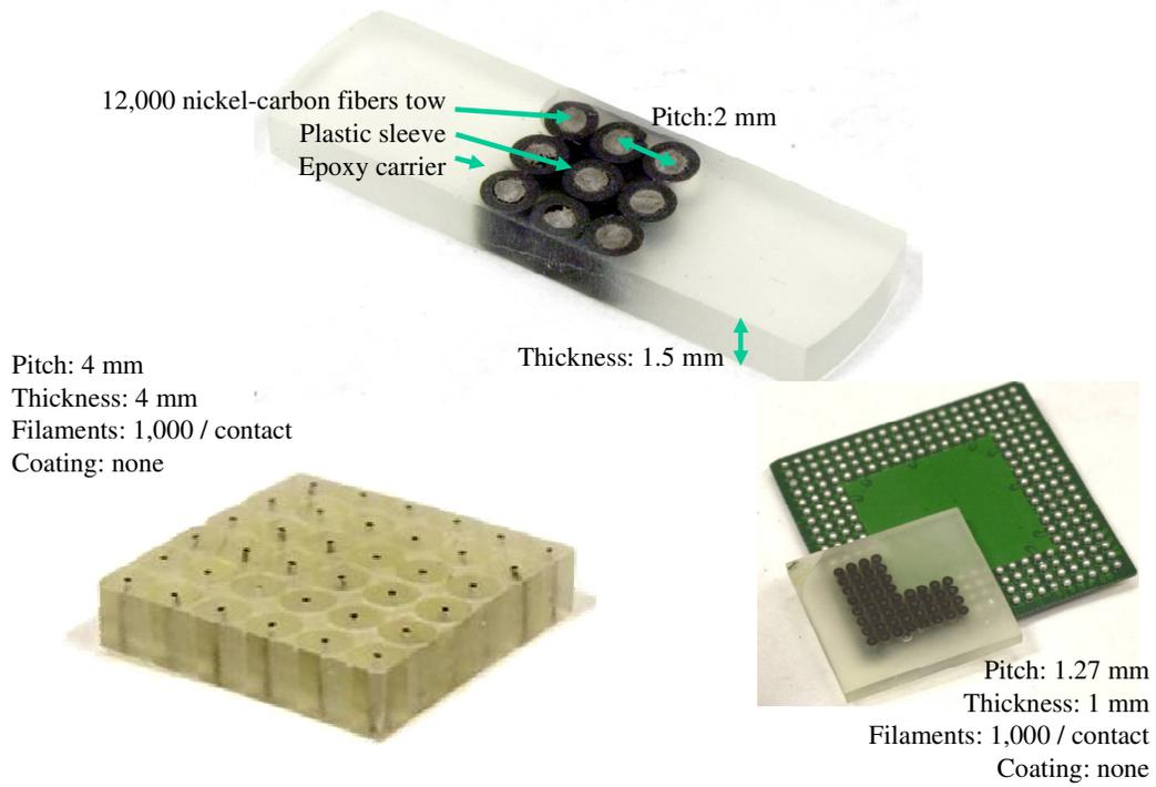
**(c) IC package to board interconnect prototypes**
