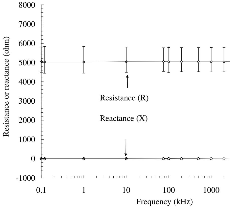
**Figure 10: Resistance and reactance of individual plain carbon fiber**
