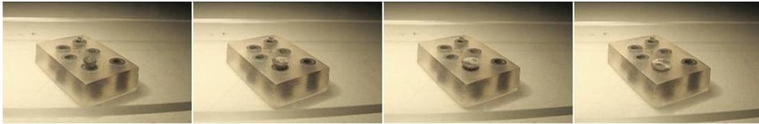
**Figure 21: A carbon fiber brush being compressed by a piece of glass**
