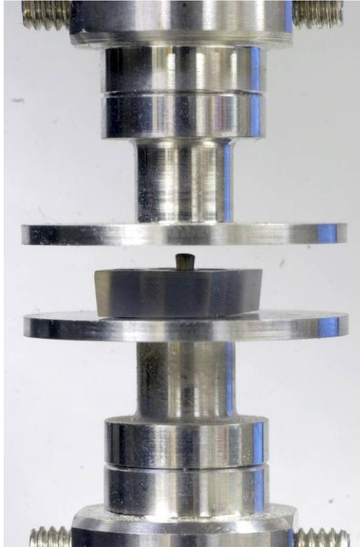
**Figure 27: Test probe and contact under test**
