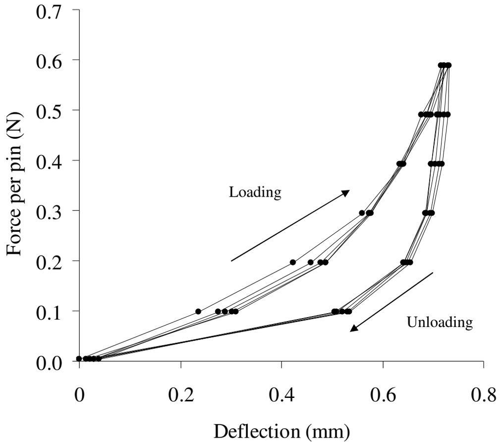
**Figure 34: Force-deflection result of first 5 cycles**
