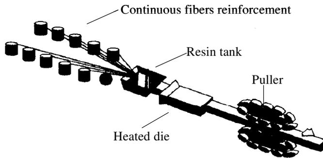
**Figure 4: Pultrusion process of carbon fiber composite [12]**
