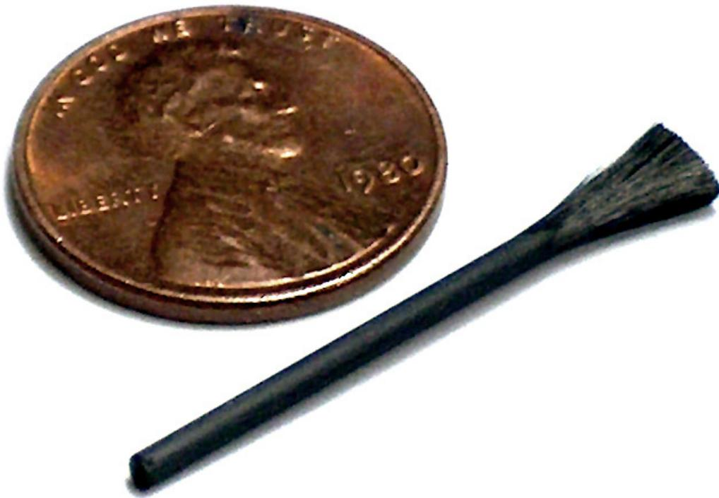
**Figure 20: A carbon fiber composite rod with a brush at the end**
