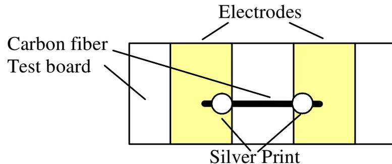
**Figure 9: Schematic of test board for carbon fiber characterization**
