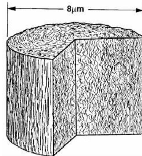
**Figure 2: Illustration of the microstructure of a PAN-based carbon fiber [1]**
