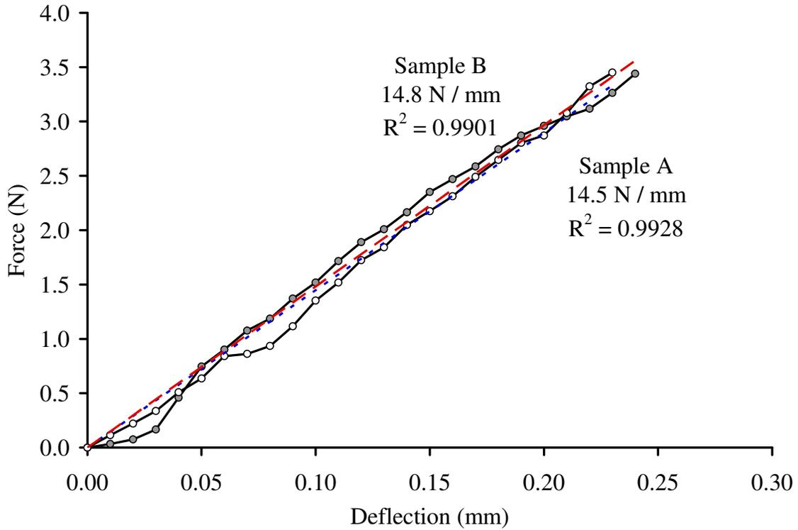
**Figure 29: Force-Deflection Result - Samples A and B**
