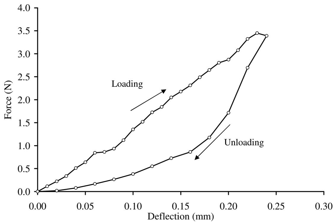
**Figure 30: A cycle consisting of loading and unloading indicates an energy loss**
