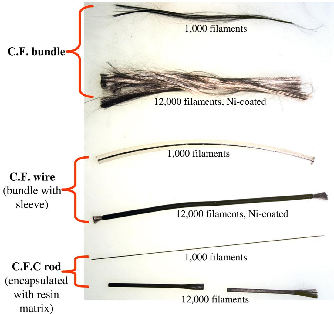
**Figure 3: Carbon fibers in different one-dimensional continuous forms**
