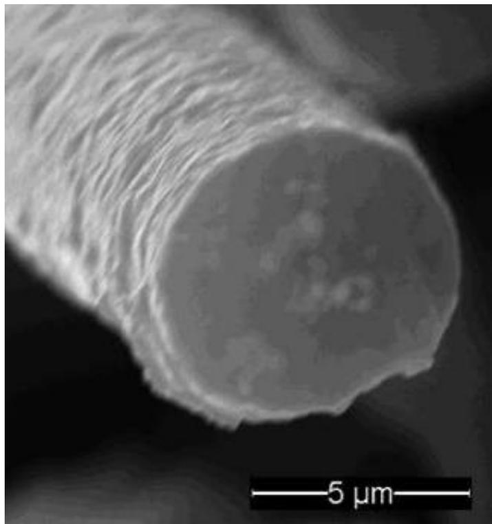
**Figure 1: A carbon fiber under scanning electron microscopy (SEM)**
