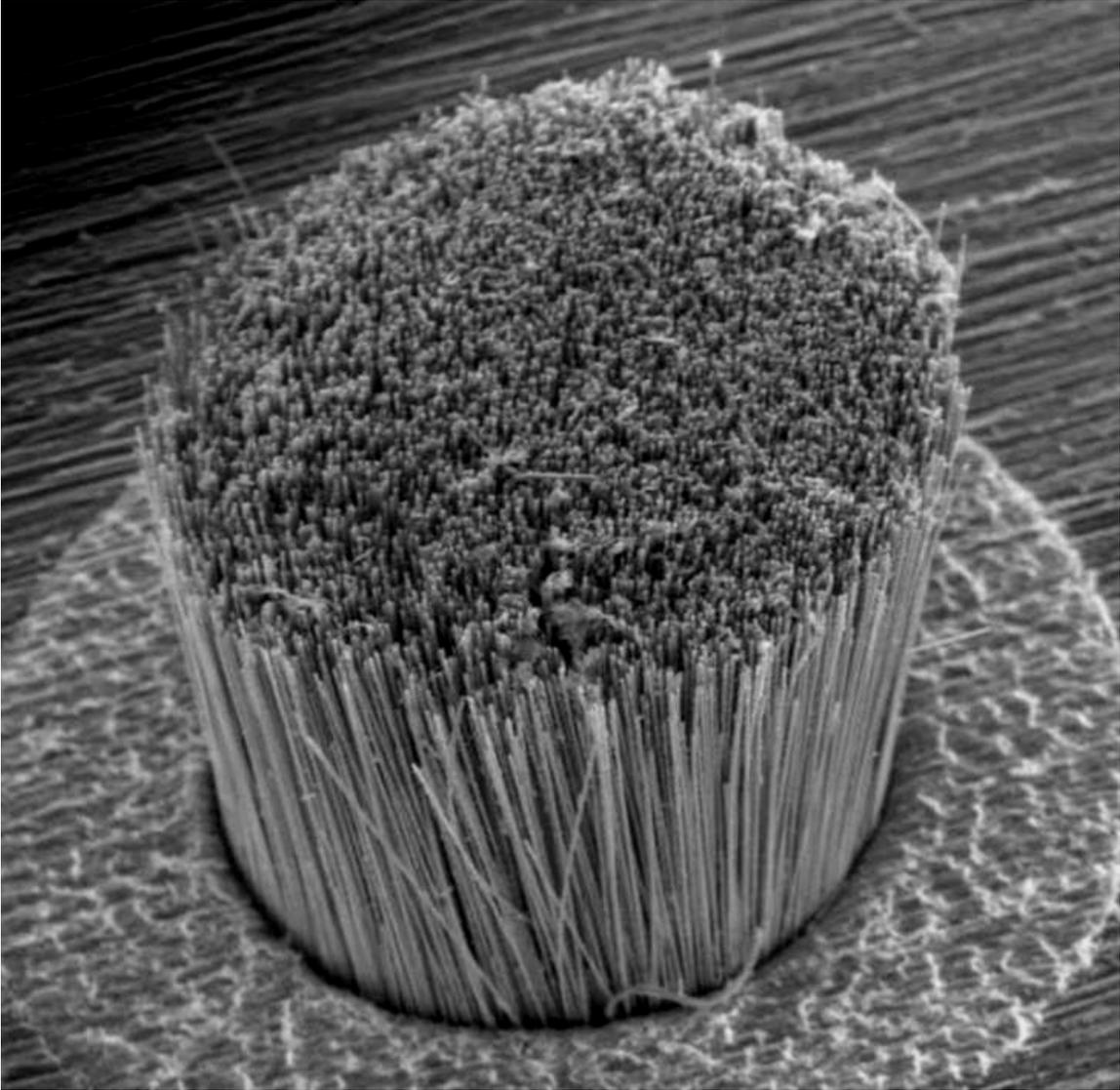
**Figure 36: Microstructure of a contact after the cyclic loading test**
