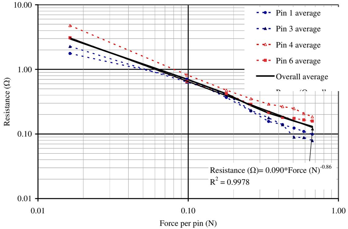
**Figure 43: Resistance-load characterization result (averaged, log-log)**
