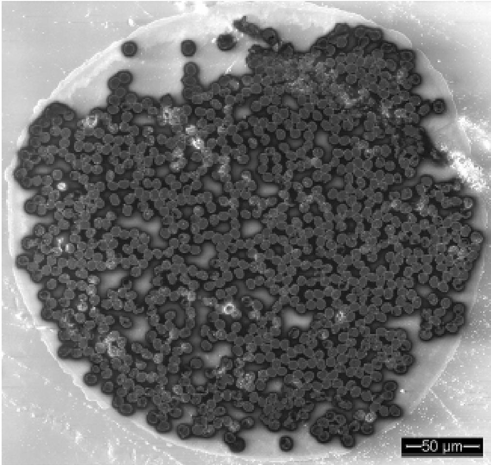
**Figure 5: Cross section of a carbon fiber composite rod (1,000 filaments)**
