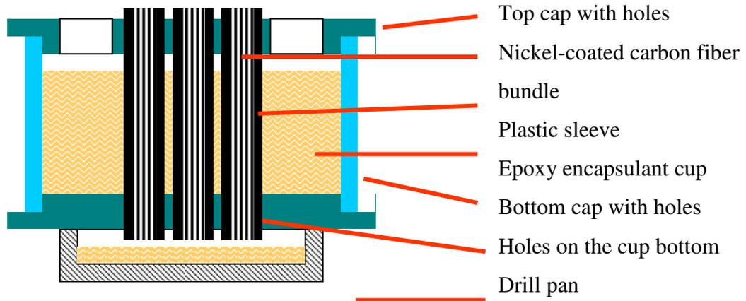
**Figure 25: Cross-section illustration of the mold in encapsulation**
