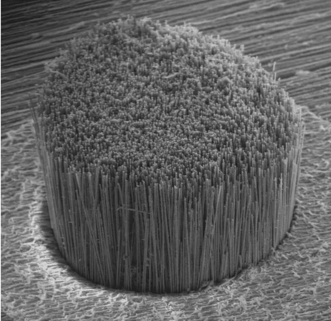
**Figure 35: Microstructure of a contact before the cyclic loading test**
