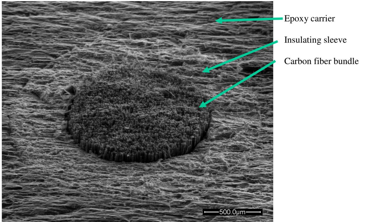
**Figure 26: Surface processed by water-jet cutting**
