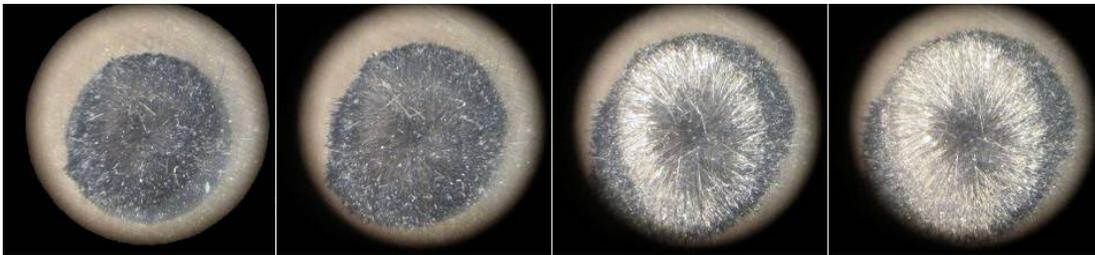
**Figure 22: Close-up of a carbon fiber brush being compressed by a piece of glass**
