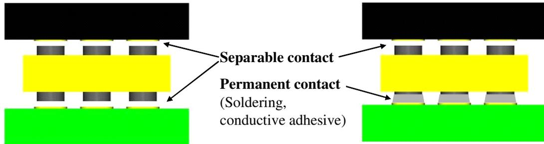
**Figure 8: Permanent and separable contact**
