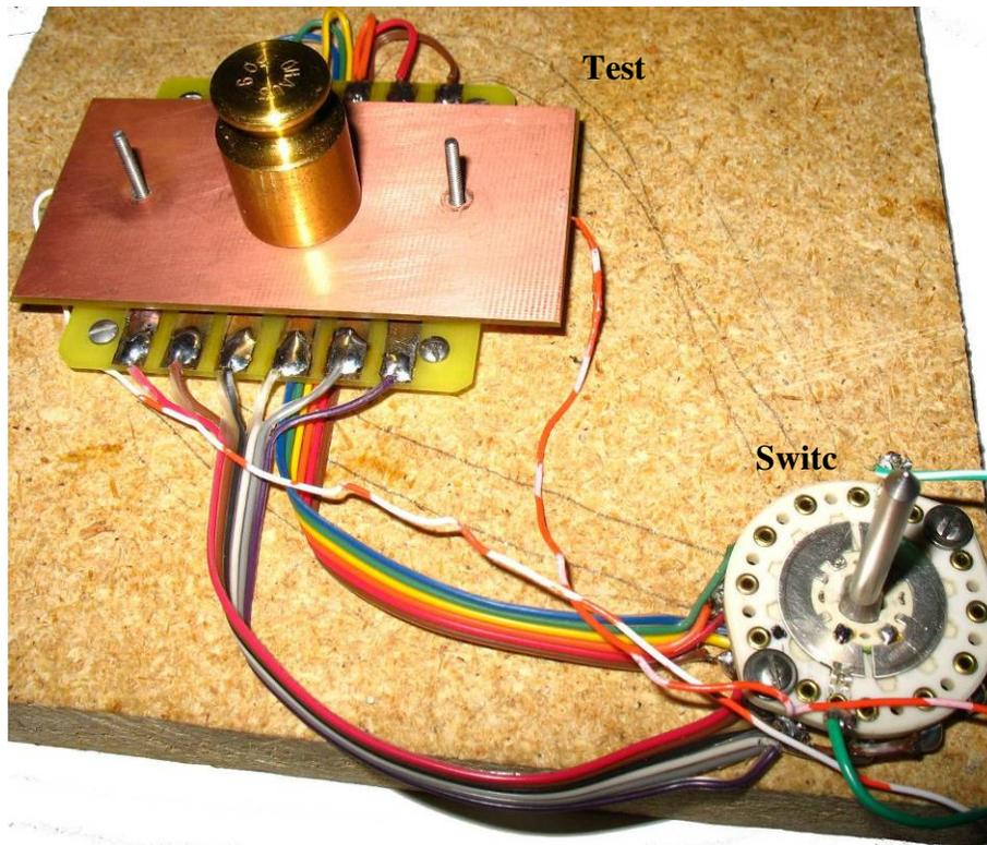
**Figure 40: Test fixture for resistance characterization of the prototype**
