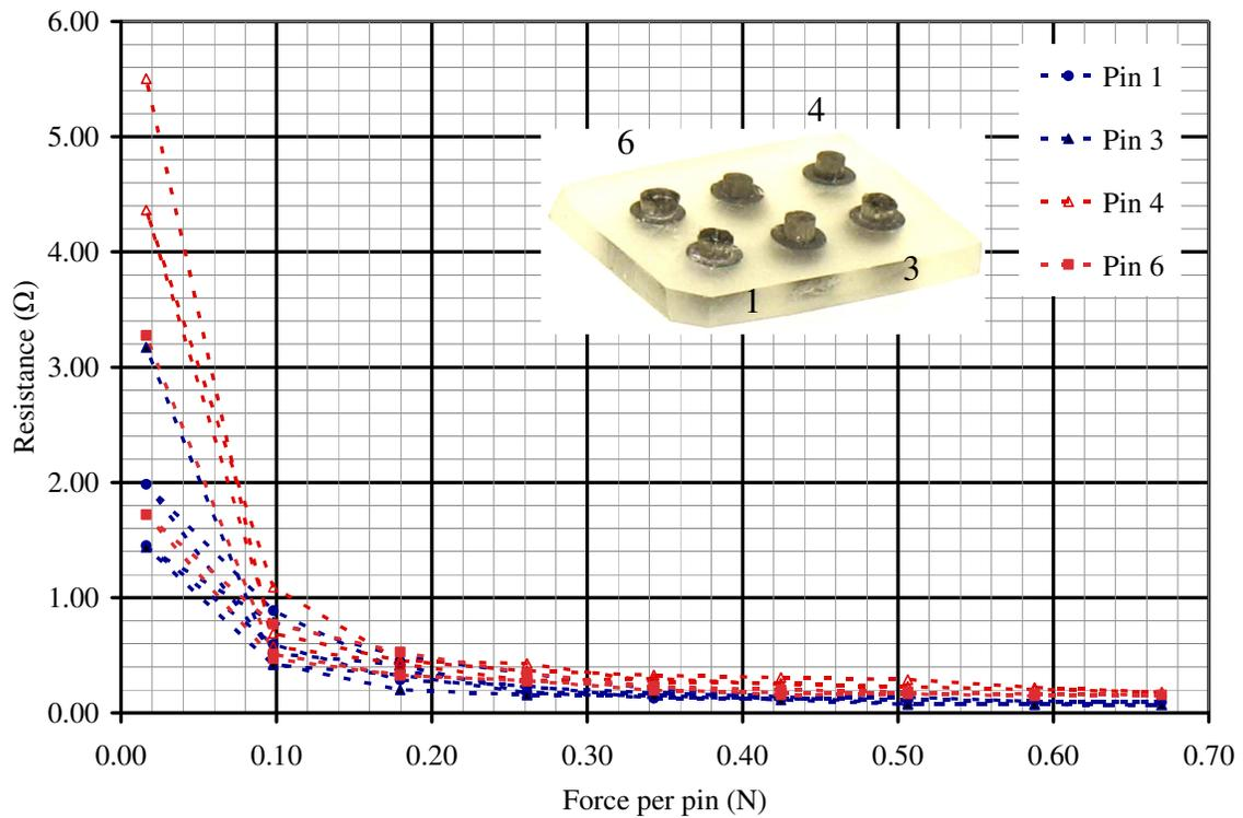
**Figure 42: Resistance-load characterization result (raw)**
