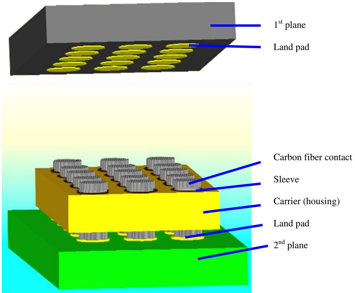
**Figure 7: Carbon fiber grid-array interconnect design**
