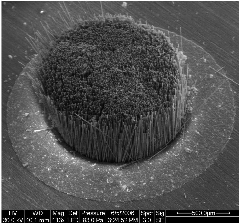
**(b) A contact pin, consists of 12,000 nickel-coated carbon fibers**
