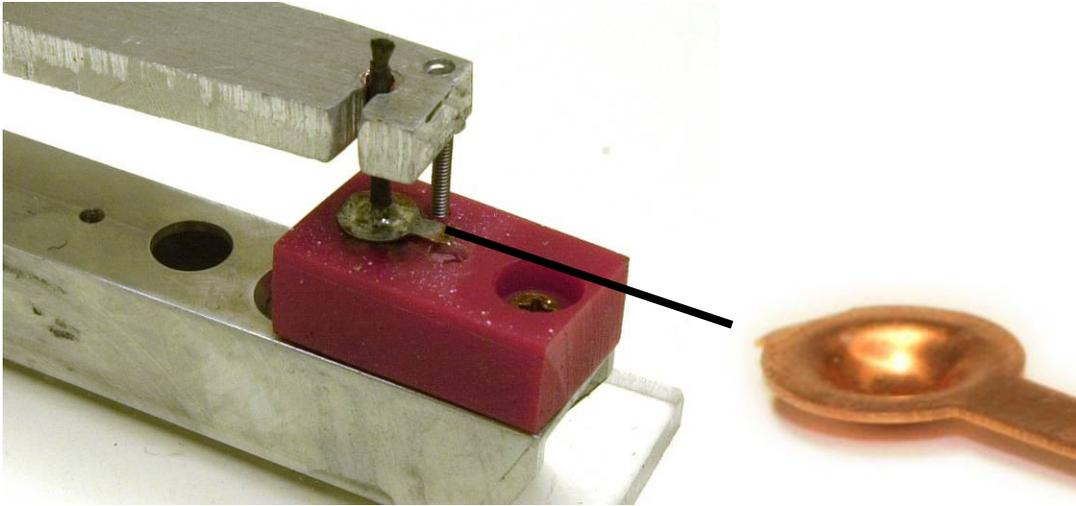
**Figure 14: A fixture holding carbon fiber sample and copper substrate**
