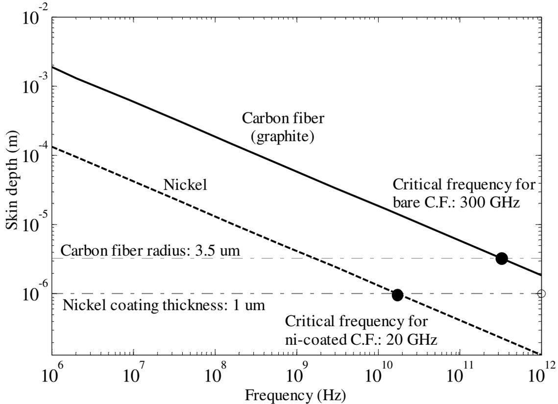
**Figure 13: Skin depth versus frequency for different conductor materials**
