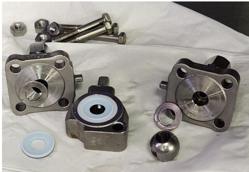
Figure 4.8: Hand Valve Disassembled Post-Test Showing No Signs of Reaction
