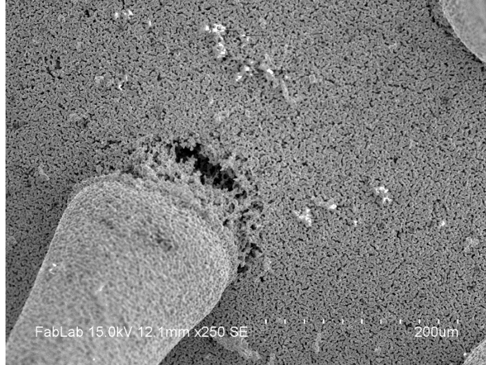
Figure 3.8: SEM images reveal excellent contact between the 3D printed garnet columns and the dense garnet. Accidental knocking over of the column during handling resulted in the extraction of a significant portion of the dense garnet, highlighting the intimate contact achieved.
