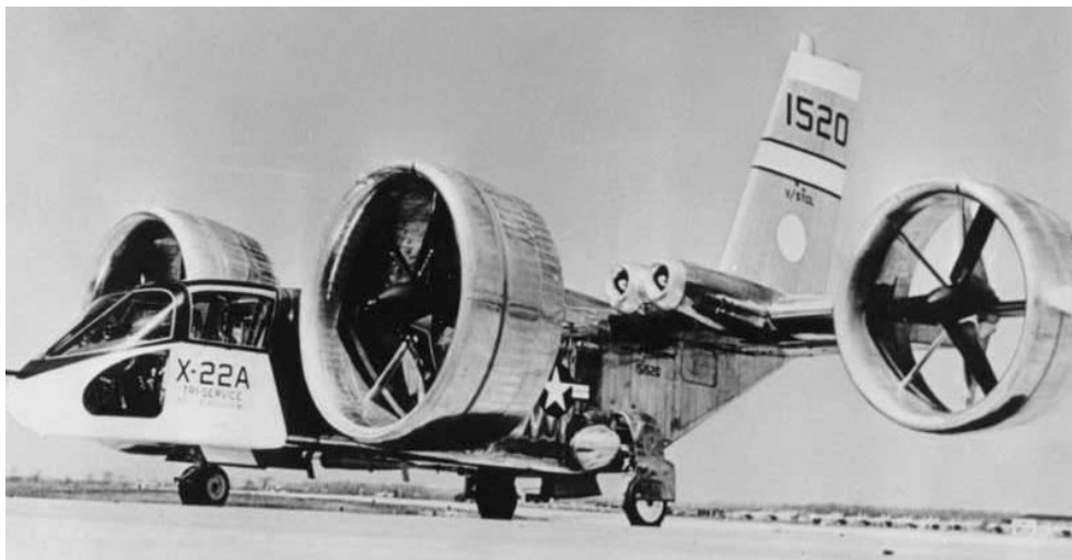
Figure 1.2. Bell X-22 experimental V/STOL troop transport
