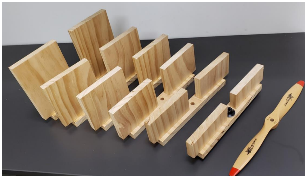
Figure 3.21. High-profile-drag rotors and a wooden propeller
