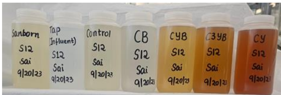
Fig. 4-2. Influent (tap water) and effluent samples collected after simulated rainfall event #12
