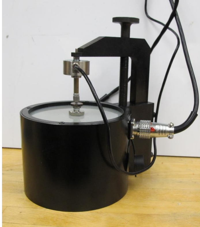
Figure 3 The Berlincourt-type quasistatic d_{33} meter was used to measure the piezoelectric coefficient for all porous samples.
