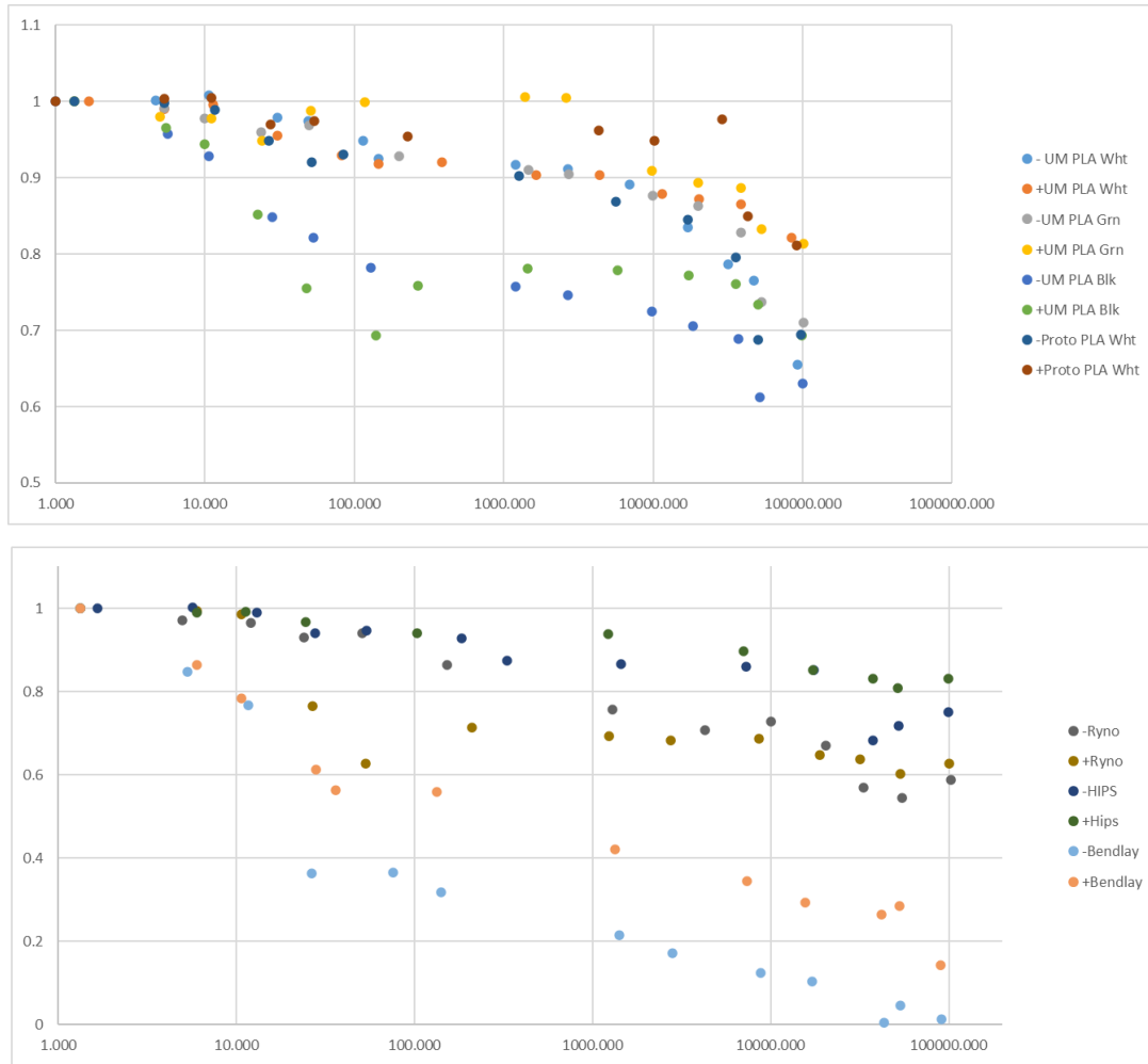
Figure 14 Normalized surface potential decay at ambient temperature, dry box conditions, for all studied filament materials. Separated into two plots for clarity.
