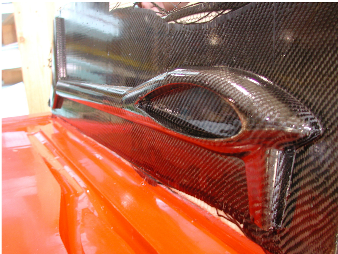
Figure 5.20. Boom Mold and Part – PVA release rinsed off with water.
