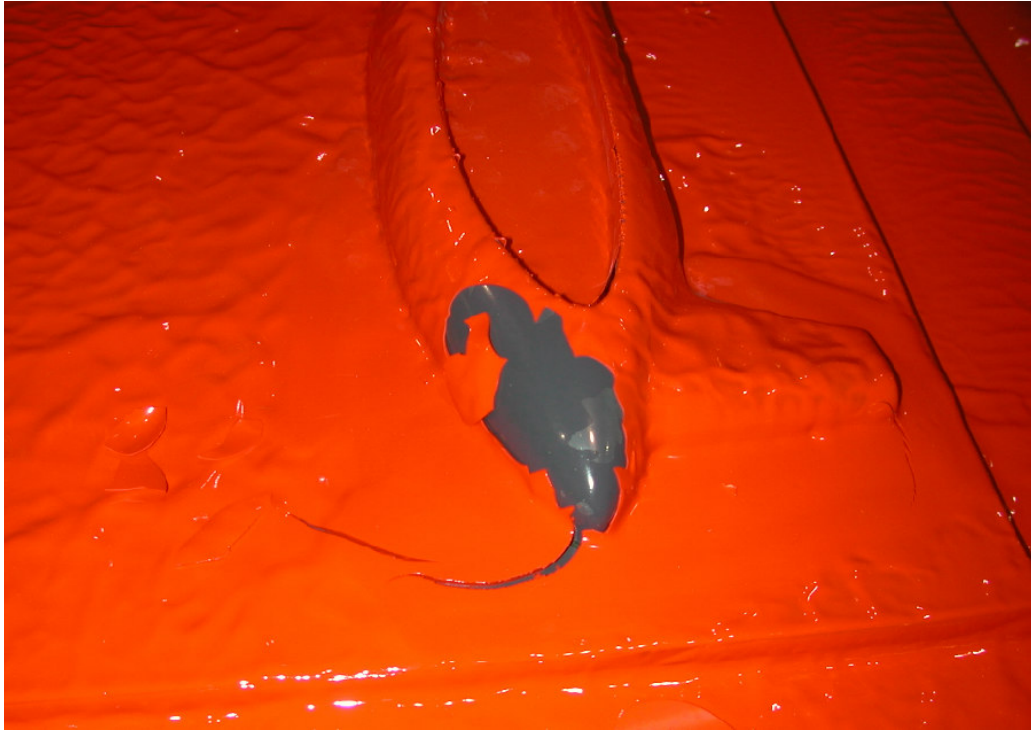
Figure 4.7. Cracked Gel Coat due to Uneven Thickness.
