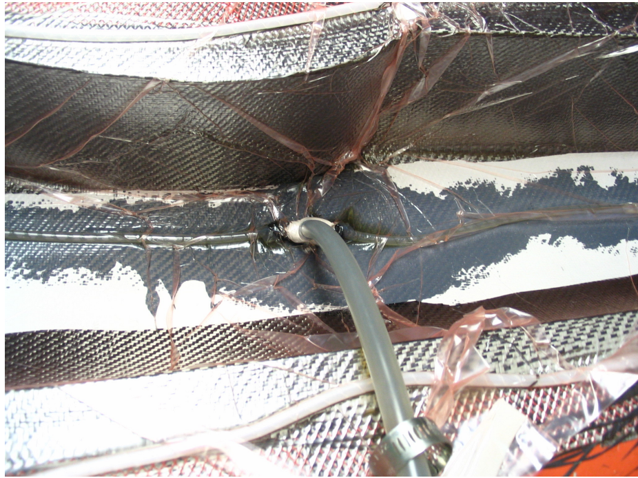
Figure 5.16. Resin Infusion in Progress – right fuselage half.
