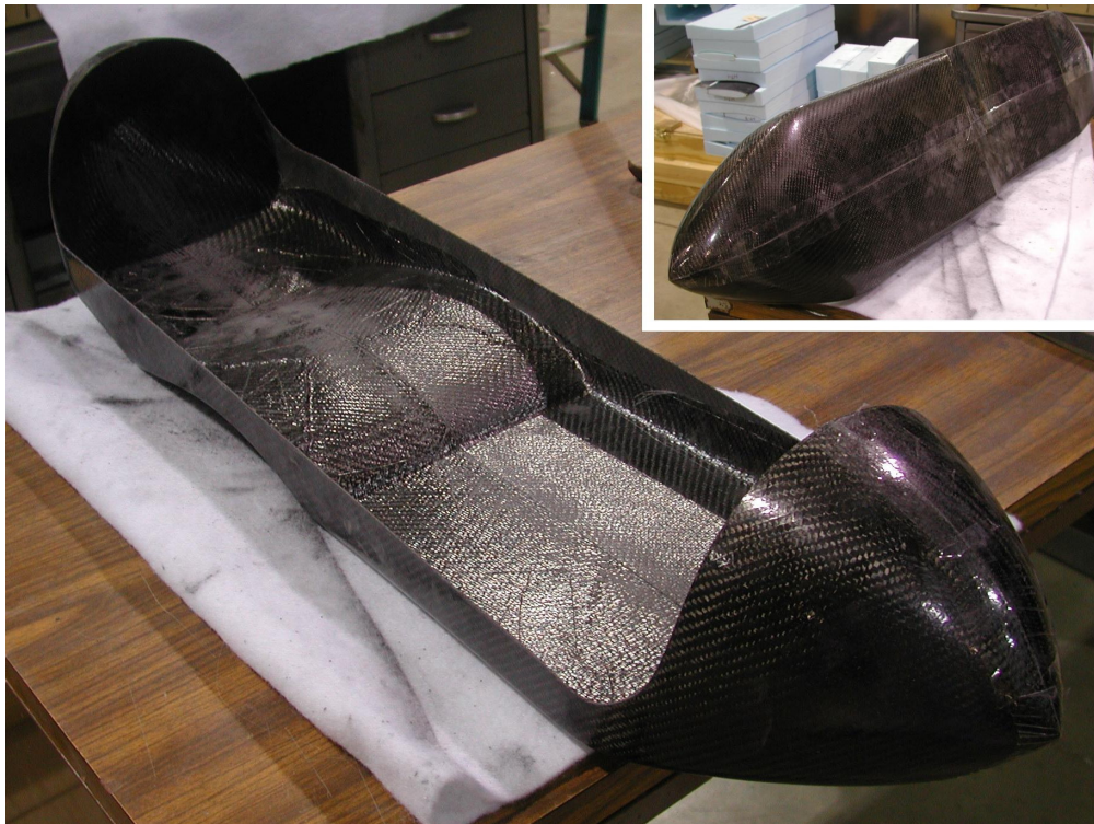
Figure 7.7. Fuselage Joining – taped seam, detail view top right.
