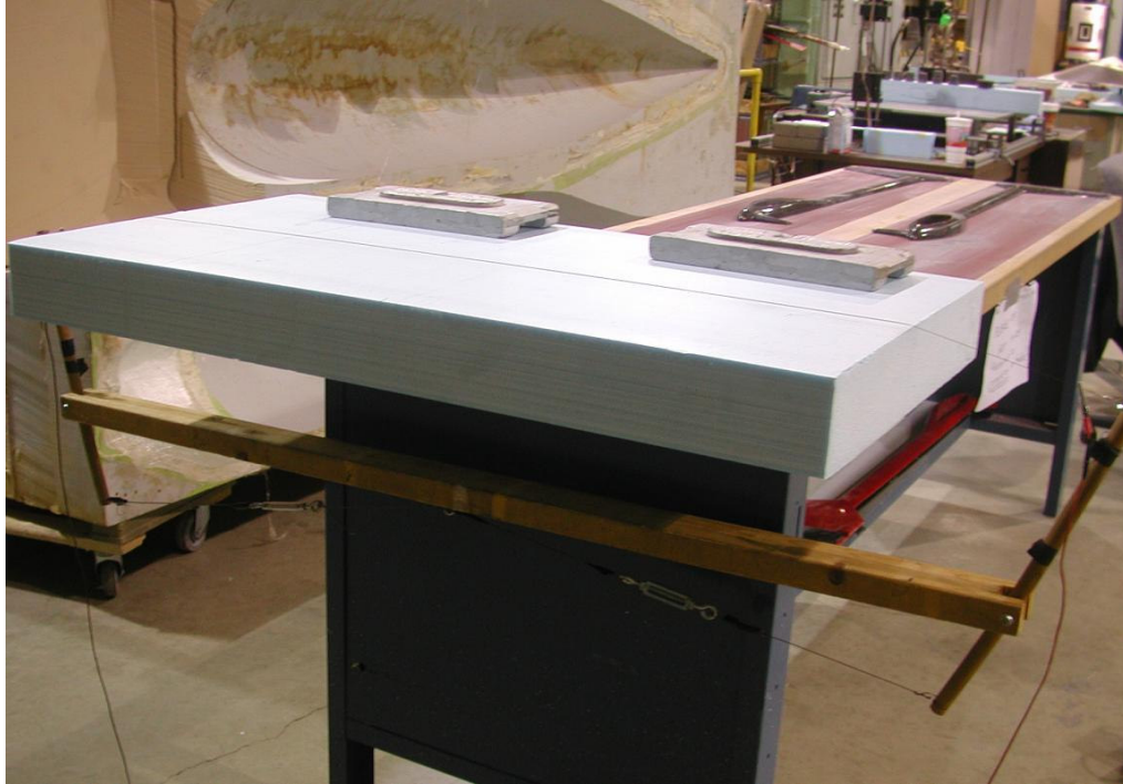
Figure 6.29. Wing Blank Being Cut with the Hot Wire Bow.
