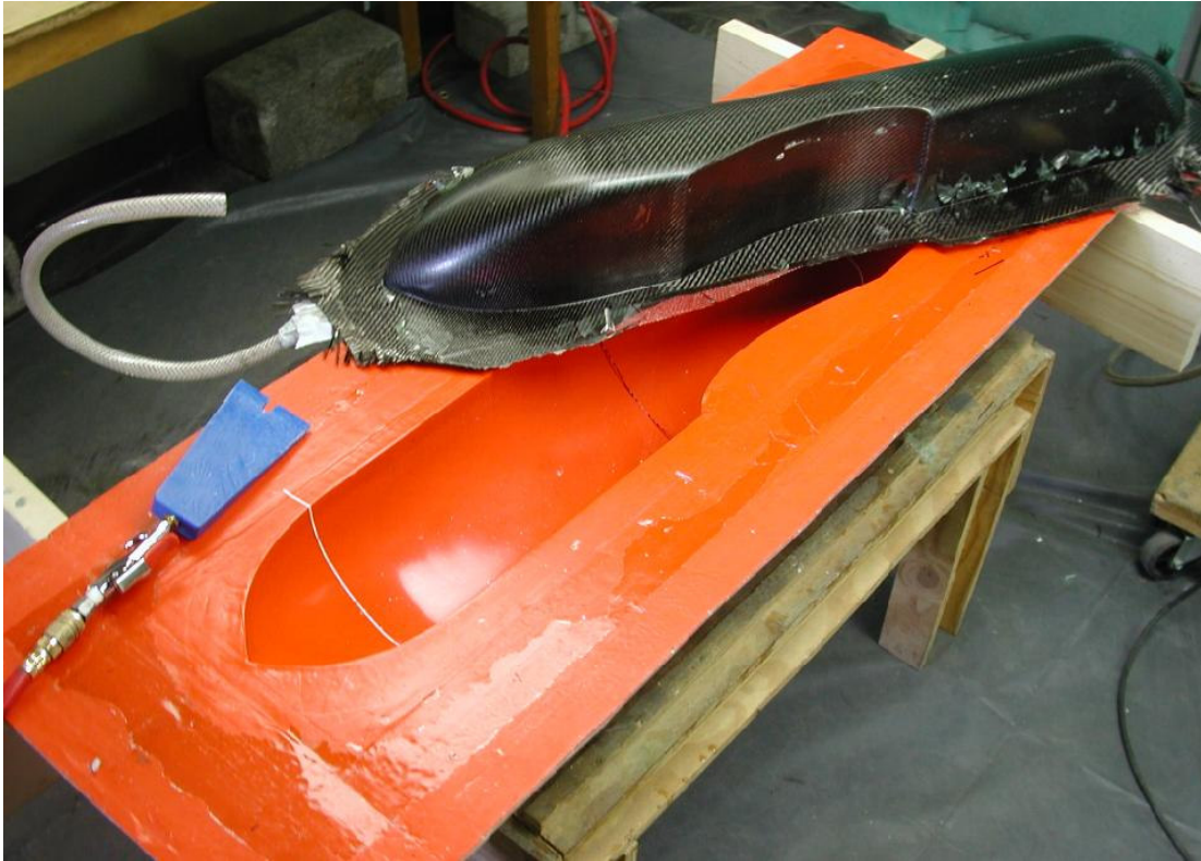
Figure 5.21. Fuselage Mold and Part – with PVA release and outlet port attached.
