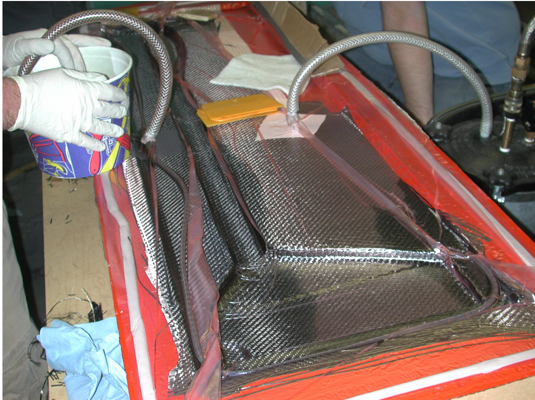
Figure 5.14. Resin Infusion in Progress – right boom half.
