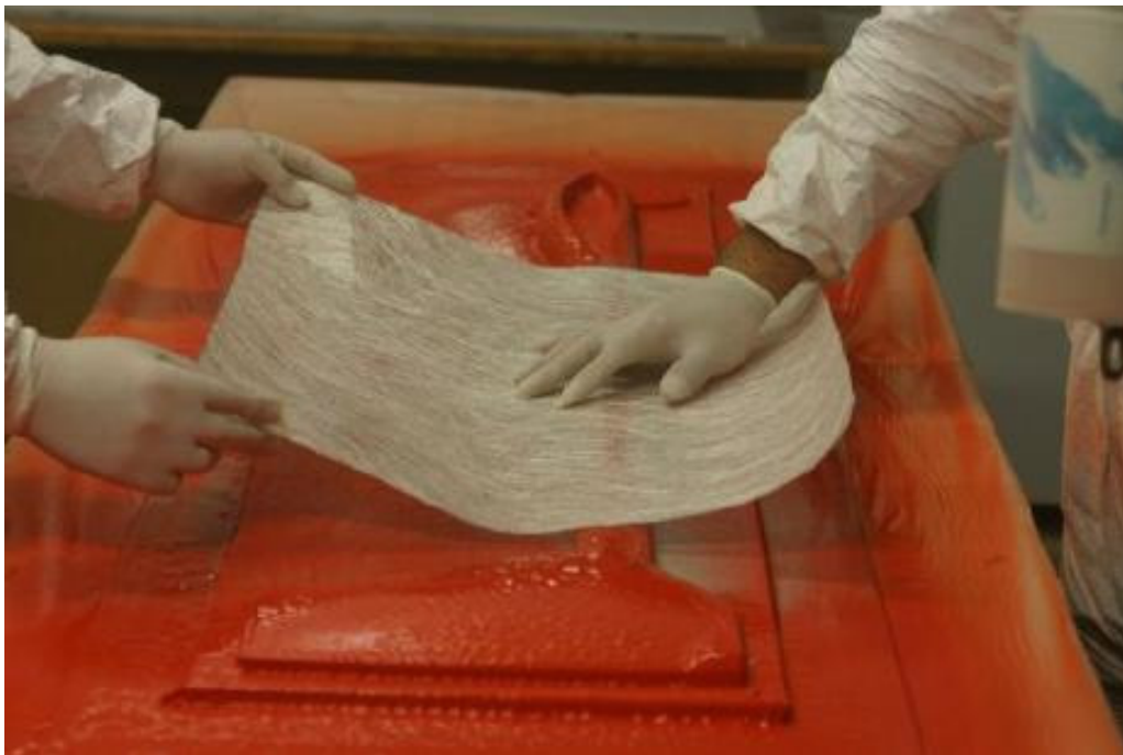
Figure 4.1. Strand Mat Sheet placed on bare Gel Coat.
