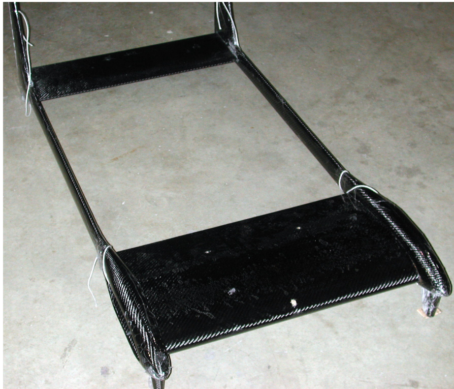
Figure 7.31. Twin Boom Sections Ready to be Joined.
