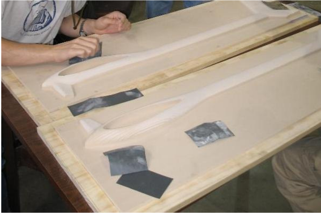
Figure 3.4. Sanding the Boom Molds.
