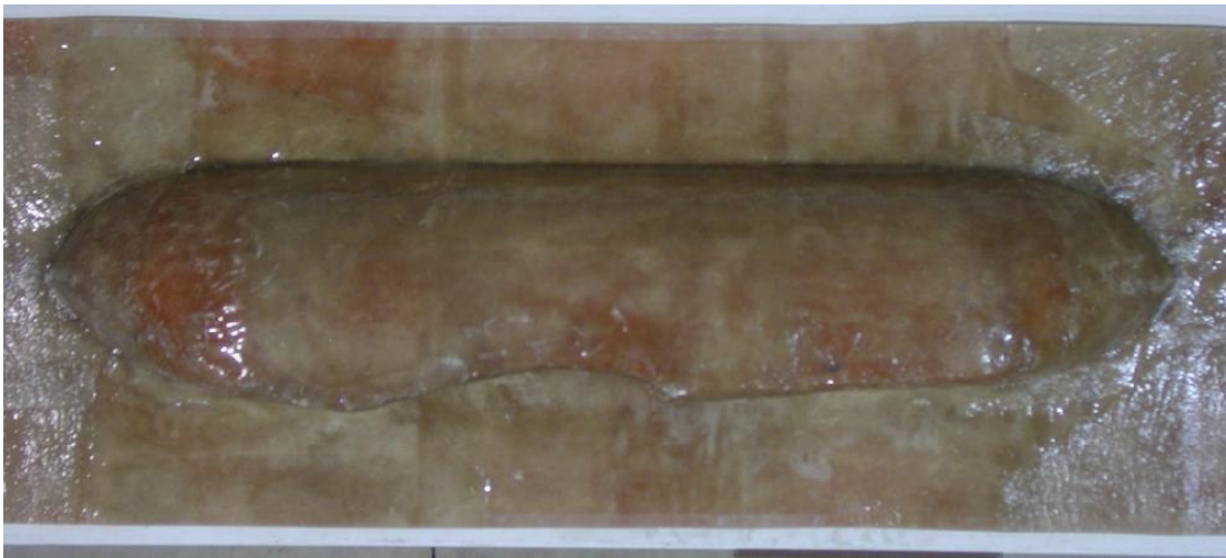
Figure 4.5. Finished Fuselage Mold – reverse side.
