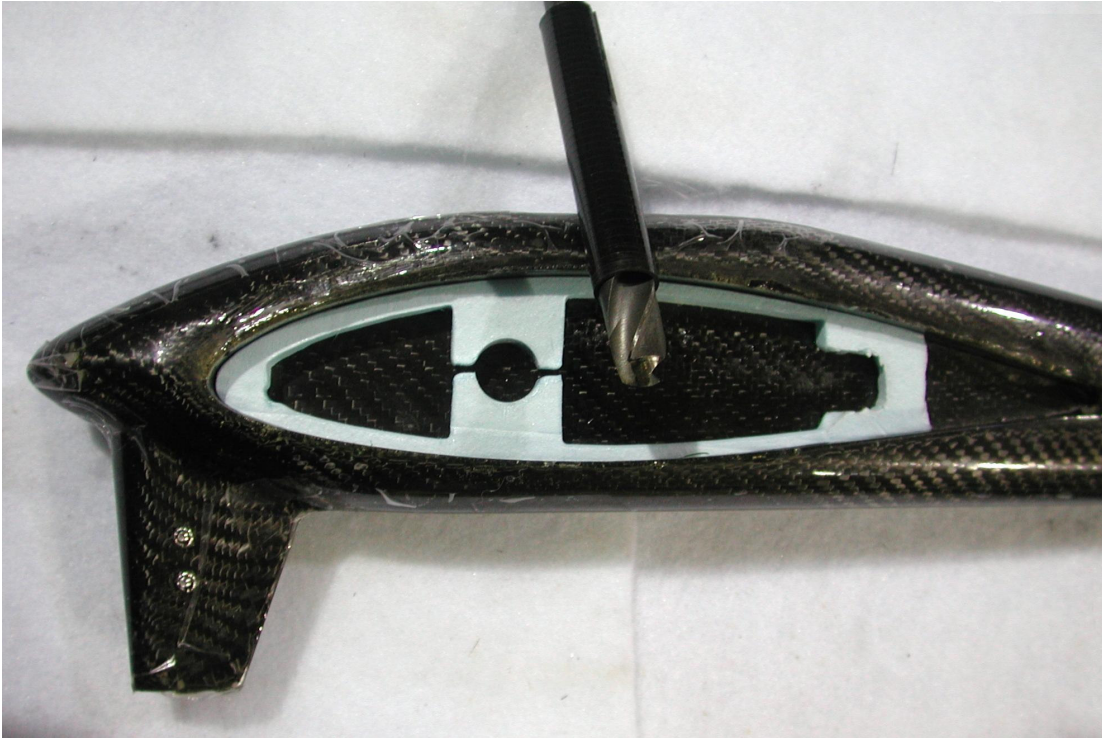
Figure 7.23. Spar Hole Template in Place – ready to locate spar hole.
