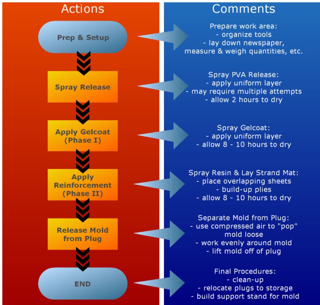
Flowchart 4.1. Mold Making – breakdown and comments.
