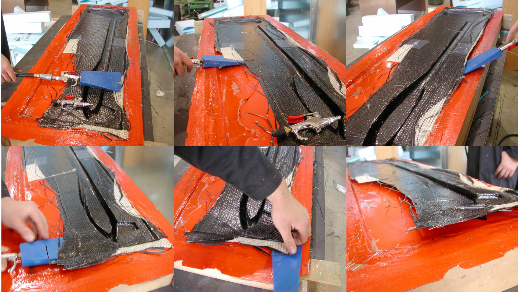
Figure 5.18. Boom – de-molding process (from top left to bottom right).
