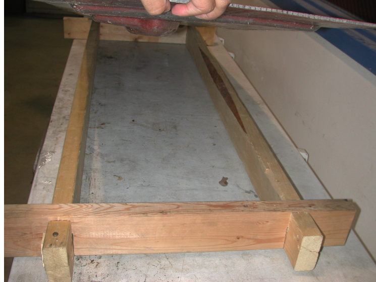
Figure 4.6. Boom Mold – support 2” by 4” frame.
