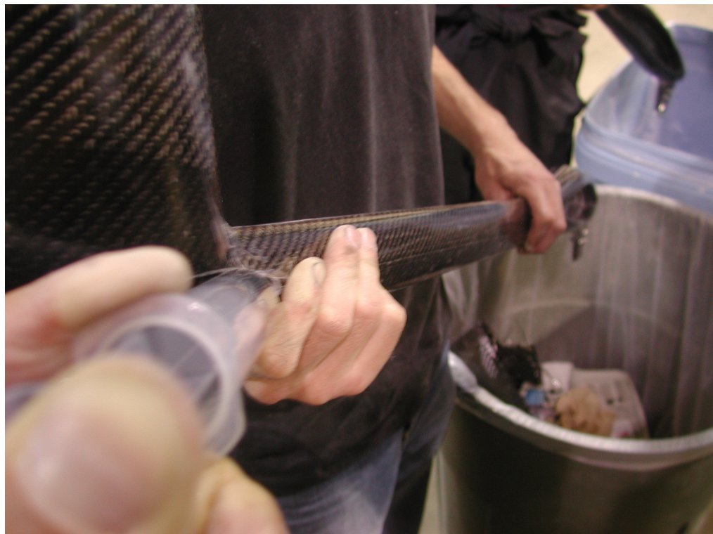
Figure 7.13. Boom Joining – resin being injected.
