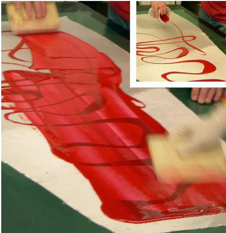
Figure 6.11. Outboard Wing-Section – wet lay-up, detail view top right.
