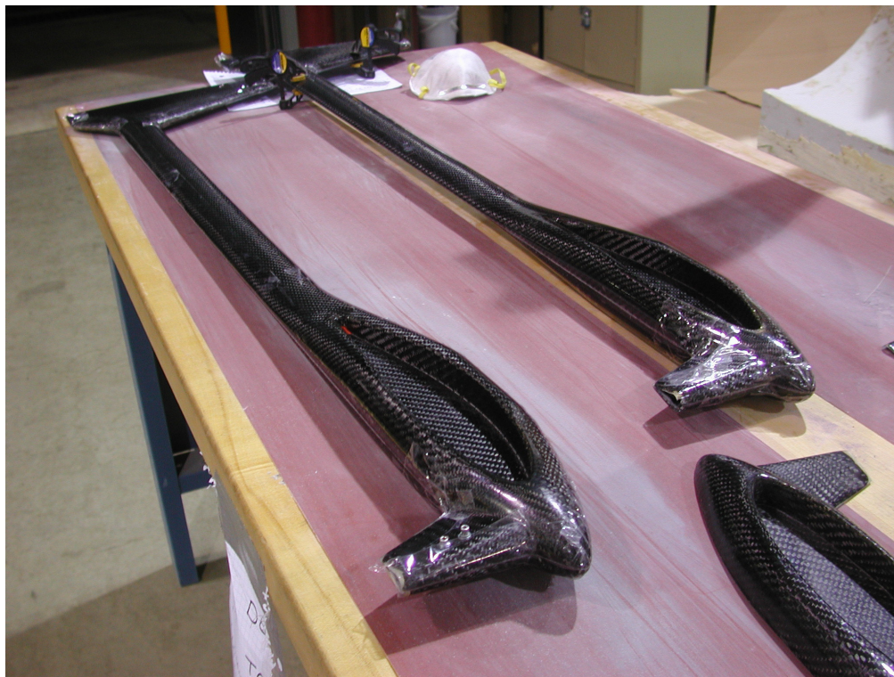
Figure 7.14. Left and Right Boom Pair Injected with Resin.
