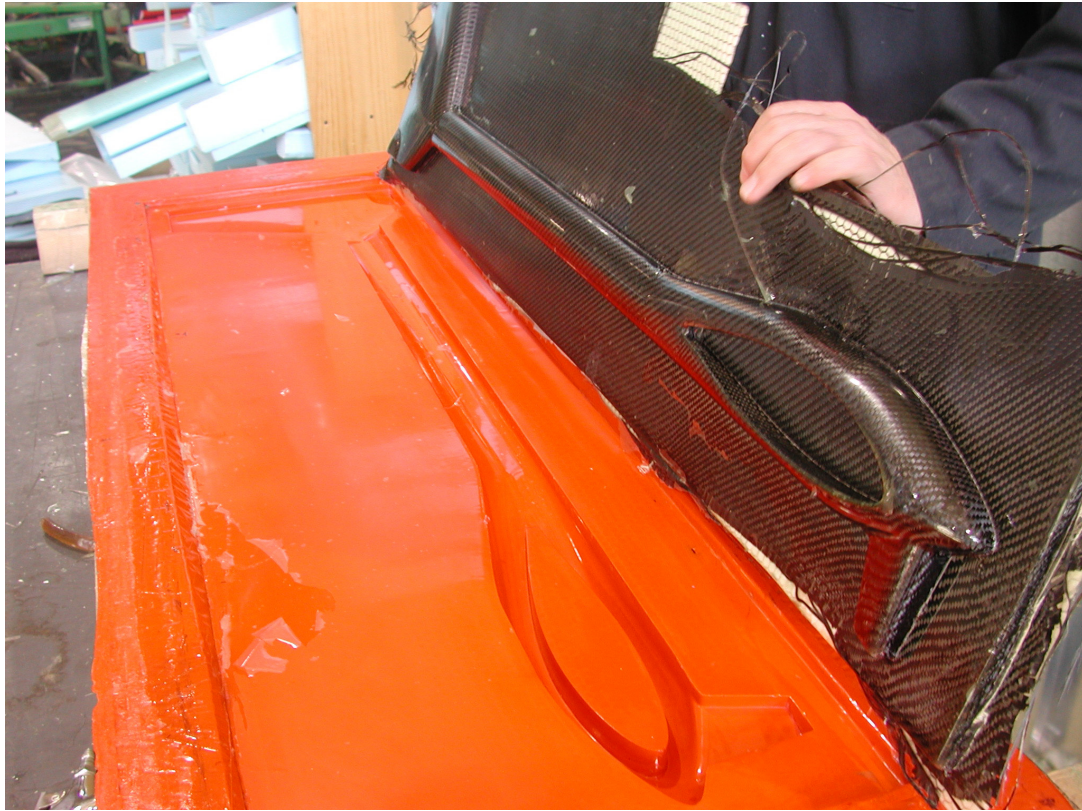
Figure 5.19. Boom – de-molded part with release film.
