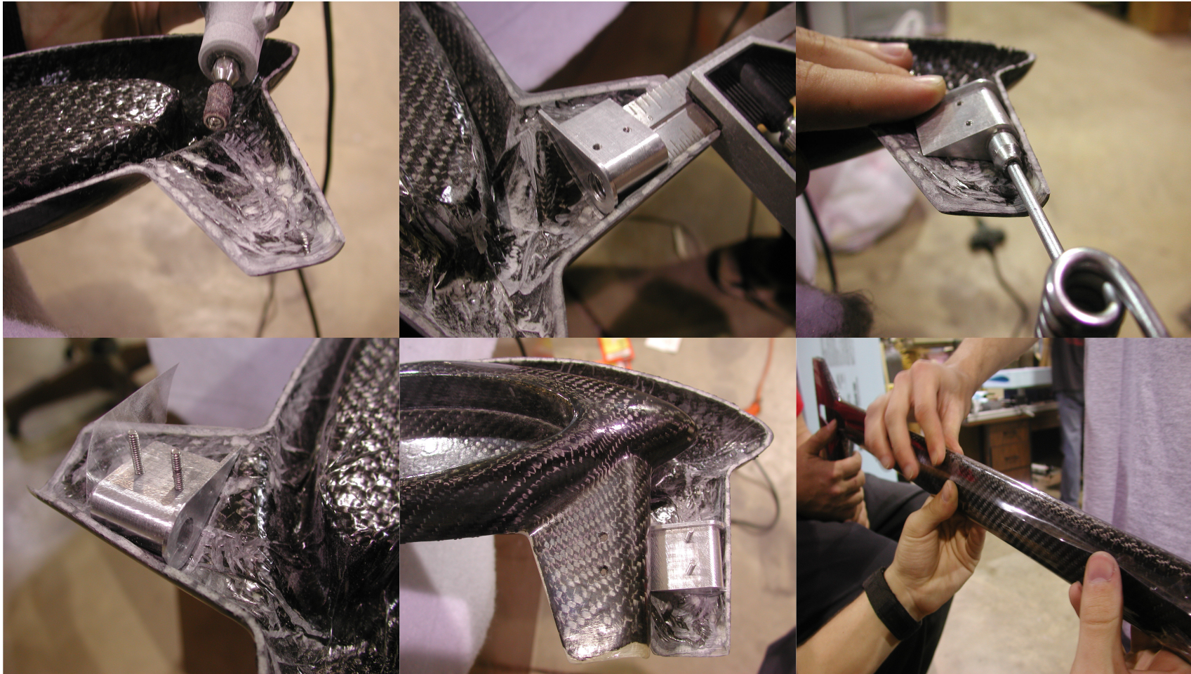
Figure 7.11. Installation of Main Strut Interface (from top left to bottom right).
