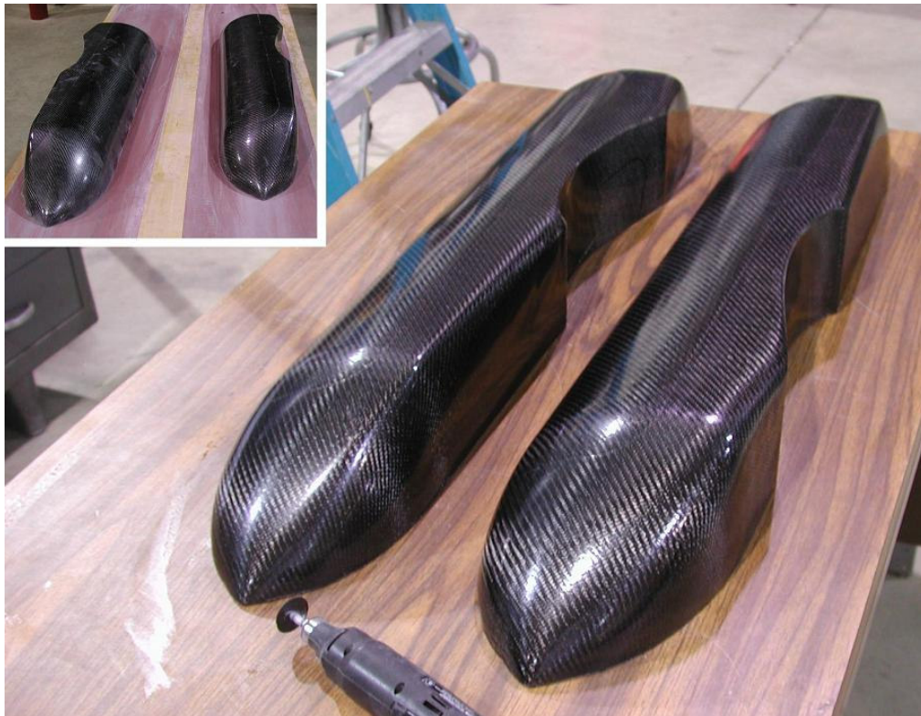
Figure 7.4. Fuselage Ready for Hatch Cutout – fine sanding, detail view top left.
