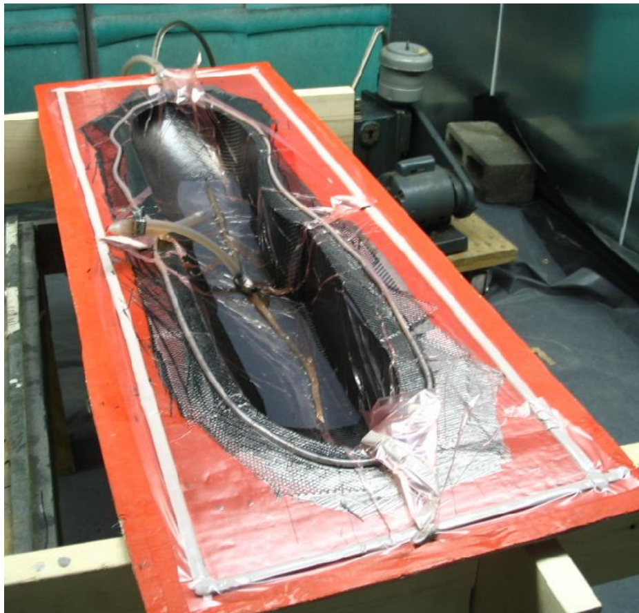
Figure 5.17. Fuselage Resin Infusion Complete.
