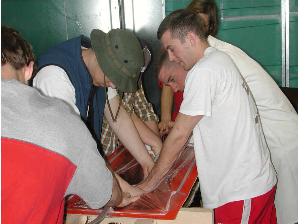
Figure 5.22. Working reinforcement into mold cavity.
