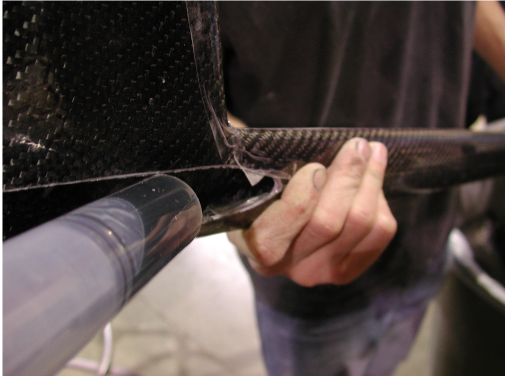
Figure 7.12. Boom Joining – resin being injected (close-up).
