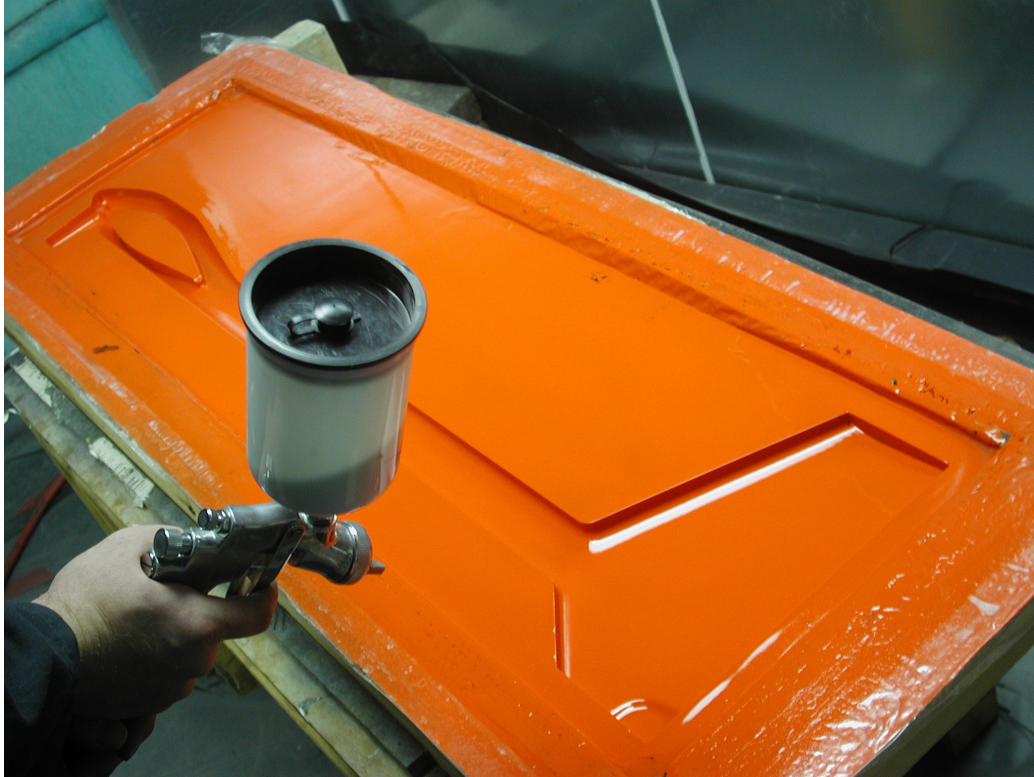
Figure 5.2. Boom Mold (Right Half) Being Sprayed with PVA – with tape along flange border.
