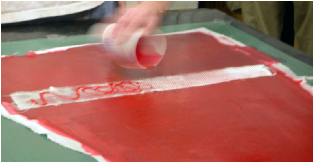
Figure 6.12. Outboard Wing-Section – reinforcement strip wet lay-up.
