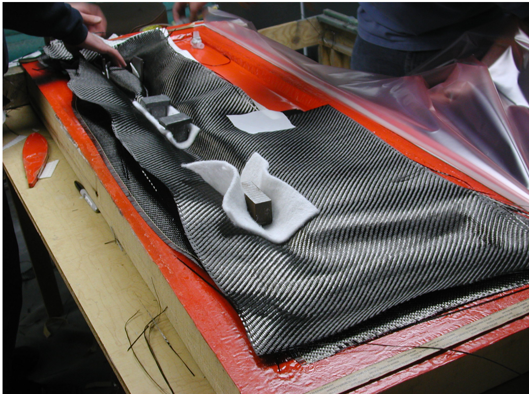
Figure 5.8. Carbon/Infusion Medium/Carbon Sandwich – worked into boom.
