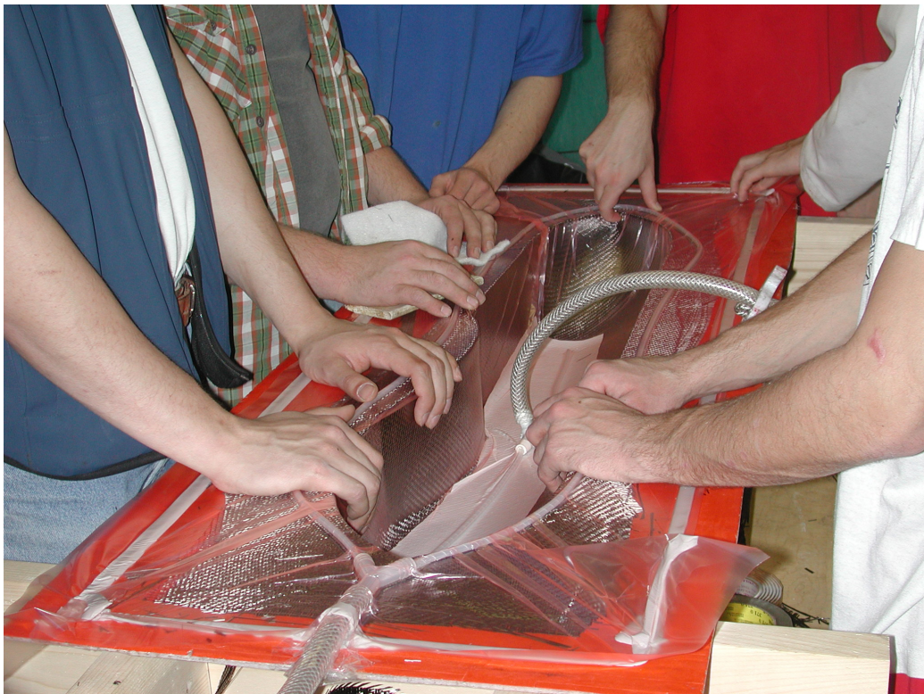
Figure 5.23. Vacuumed part – check for bridging.
