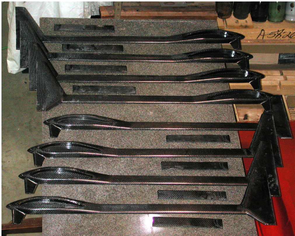
Figure 7.6. Rudder Cutout Complete for all Boom Halves.
