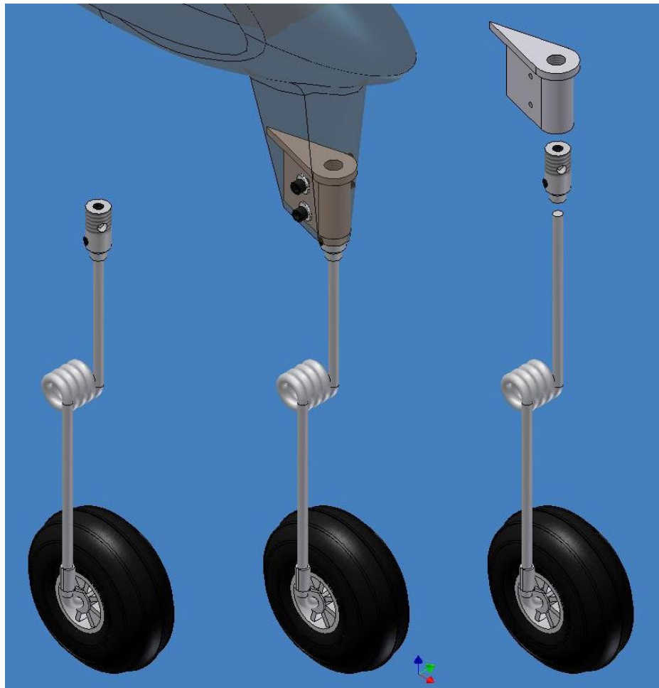
Figure 7.1. Main Landing Gear Assembly (see Figure 2.6).
