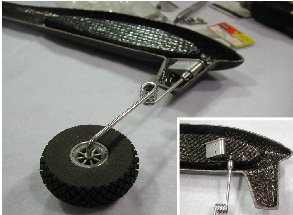
Figure 7.10. Landing Gear Interface – detail view bottom right.
