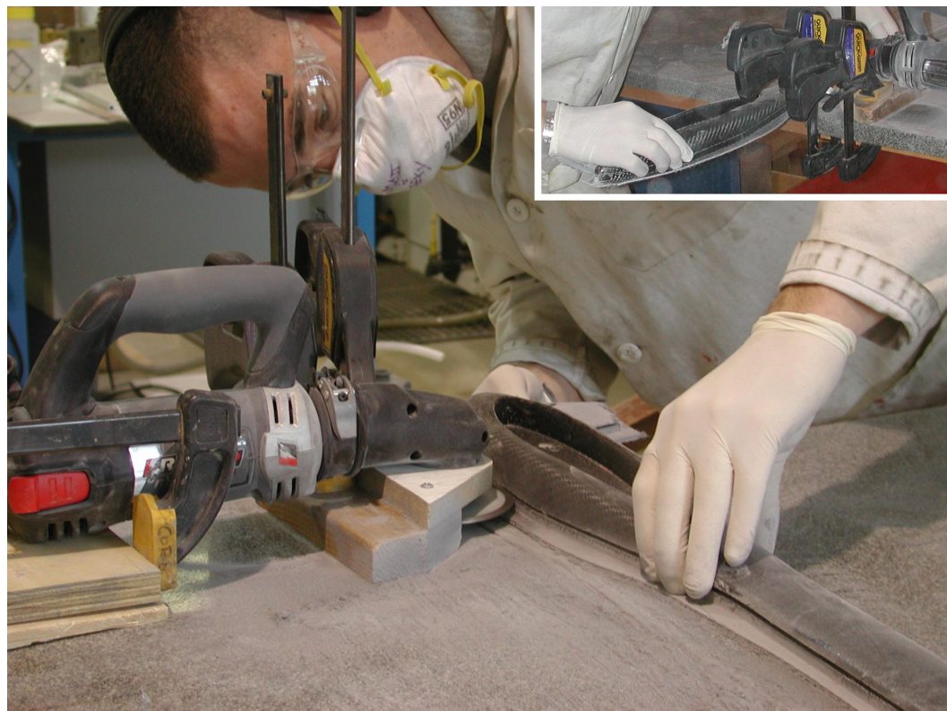
Figure 7.3. Boom Trimming in Progress – inscribed line detail view, top right.
