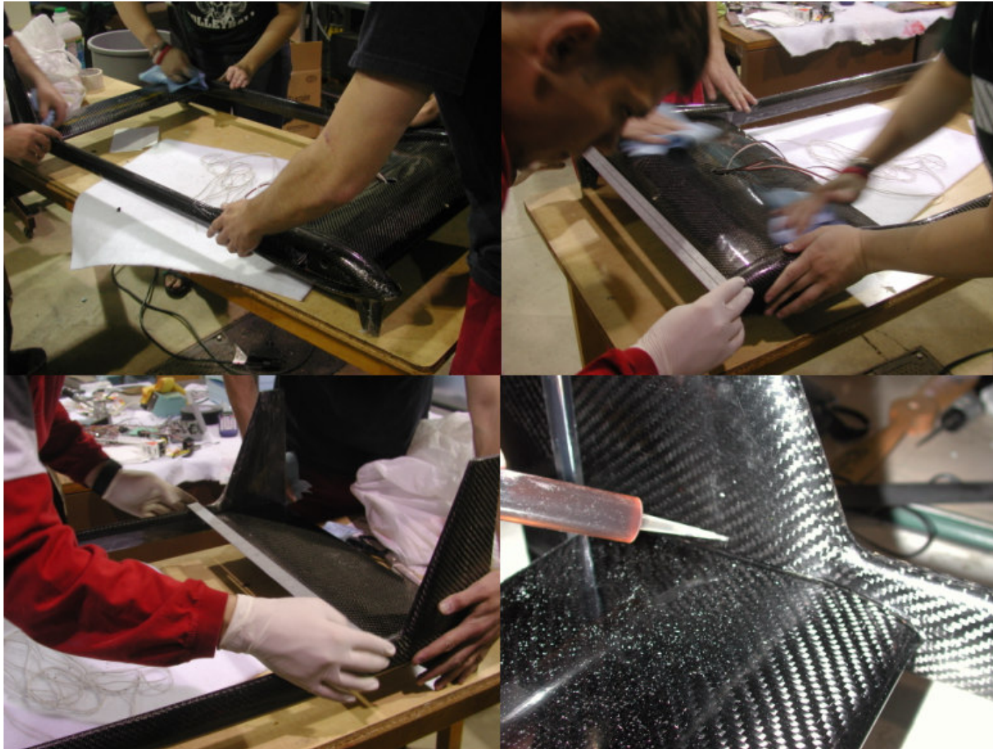
Figure 7.33. Twin Boom Assembly Joined.
