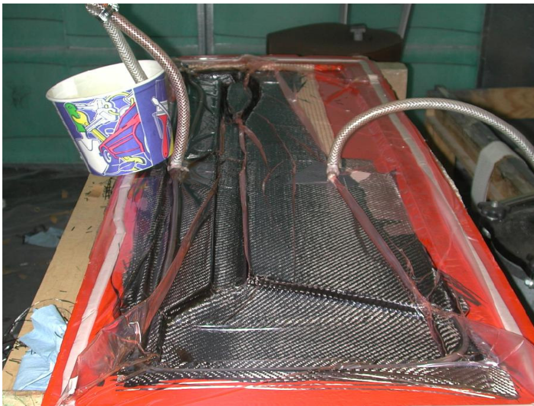
Figure 5.15. Boom Resin Infusion Complete.
