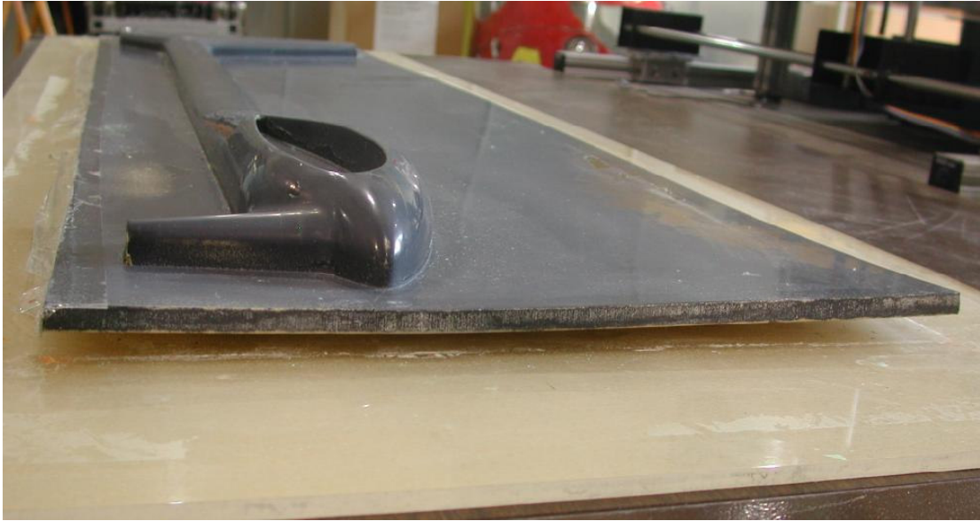
Figure 3.7. Boom Plug on Plexiglas Base Plate.
