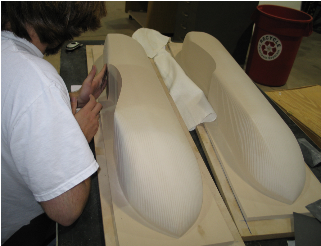
Figure 3.5. Sanding the Fuselage Molds.
