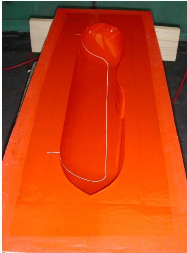
Figure 5.1. Fuselage Mold (Right Half) Sprayed with PVA – tape along flange border removed.
