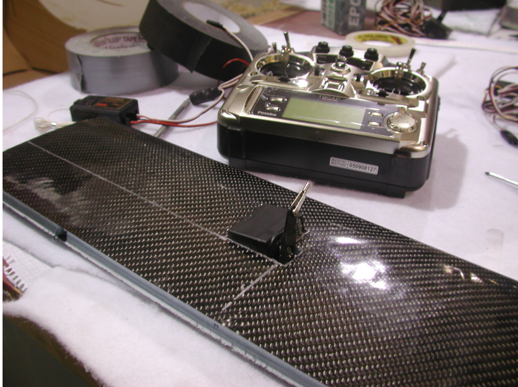
Figure 7.29. Elevator Servo Installed – ready for installation into wing foam-core.
