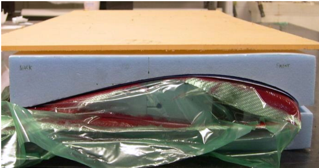
Figure 6.14. Outboard Wing-Section – wrapped and ready to receive weights.
