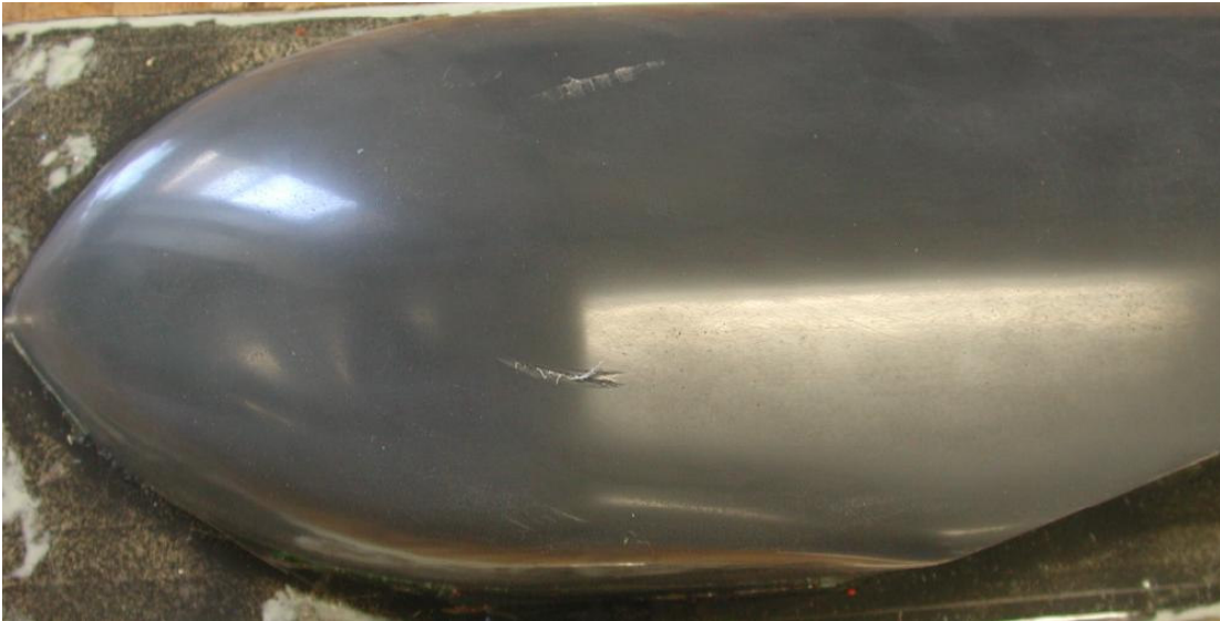
Figure 3.9. Surface Damage on Fuselage Plug.
