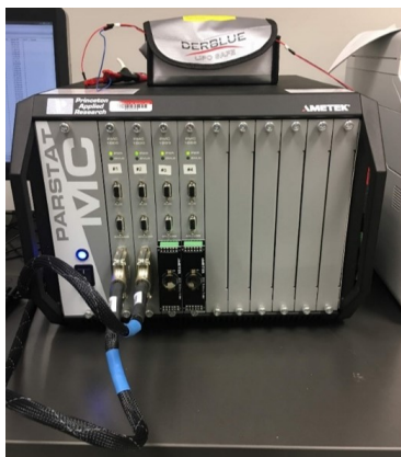
Figure 5.6: Solartron Analytical PARSTAT instrument used to collect transient data for coin cells.
