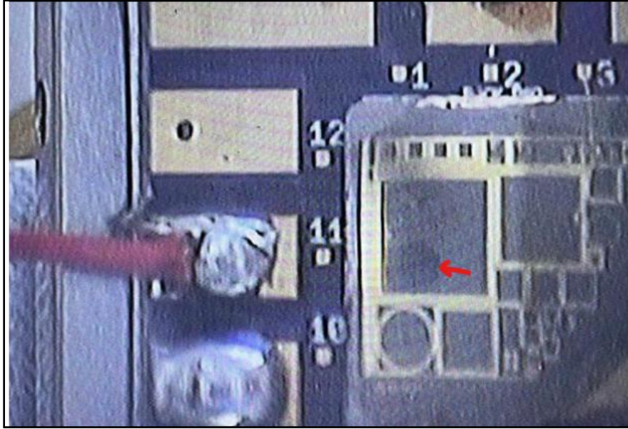
Figure 7.4: 1.4 nA beam exposure mark showing visible discoloration in the GaN device.
