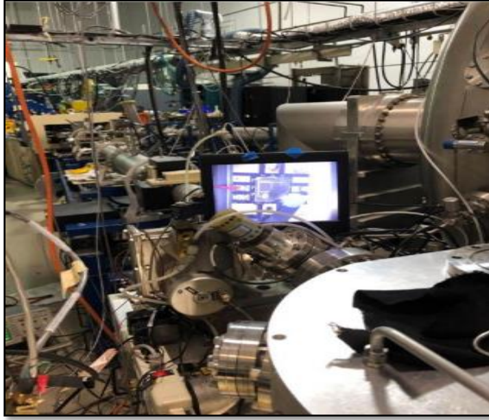
Figure 7.1: Alpha beam linear accelerator with a device package mounted in the vacuum chamber.
