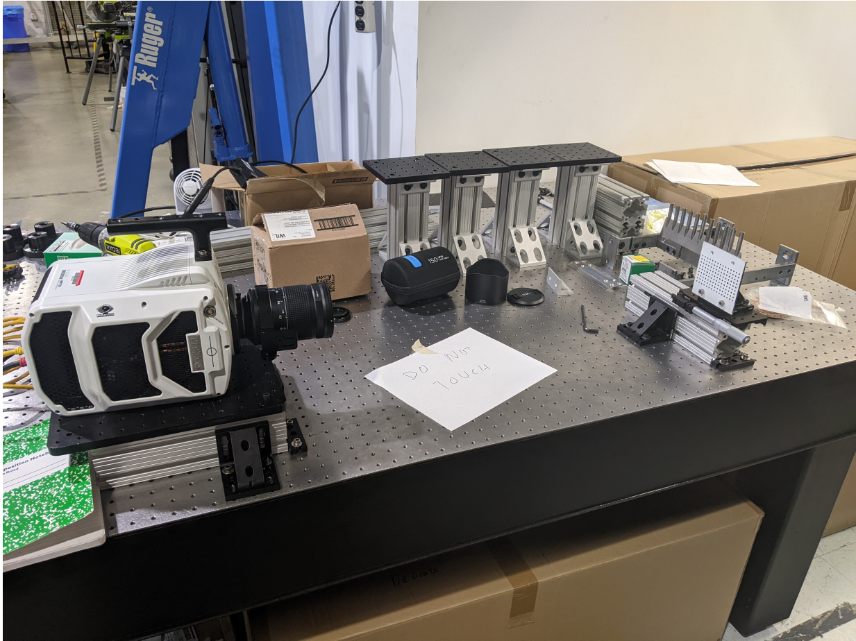
Figure 3.8: Photographic calibration setup with camera, linear stage, and marker plate.
