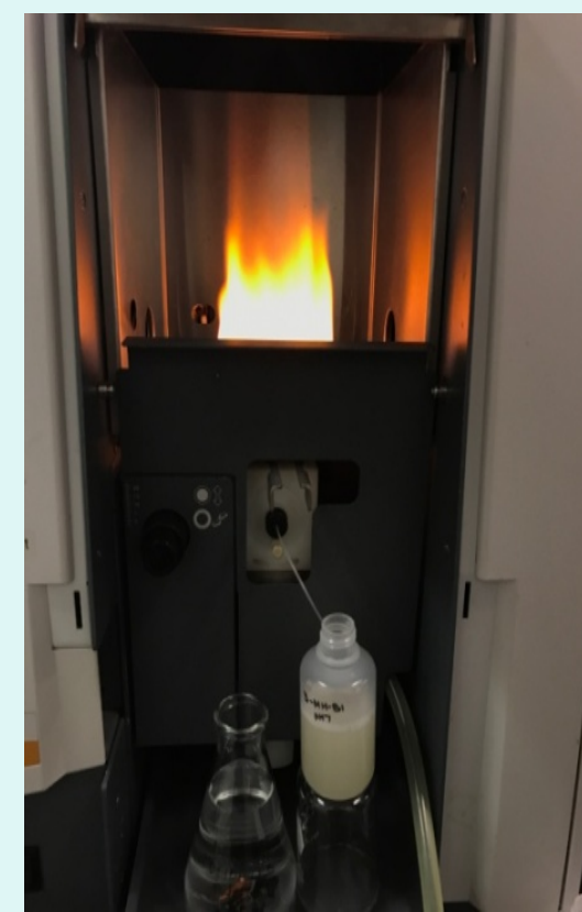
Figure 7 - Testing with FAA Spectrometer
