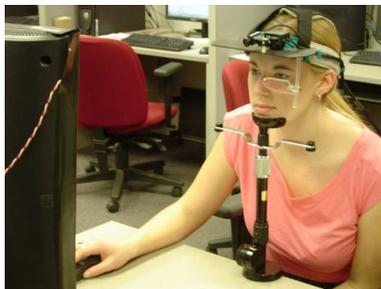
Figure 2.1: *Experimental setup for the user study with the ISCAN ETL-500 eye-tracker.*
