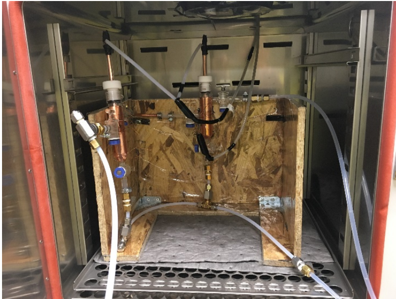
Figure 4-22: Separation tubes attached to the holder in the heating oven
