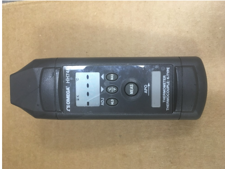
Figure 4-16: Thermometer: Omega HH74K
