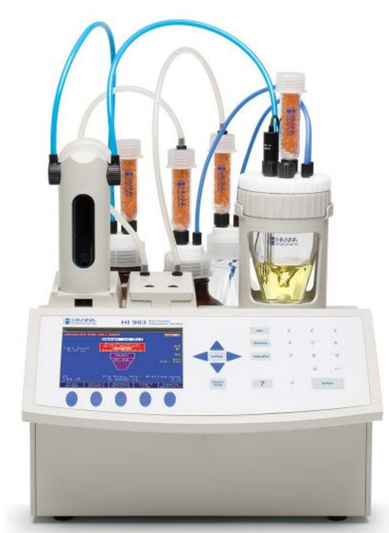
Figure 4-1: Coulometric Karl Fischer Titration
