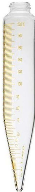
Figure 4-10: Cone-shaped separation tube of the heating centrifuge
