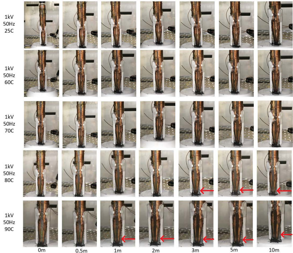
Figure 6-5: Temperature effect on the separations of 5% water-in-oil microemulsions
