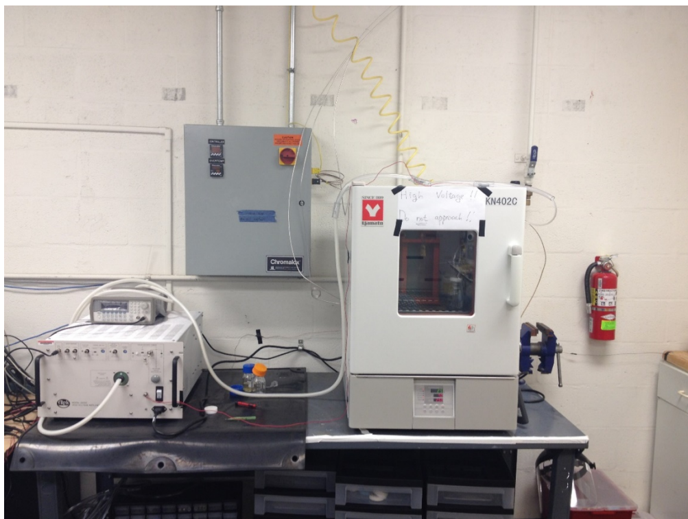
Figure 4-2: The whole static water-in-oil emulsion separation system
