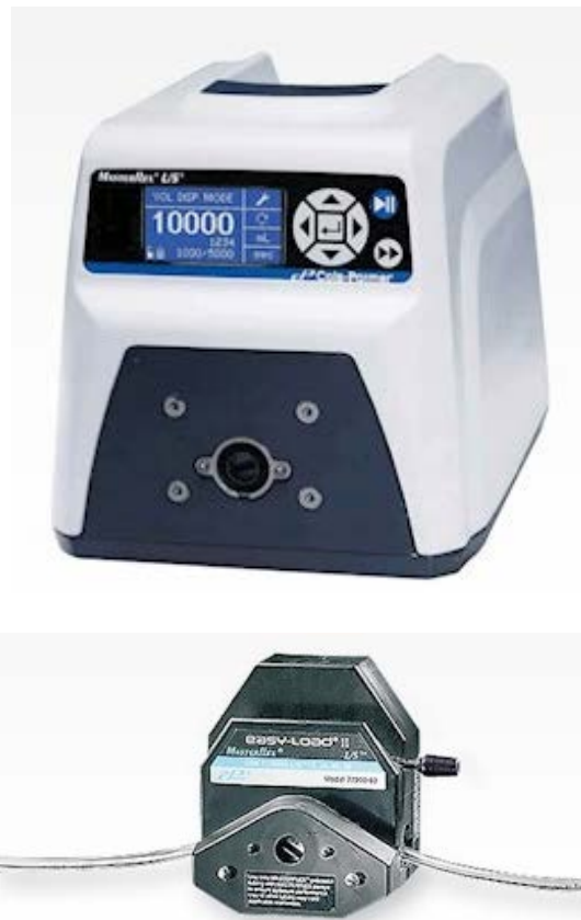
Figure 4-26: Peristaltic tubing pump (EW 07522-20 from Cole Parmer)
