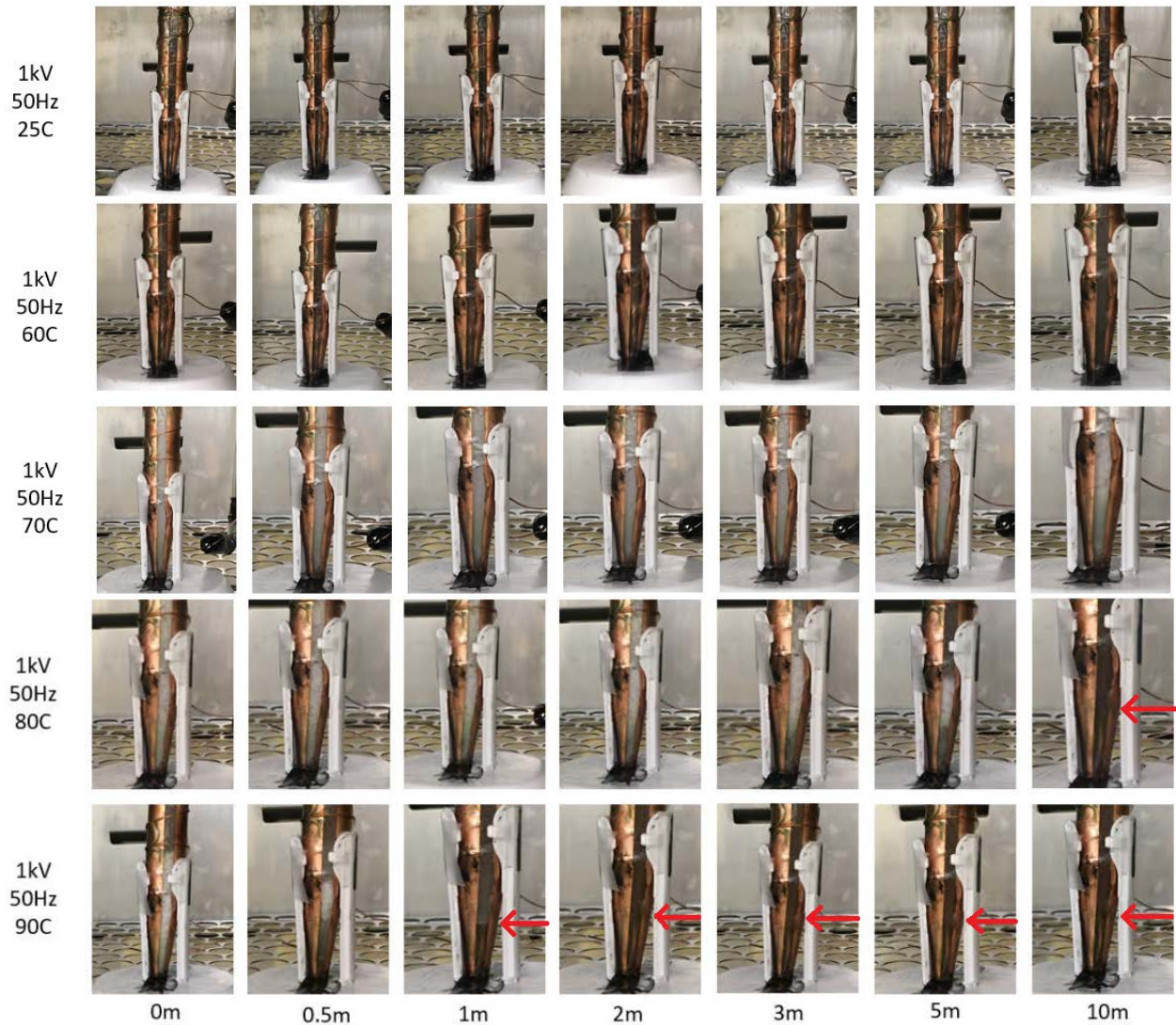
Figure 6-6: Temperature effect on the separations of 10% water-in-oil microemulsions
