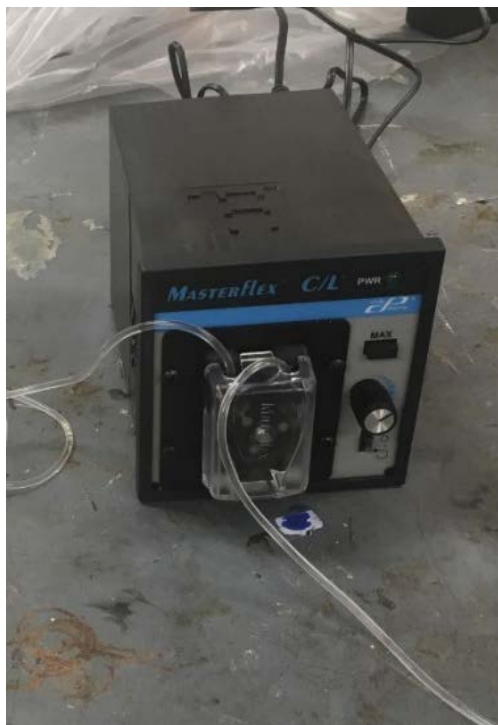
Figure 4-18: Peristaltic pump: Masterflex C/L 77122-24 from Cole-Parmer
