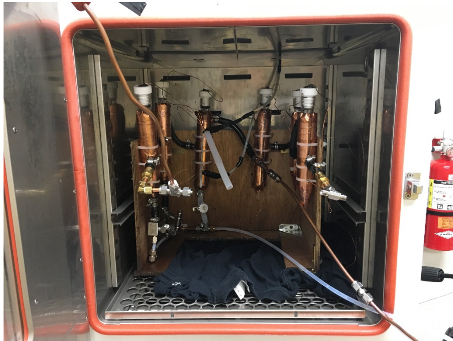
Figure 4-24: Series of the separation tubes in the heating oven
