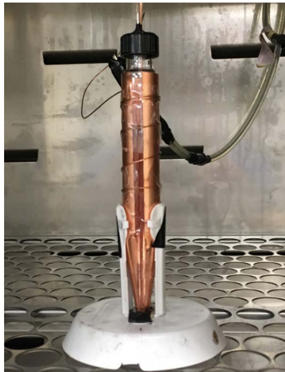
Figure 4-6: Cone-shaped cylindrical water-in-oil emulsion separator
