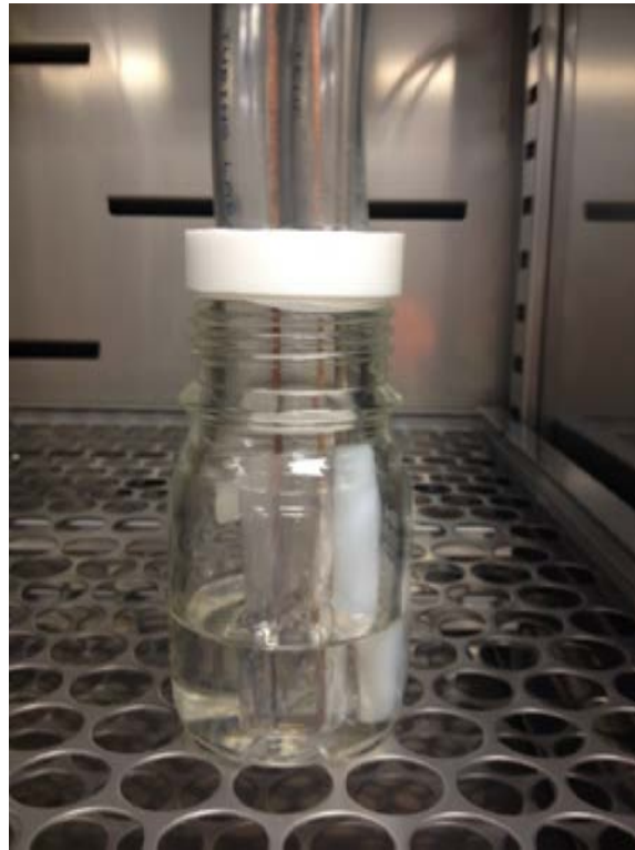
Figure 4-4: Two flat-plate electrodes water-in-oil emulsion separator
