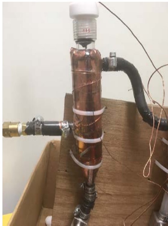
Figure 4-28: Dynamic separation tube for higher flow rate
