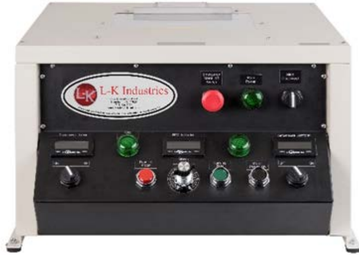
Figure 4-9: Centrifuge with heat treatment: Benchmark' 14 from L-K Industries
