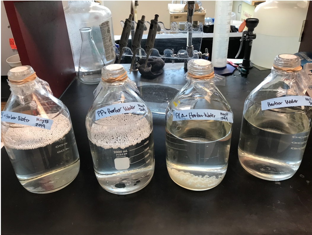
Figure 2.2. In vitro incubation of three different plastic microbeads and the water control on the benchtop. From left to right are PS, PP, PLA and the Harbor water, respectively.
