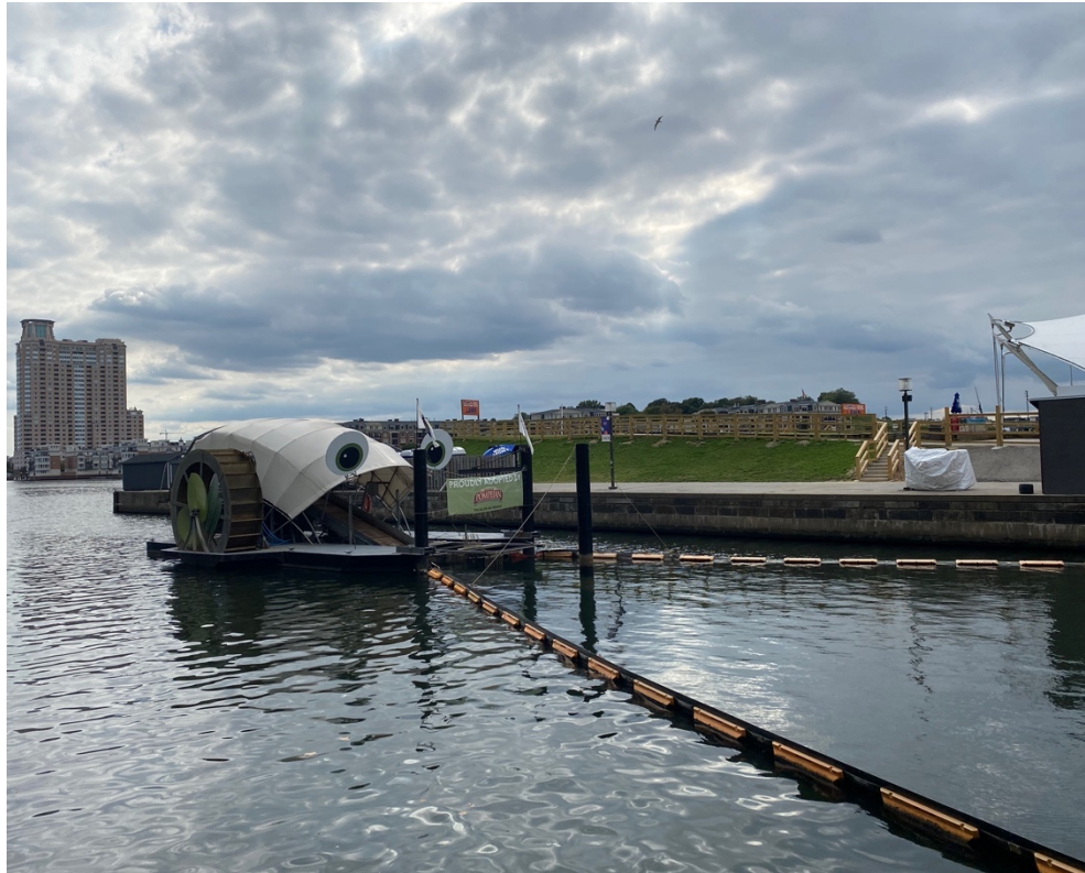
Figure 1.1. The anthropomorphic solar-powered trash collector in Baltimore's Inner Harbor Mr. Trash Wheel.
