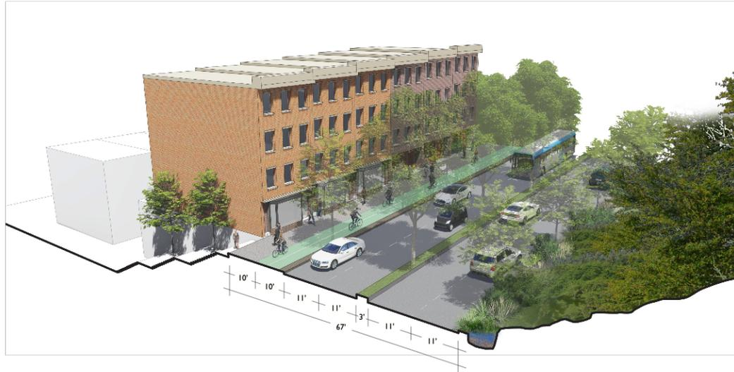
**Figure 7.18:** Raised highway transformed into an urban boulevard with streetscape for pedestrians and bikers. (Source: Author)
