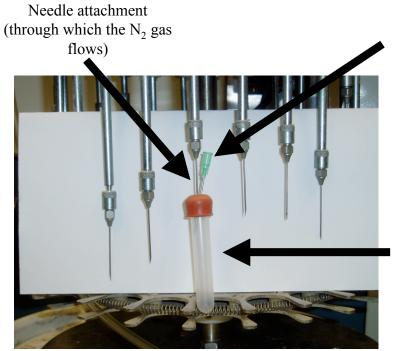
Needle allows oxygen to escape
