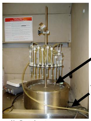
Needle attachment for sample tubes fitted with a rubber septum (see image below)
