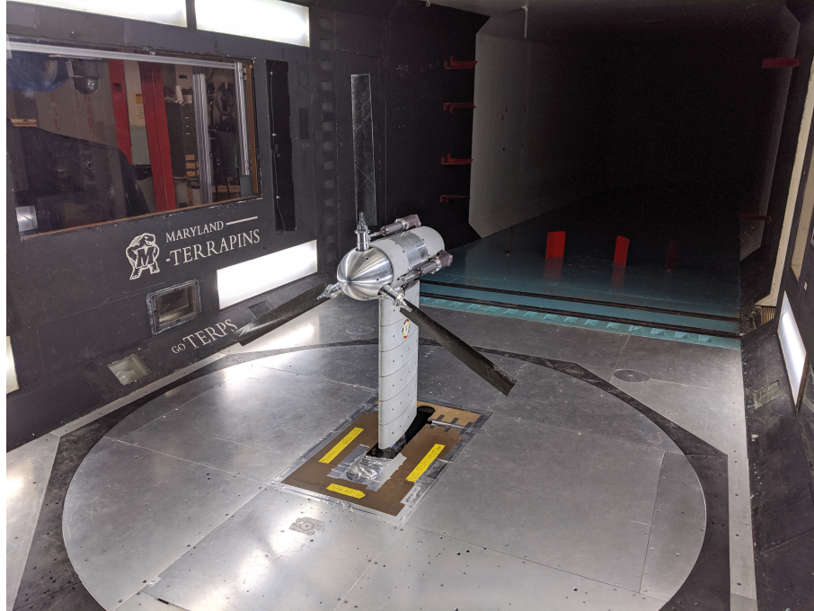
Figure 7.1: MTR installed in GLMWT 7.75 by 11-ft subsonic wind tunnel. November 2019.
