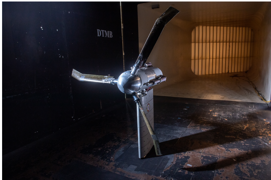
Figure 7.4: MTR installed in NSWCCD 8- by 10-ft subsonic wind tunnel. October 2021.
