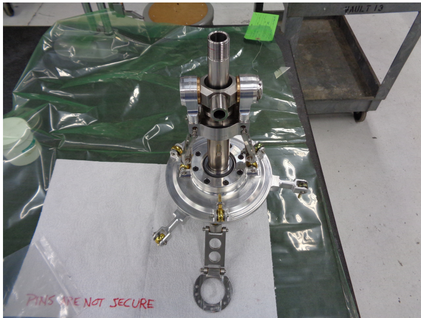
Figure 4.21: Swashplate and yoke mounted on rotor shaft.
