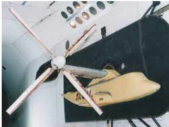
(b) 4-bladed, semi-articulated WRATS model.
