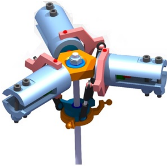
(a) CAD model of the FSD gimballed hub.
