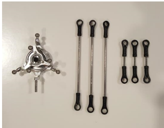
(c) Off-the-shelf RC helicopter swashplate and in-house fabricated linkages.
