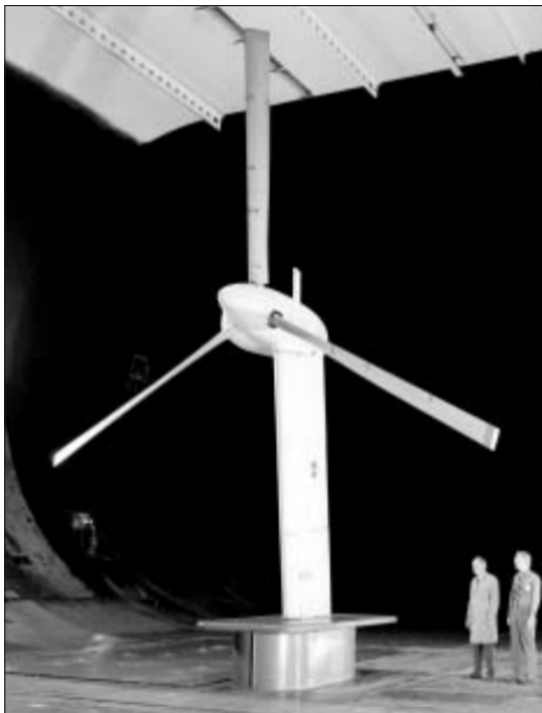
(a) Bell 25 ft. gimbaled hub proprotor.
