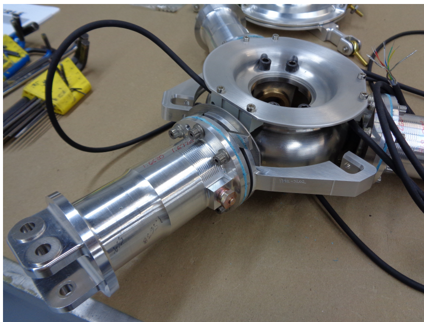
Figure 4.22: Pitch case and gimbaled hub component.
