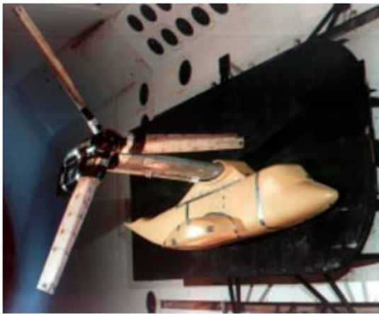
(a) 3-bladed, gimballed hub WRATS model.
