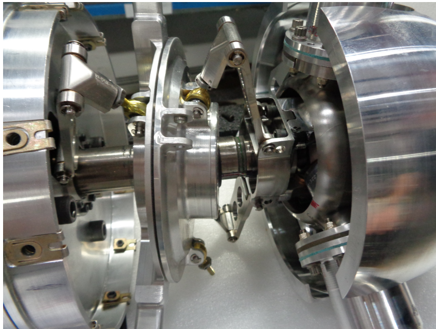
Figure 4.23: Rotor assembly mounted to pylon.
