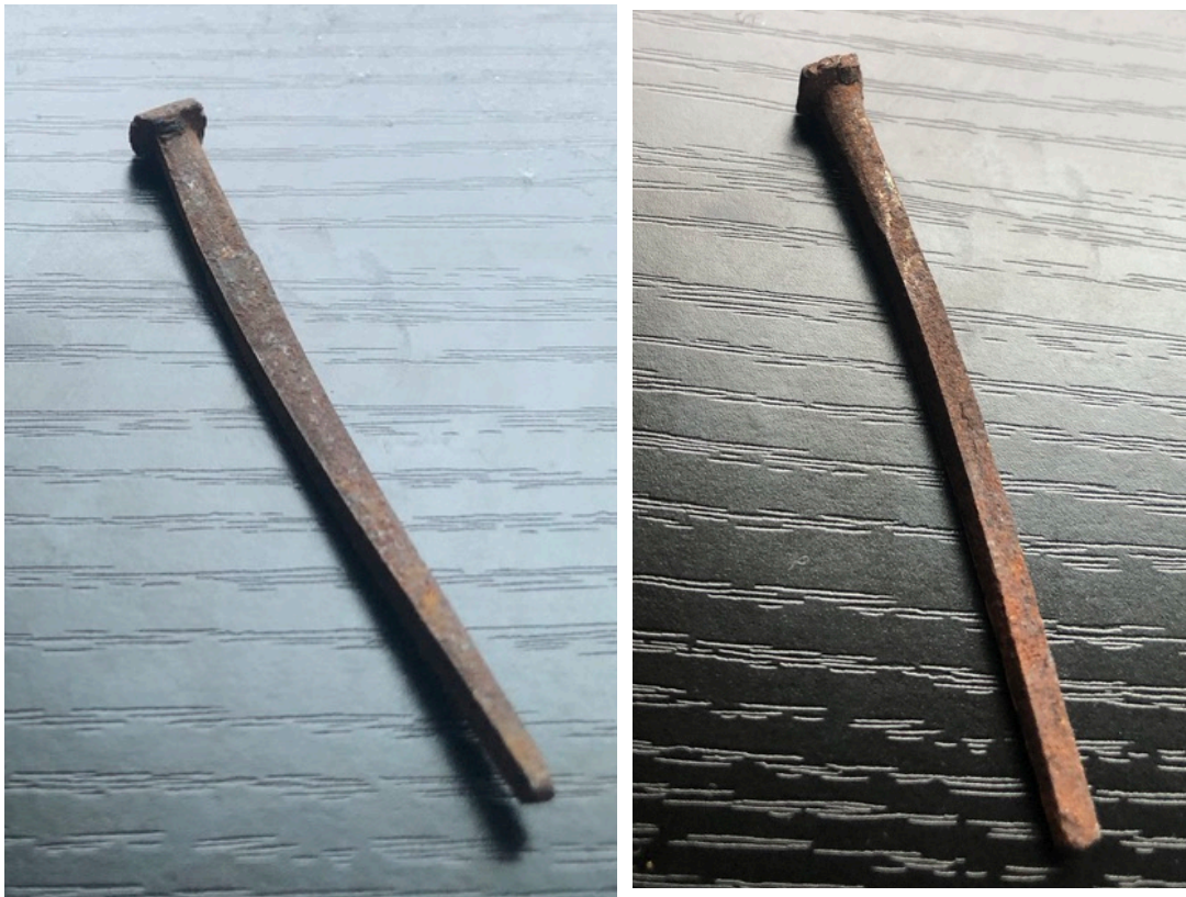
Figure 43. Face and side of a nail found in the half-story of Phase Two, indicating that the nail was side-pinched. (Source: Francesca Evans, 2022)
