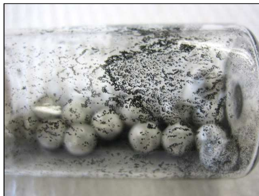
Figure 2.3: PtMo catalyst ink prepared with 5% Nafion solution and IPA after 1 hours of ball-milling.
