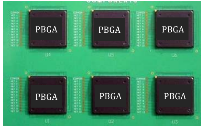
Figure 2-4: A sample of the test boards. Each board had six PBGA1156 components mounted on one side. High temperature wire was soldered to the copper pads on the board surface. These were used to monitor the 12 daisy-chain nets per component.
