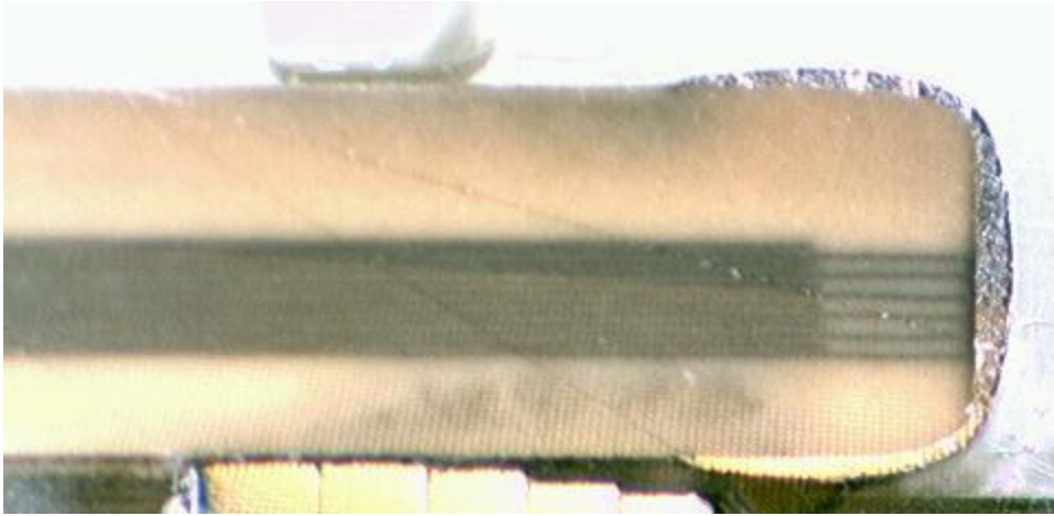
Figure 22: Propagation of stain into the ceramic dielectric of a standard termination MLCC
