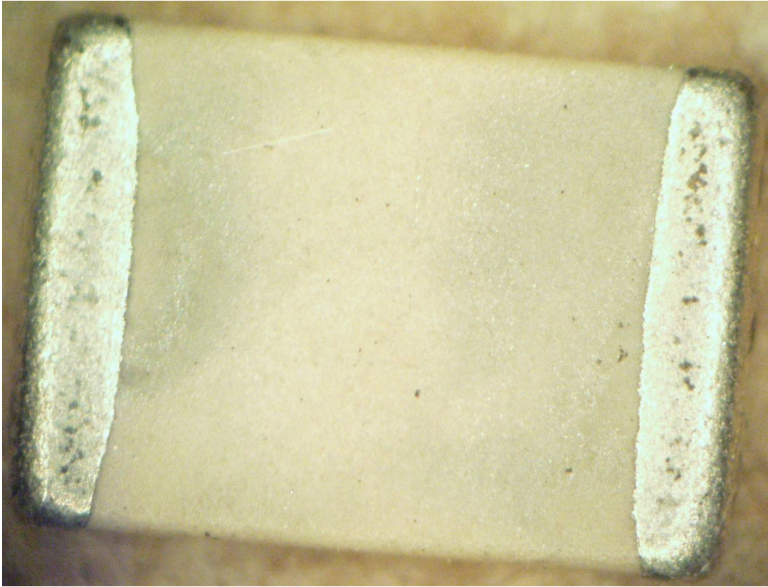
Figure 21: Image of standard termination MLCC with staining present in the dielectric
