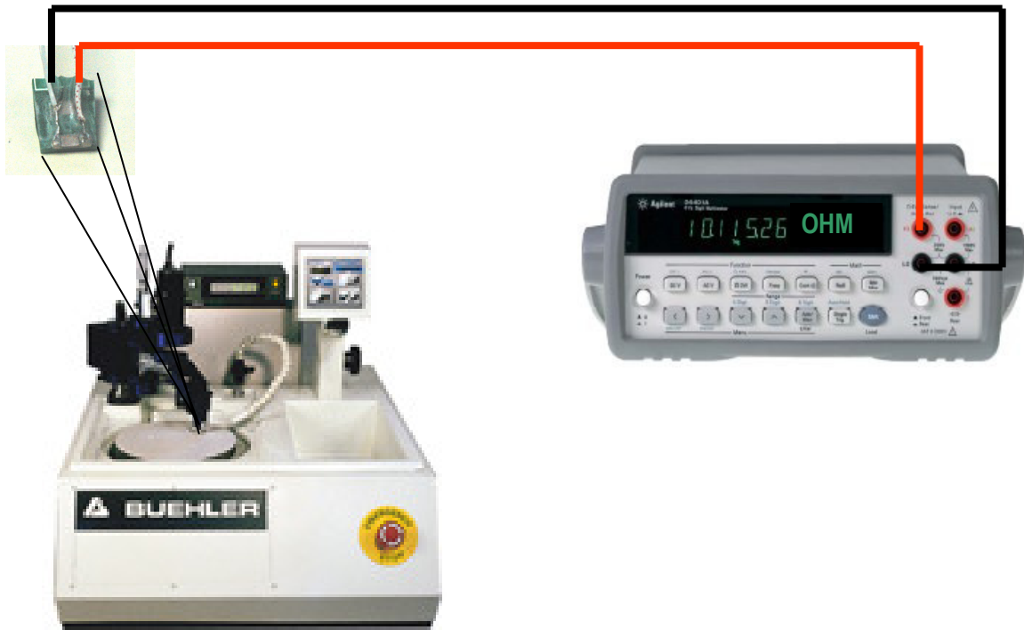
Figure 13: Cross sectioning equipment setup
