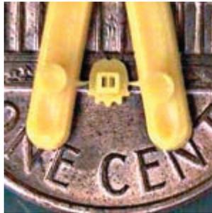
Figure 1.4 Piezoelectric sensor made using miniature molding methods [7]
