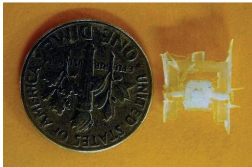
Figure 1.9 Example mesoscale revolute joint rendered ineffective due to excessive flash
