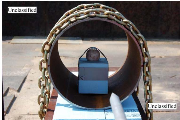
Figure 7.9. Explosive positioned on foam support.
