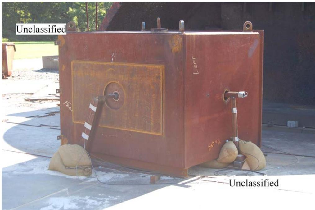
Figure 8.7. Confined blast post-test #1 exterior view of gage stands.
