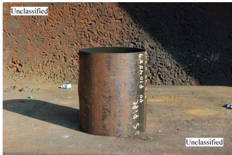
Figure 7.10. Post experiment center-line deformation of 12.75 in cylinder
