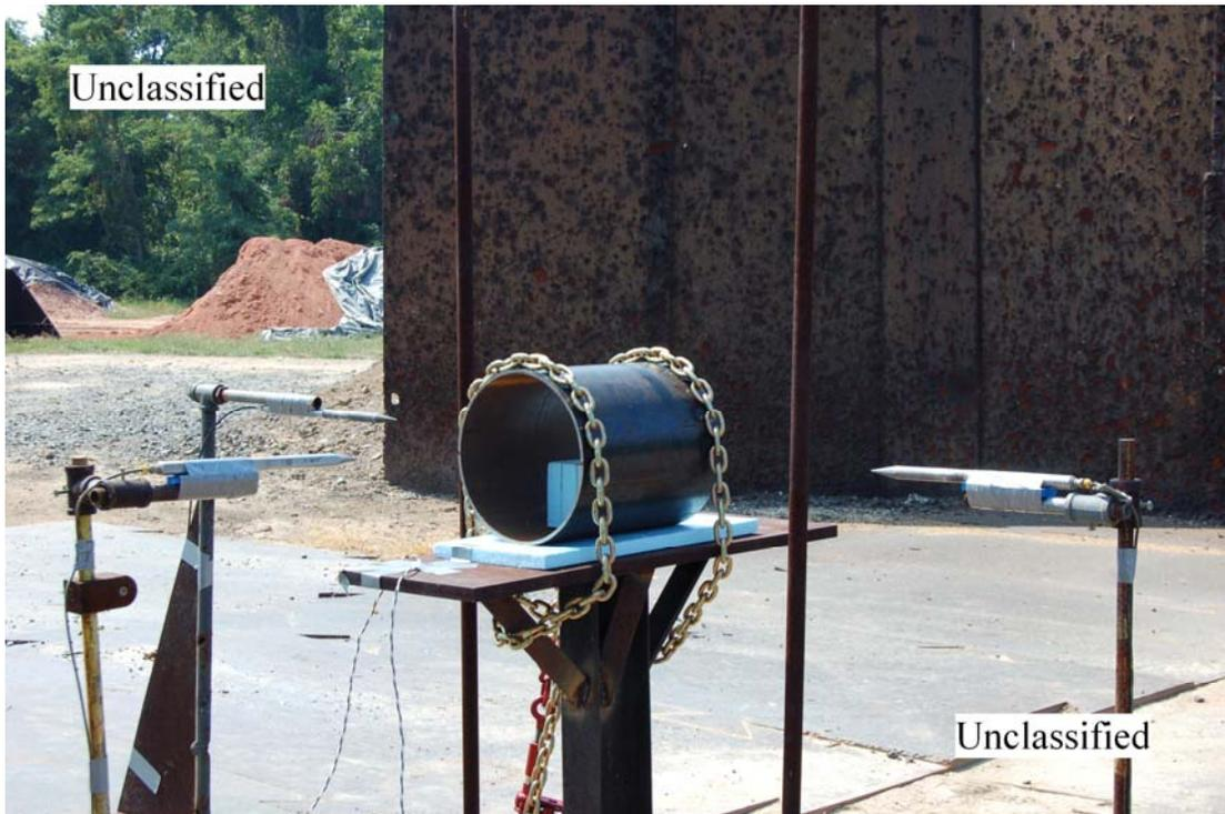
Figure 7.8. Field test set-up of 12.75 in diameter cylinder.
