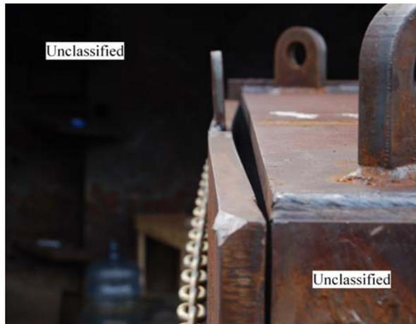
Figure 8.16. Confined blast post-test #2 post-test, chamber door deformation.
