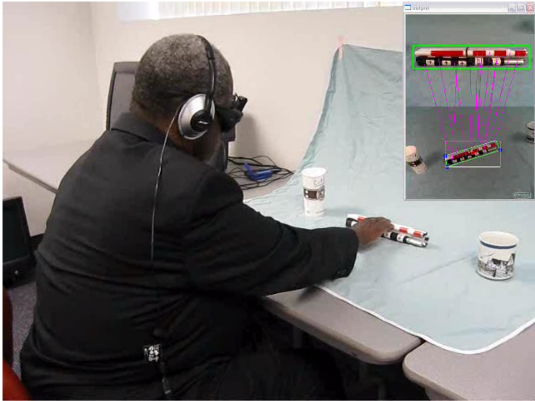
Figure 3.9: Subject locating a white cane. In the upper right, a representation of the computer vision algorithm
