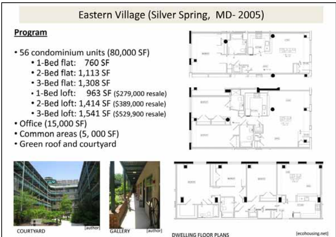
Figure 47: Eastern Village Program and Units Plans.
