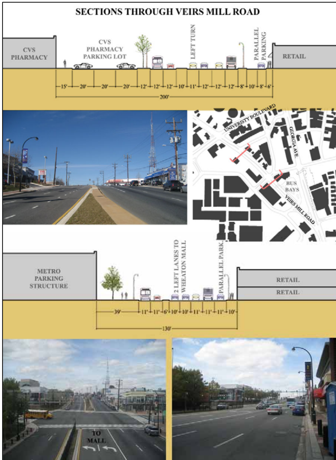
Figure 24: Sections Through Veirs Mill Road, Wheaton, MD. [Cesar Ramos, 2008] Current conditions show the lack of reinforcement of the street fabric. Buildings are not tall enough and they are not continuous. Also, there is a need for a greater set back that would allow better pedestrian circulation.
