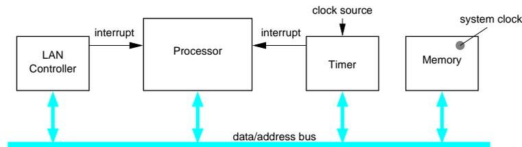
Figure 1: A node of a typical distributed real-time system
