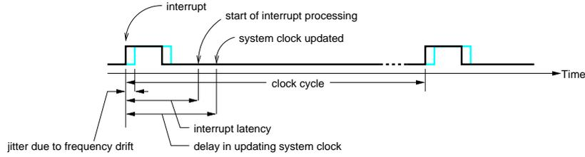
Figure 2: Timing diagram of external timer-based time management
