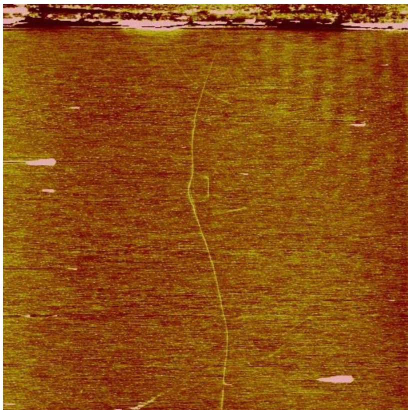
Figure A-1: An AFM topography scan of nanotube D2. The scan size is 22x22 \mu\text{m} . The cut in the nanotube near the bottom of the frame accidentally happened during the measurement. The other nanotube intersecting D2 is visible near the top.
