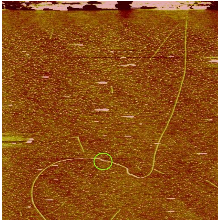
Figure 4-14: An AFM topography scan of nanotube D3, the scan is 35 \times 35 \mu\text{m} , the position of the junction ( 34 \mu\text{m} from the electrode) is indicated by the green circle.
