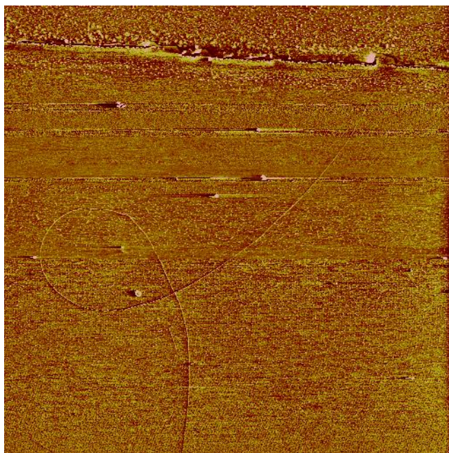
Figure A-5: An AFM phase scan of nanotube D6, the scan size is 25x25 μm.
