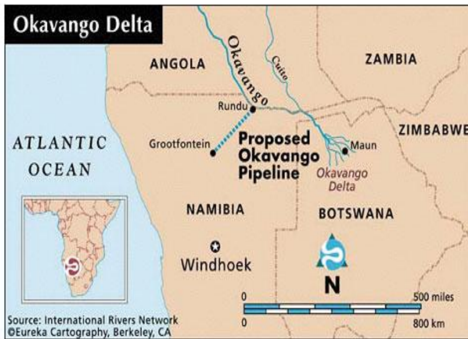
Figure 7. Proposed Rundo-Grootfontein Pipeline (represented by the broken line)—part of the ENWC IBT to divert water from the Okavango River Basin where it crosses into Namibia, and the current pipeline scheme. Map by Eureka Cartography, Berkeley, CA and is reproduced with permission (August 2008).
