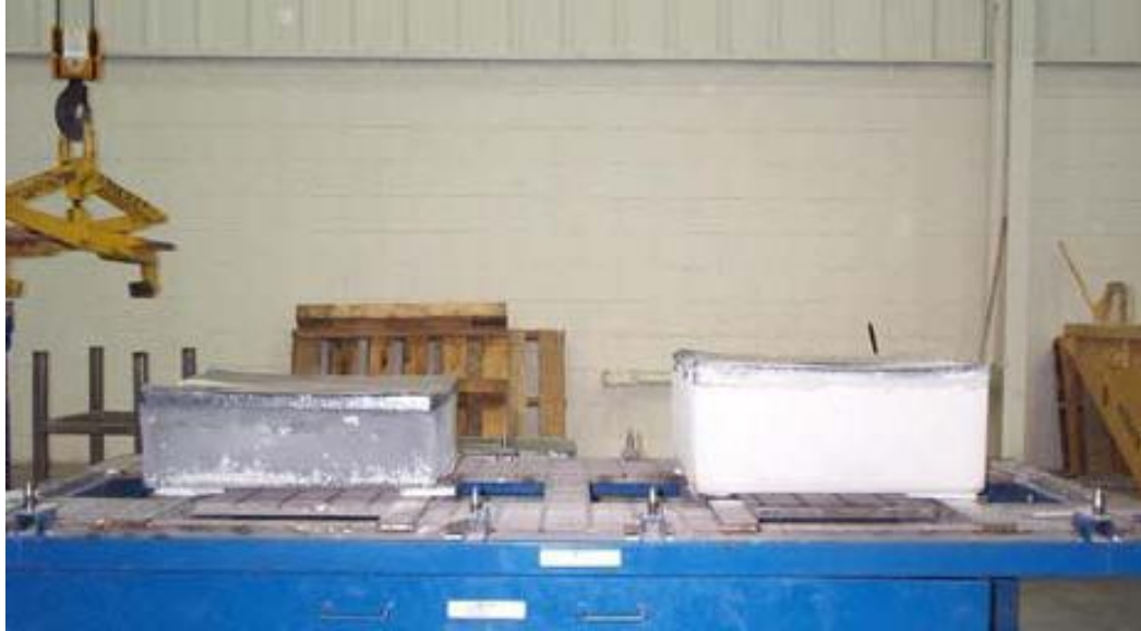
Figure 1: A typical MC Ingot [4] NREL
