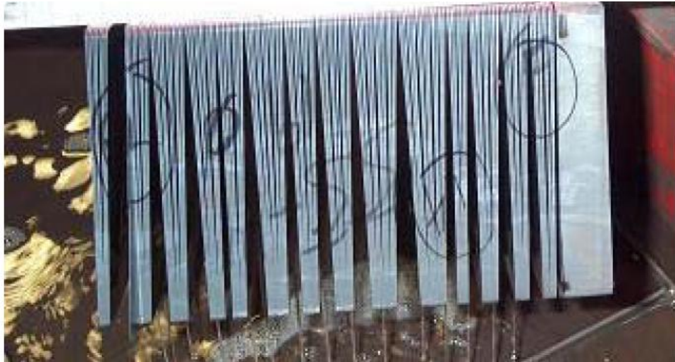
Figure 2: An Ingot after being wafered by a wire saw. [4] NREL
