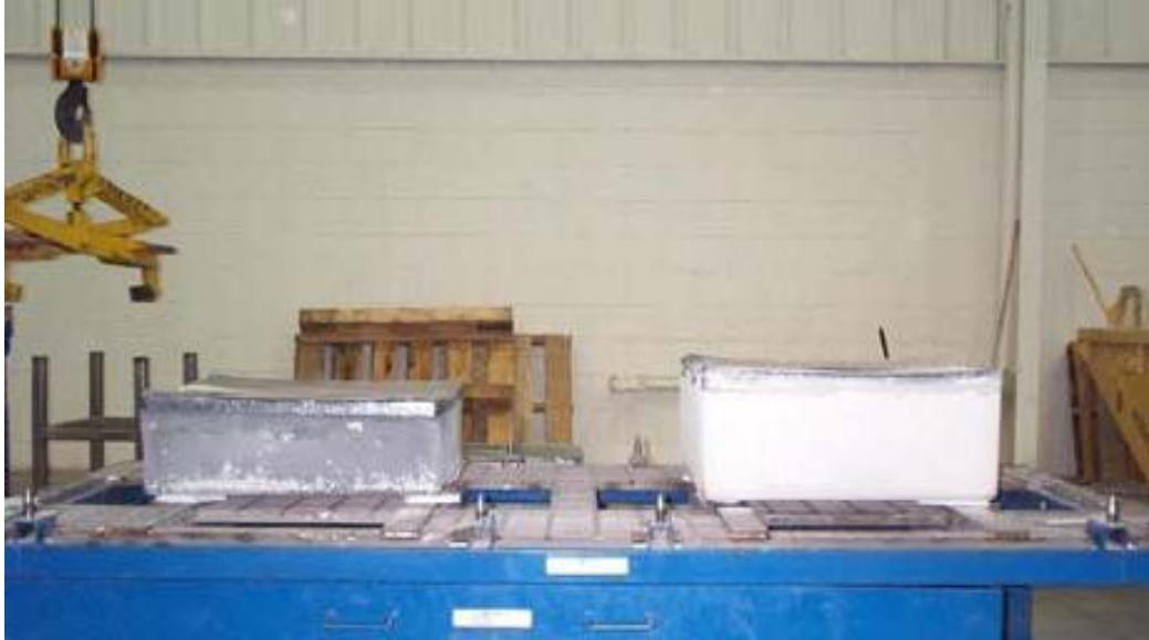
Figure 1: A typical MC Ingot [4] NREL
