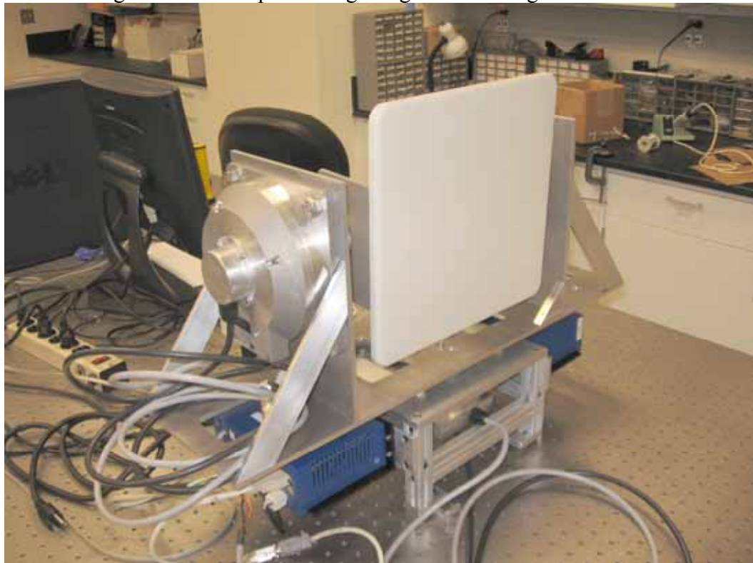
Figure 2.8: Finished RAD antenna gimbal
