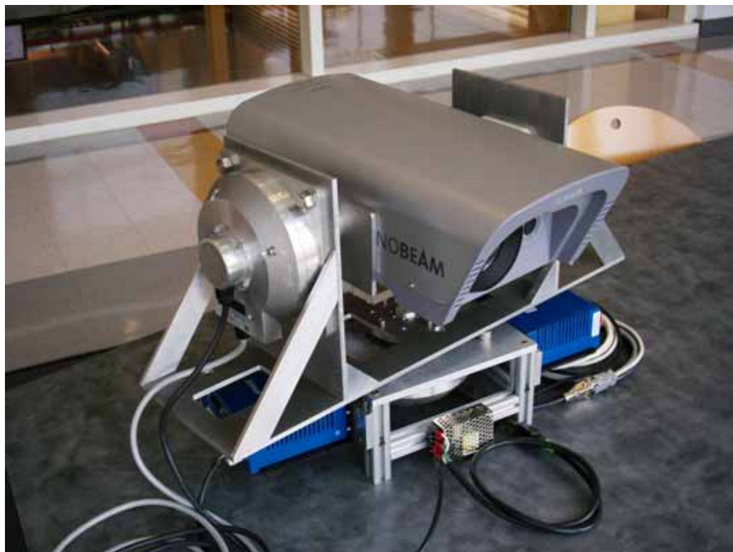
Figure 2.6: Finished Canobeam Gimbal
