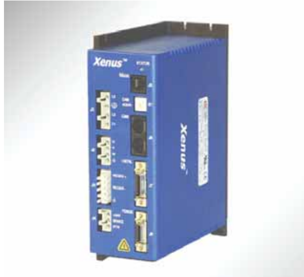
Figure 1.12: Copley Xenus Servo Drive [8]
