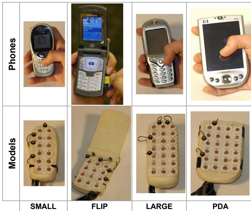
**Figure 9. Thumb Movement Study: Devices used for the thumb movement study, chosen to represent a range of sizes and forms (top row), together with their study-ready models (bottom row).**
