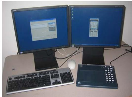
**Figure 31. The FaThumb study equipment setup. The study control software is displayed on the left screen, which was controlled by the Qwerty keypad, and the FaThumb interface is displayed on the right screen, and controlled by the Ergodex keypad.**
