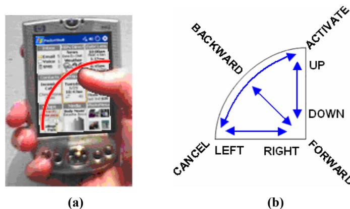
**Figure 24.** A depiction of the screen region that is accessible to the thumb of one hand (a), and the AppLens command gesture set (b).
