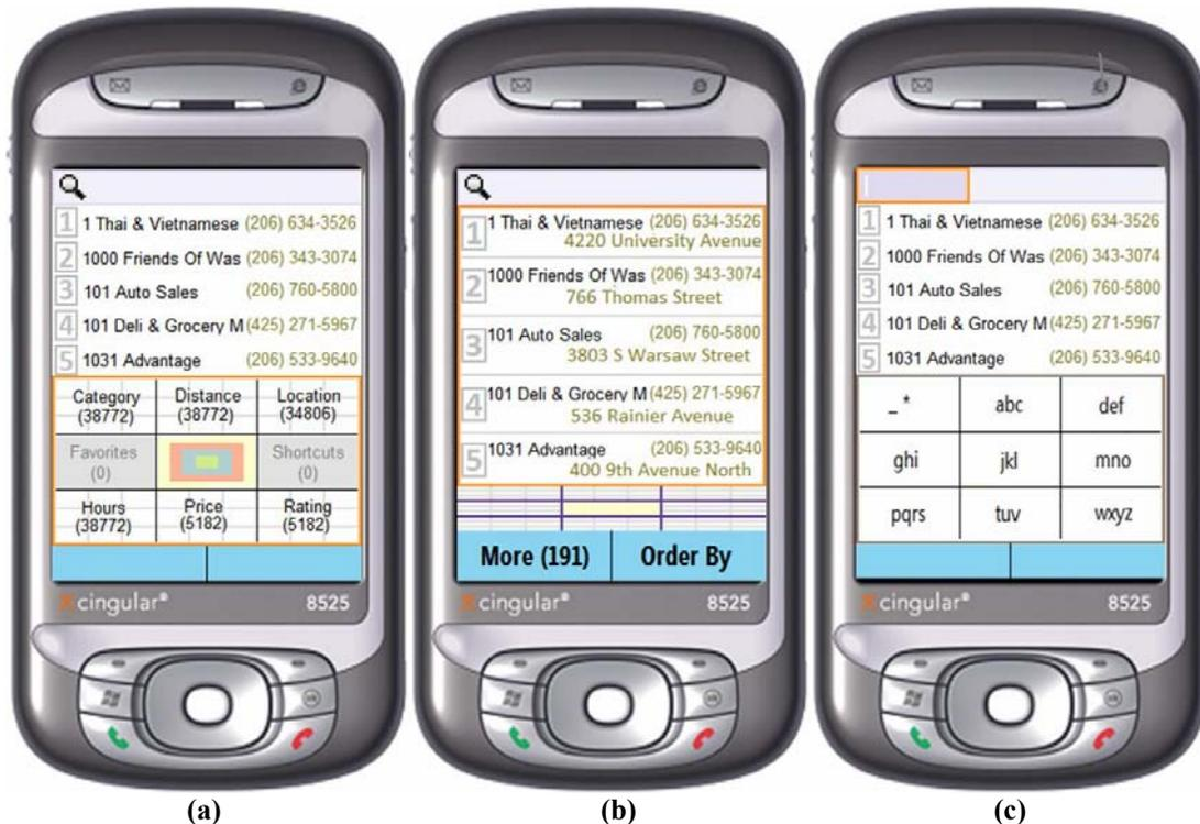
**Figure 30. Example screen designs for a thumb-based touchscreen version of FaThumb. The default layout, with the input focus on the Facet Navigation region (a) and the display of results when the input focus is on the Results region (b). When the input focus is on the Filter region, the Facet Navigation region updates to support text entry (c).**
