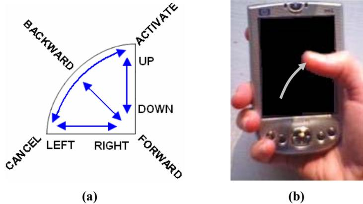
**Figure 20. Gesture Study: The indirect gesture command language for controlling the object selection cursor (a); and an example of issuing an ACTIVATE command (b).**
