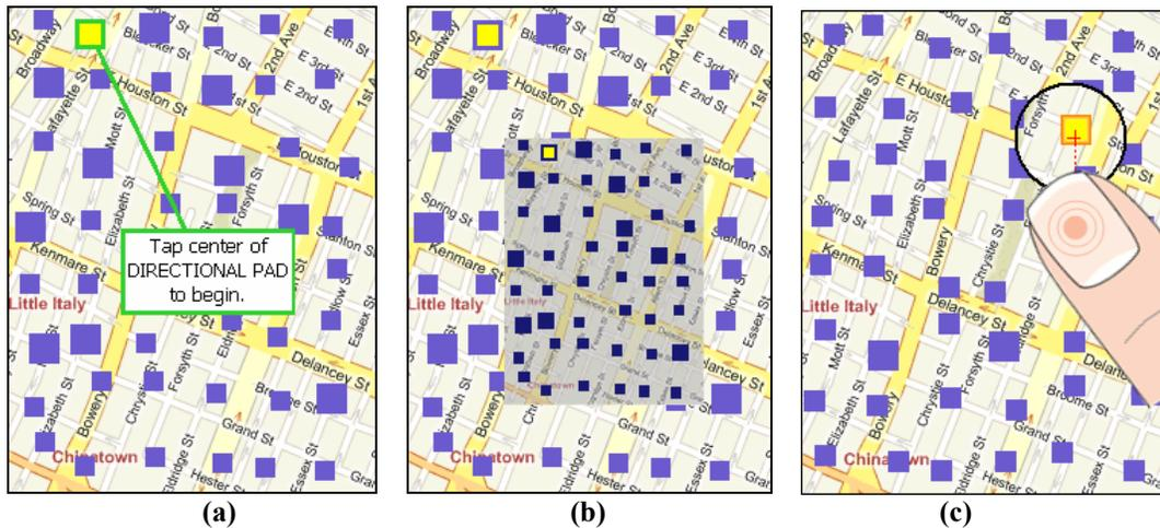
**Figure 39. ThumbSpace Study 1: Representative screen shots from the experiment. An example of a task instruction (a). Performing a task using ThumbSpace (b). Performing a task using Shift (c).**
