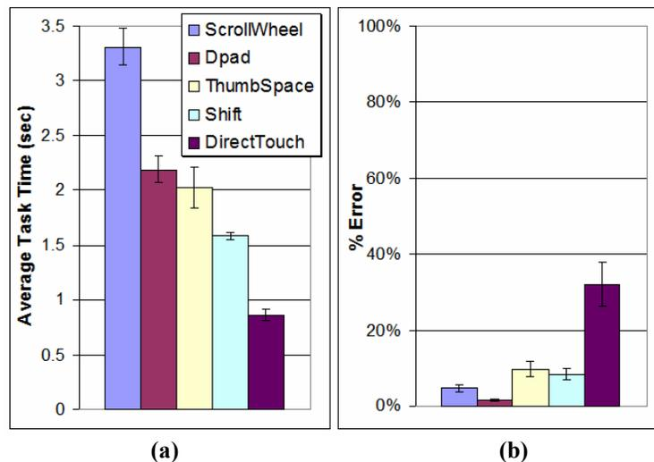
Figure 40. ThumbSpace Study 1: Average task times (a) and error rates (b) by input type.
