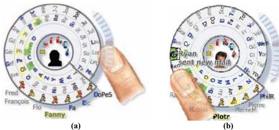
**Figure 4. SpiraList, a one-handed thumb-based design for viewing and navigating text-based lists on a touchscreen device. Browsing via an indirect list control widget (a), and direct item selection using an offset cursor (b).**
