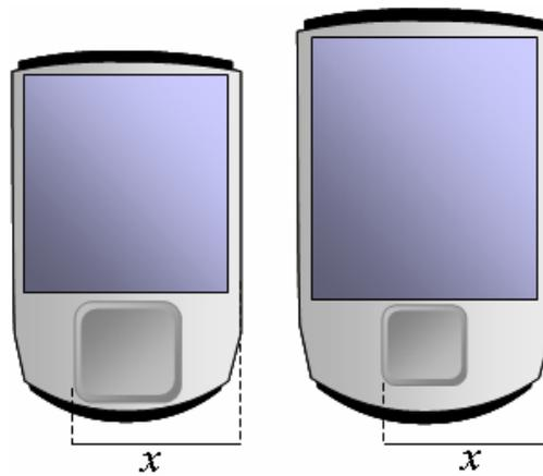
**Figure 51. A depiction of how the size of a touchpad might change to accommodate left and right handed use for two different screen sizes. Assuming a user’s maximum horizontal reach is of length  $x$ , touchpads will need to shrink as devices grow larger in order to accommodate one-handed operation.**
