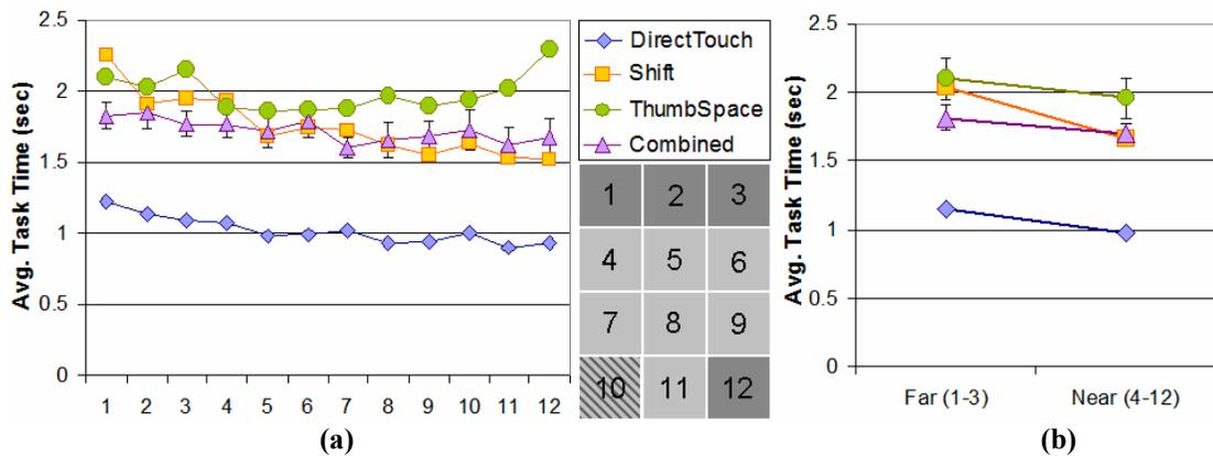
**Figure 45. ThumbSpace Study 2: Average task times by region for each input type. Average task times for all 12 regions (a). Average task times for the aggregate distances “far” and “near” (b).**
