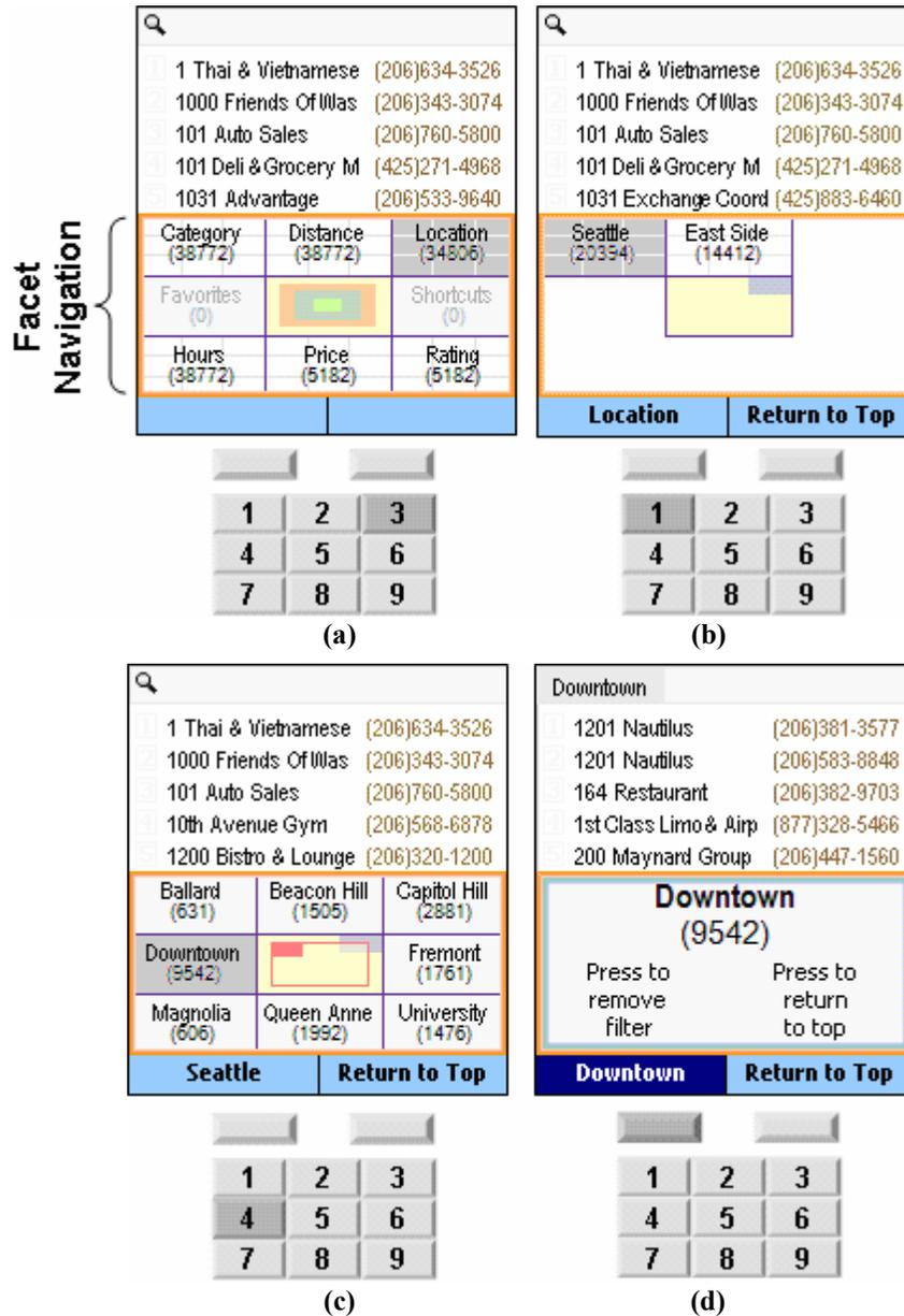
**Figure 28.** An example of facet navigation using FaThumb. From the root of the facet hierarchy, pressing 3 navigates to Location (a). At the next level, pressing 1 navigates to Seattle (b). Pressing 4 then navigates to Downtown (c), and finally pressing the left menu button adds Downtown to the query (d).
