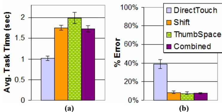
Figure 43. ThumbSpace Study 2: Average task times (a) and error rates (b) by input type.
