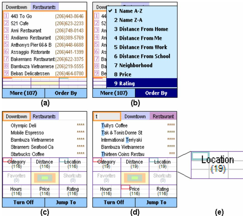
Figure 29. FaThumb results interaction sequence. When active, the results region expands to display up to 9 items (a). The right menu button opens the Order By menu (b); pressing 9 sorts results by Rating. The up arrow moves the activation region to the filter bar (c). Typing in a search term updates the results (d). A facet node in detail (e).
