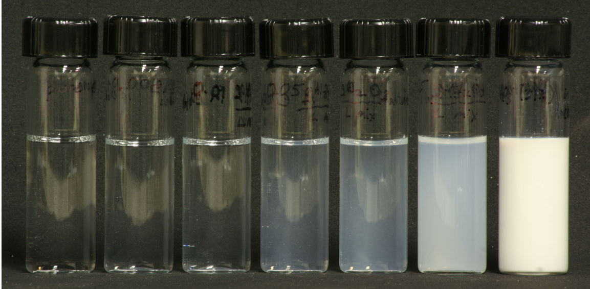
Fig. 15. Alumina-in-ethanol nanofluid samples (from left to right: 200 proof ethanol, 0.005 g/L, 0.01 g/L, 0.05 g/L, 0.1 g/L, 0.5 g/L, and 30.84 wt.%).
