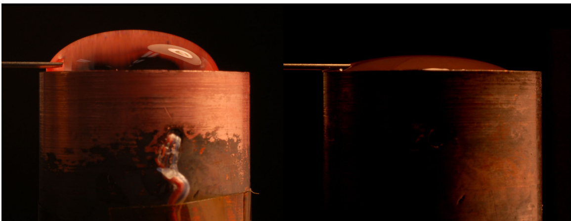
Fig. 42. Photographs of the advancing contact angle on polished copper (left) and copper oxide (right).
