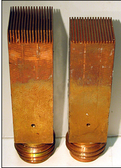
Fig. 23. Heater necks with 5 mm (left) and 1 mm (right) long fins.
