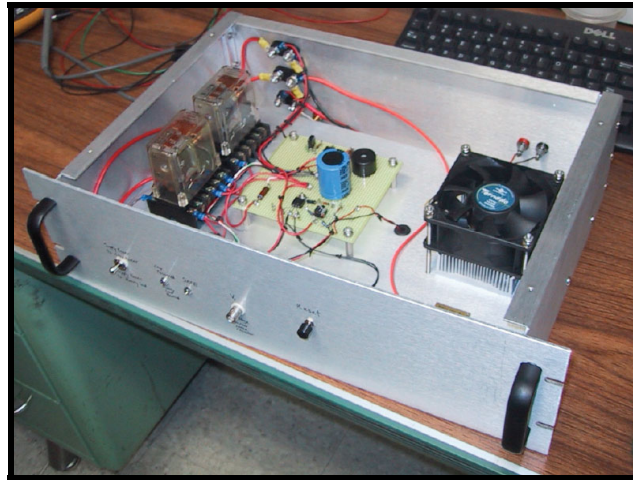
Fig. 10. Wheatstone bridge circuit to prevent burnout of the thick-film resistor.
