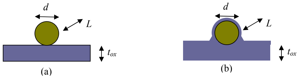
Fig. 6.12: (a) Nanowire geometry used for analytical capacitance expression, (b) Actual nanowire device geometry used for this study.
