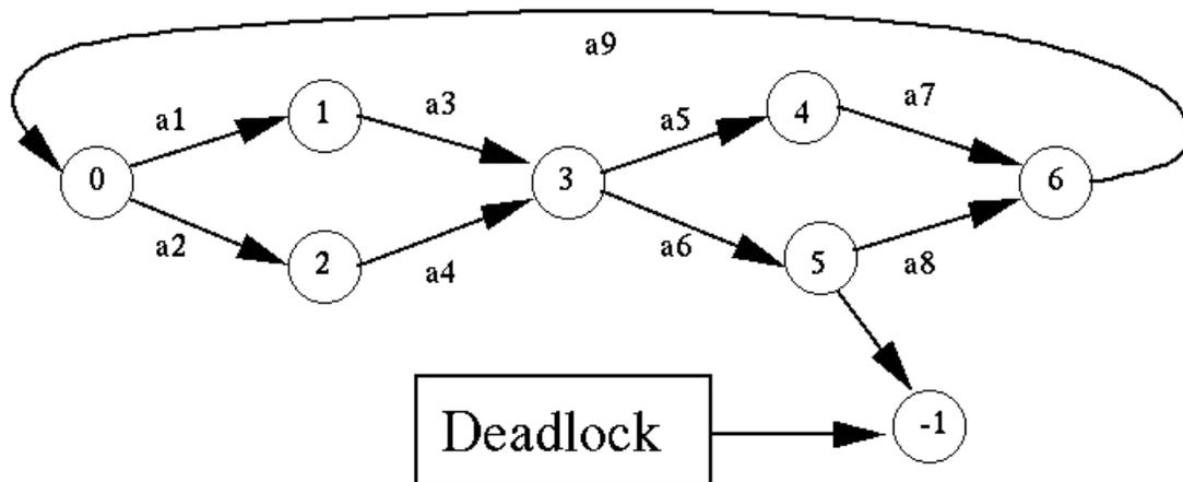
After eliminating all deadlocks within a system, the system can then be checked for progress errors, or errors in achieving desirable states. LTSA does not allow you to check for progress errors unless deadlocks are eliminated, since a deadlock is a type of progress error in itself. In the most basic terms, if a system has deadlocks, it doesn't function, but even if a system functions, it may not function properly, and that's where progress checking picks up the slack.
