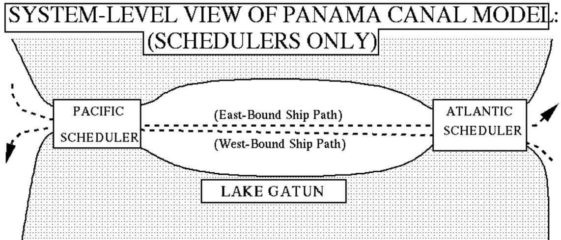
One could not simply tag two unique copies of the original lockset created. The double lock system with gates and pumps could be tagged, since the gates and pumps would still operate the same way, but the controllers and the schedulers needed to be copied and altered.
