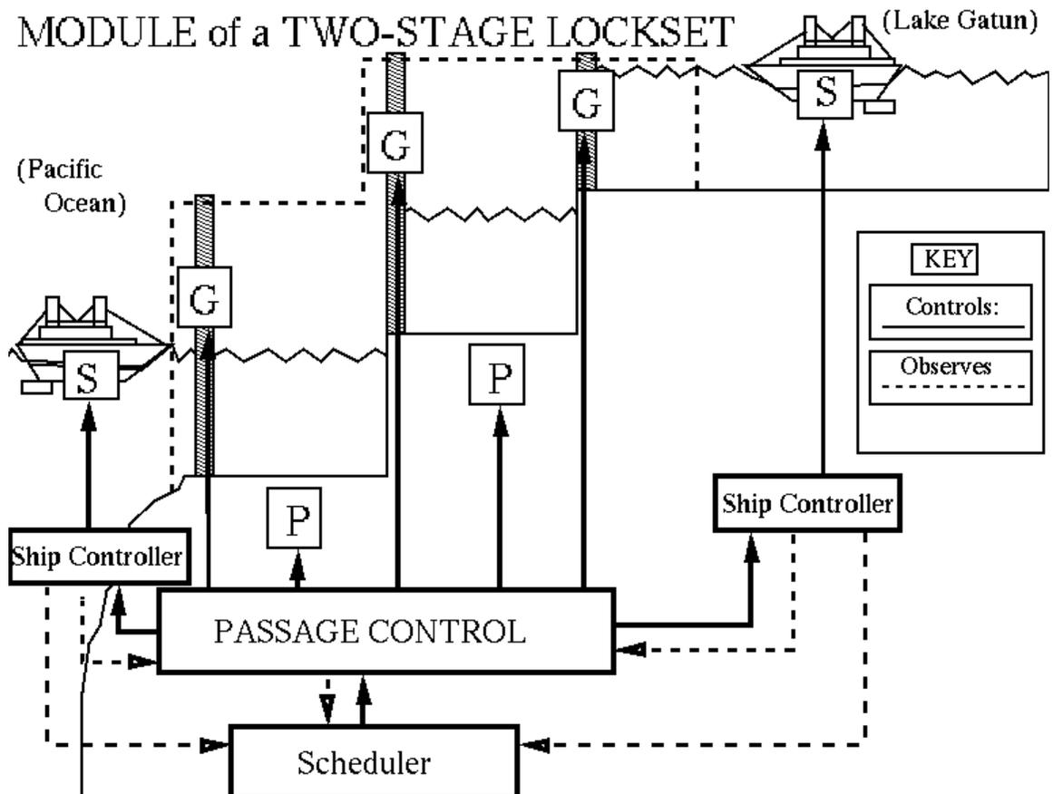
Controllers are used to make sure that each independent concurrent process works in synchronization with the others to perform the tasks of moving a ship up or down through the locks. The controller for each lock system was built with multiple starting conditions, on the basis that once one starting condition was met, a series of actions would be initiated to perform the EAST-WEST or WEST-EAST passing procedure.
