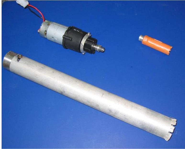
**Figure 4-10: Drill, Bit, and Core Tube**
