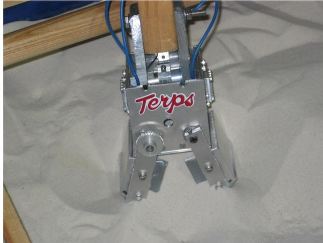
Figure 7-1: TERPS Collecting Pure Soil Sample
