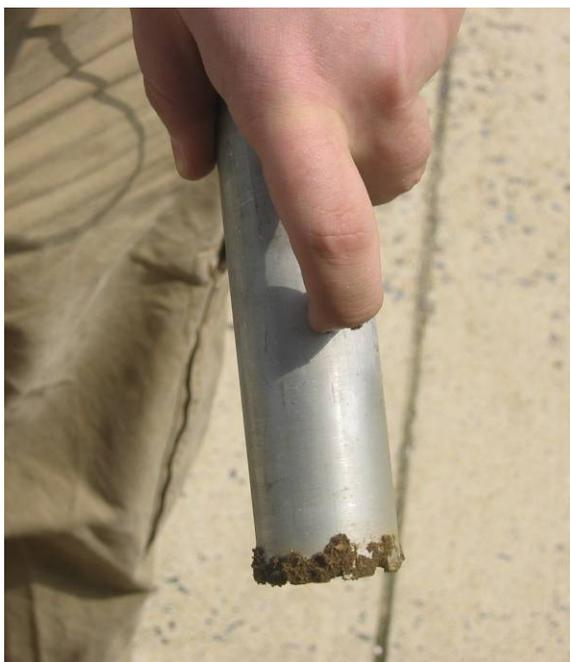
**Figure 7-6: 4 cm Soil Core**
