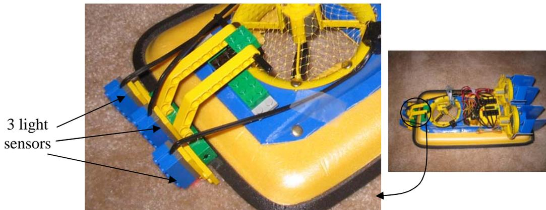
The light sensor on the left side is used to monitor the occurrence of deviations towards the left side during the motion. The light sensor on the right side is used to monitor the occurrence of deviations towards the right side during the motion. The light sensor located in the middle is used to monitor the deviation to either side.
