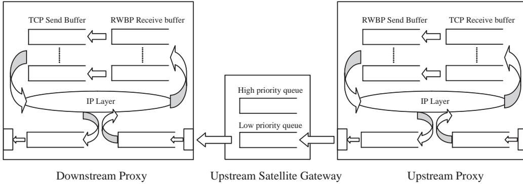
Fig. 2. Queuing model for the satellite gateway and proxies. Flow control is done between downstream proxy and upstream proxy, and between satellite gateway and upstream proxy. It is also done between link layer and the IP layer, between the IP layer and transport layer, and inside transport layer.
