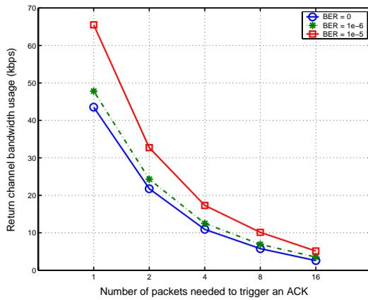
Fig. 4. Return channel usages for different acknowledgement frequency in RWBP
