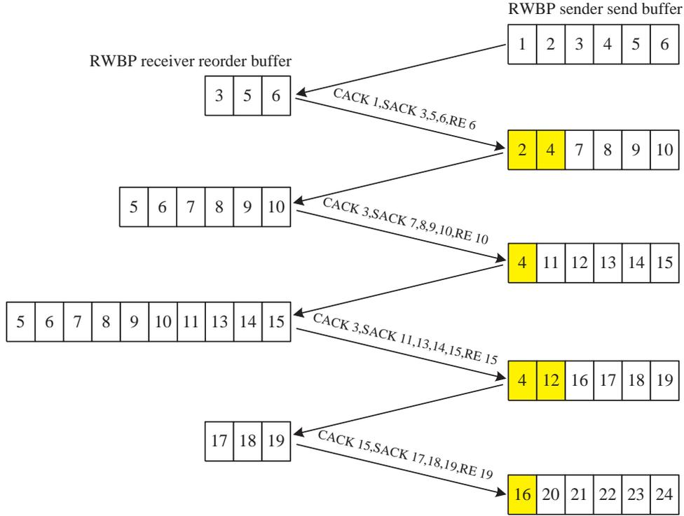
Fig. 3. Error control in RWBP. CACK : Cumulatively acknowledged; SACK : Selectively acknowledged; RE : Right edge
