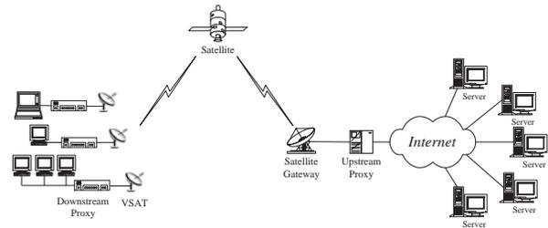
Fig. 1. Direct to user satellite networks (star topology)
