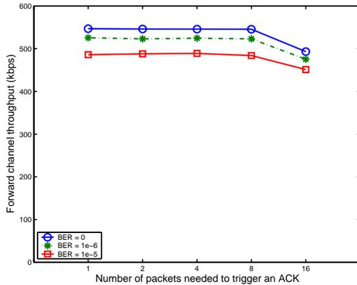
Fig. 5. Forward channel throughputs for different acknowledgement frequency in RWBP
