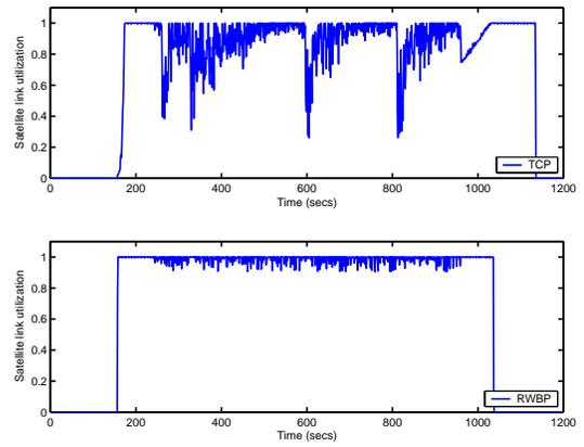
Fig. 11. Satellite link utilization for TCP and RWBP with high priority UDP traffic
