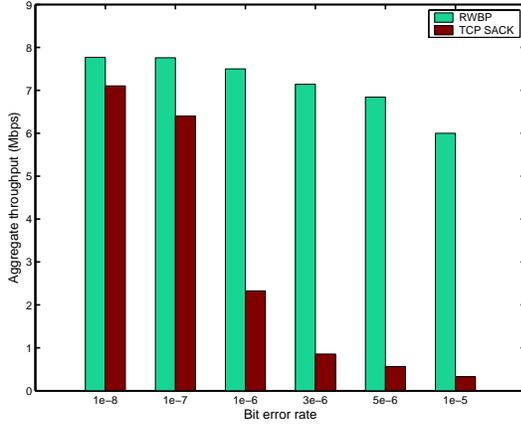
Fig. 7. Aggregate throughput for different bit error rates in RWBP and TCP
